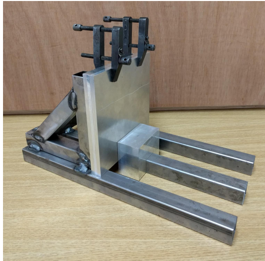
Fig. 4.9: An arrangement of three aluminium plates in rig from Fig. 4.8. Note use of Tool Maker's Clamps.
