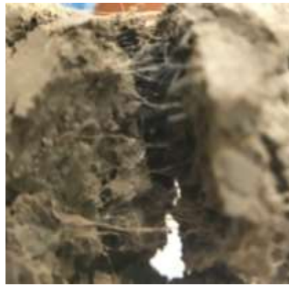
Figure 3.6 Even distribution of fibres in dry mixing.
