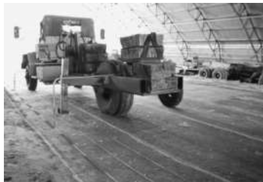
Figure 2.7. Traffic test with 13608-kg single-wheel assembly cart (from Santoni and Webster, 2001).
