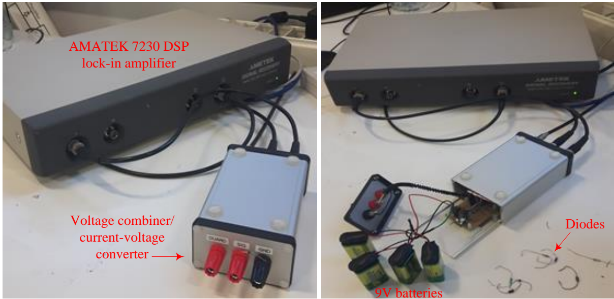
Figure 5.2: Pictorial representation of the actual setup used for the characterisation
