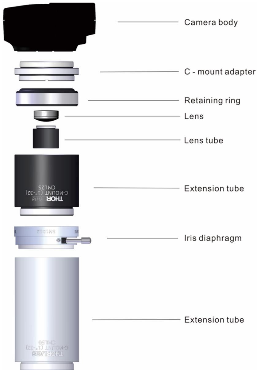
**Figure 6.3:** Visualisation of the camera and lens configuration initially used in the preliminary experiments.
