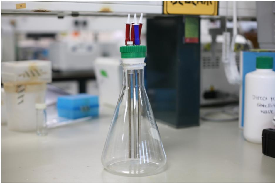
**Figure 6.2:** A standard wide-mouth 1 litre beaker fitted with the specialised bung supplied by Algeniuty for the Algem. The various nozzles can be configured to allow nutrient and gas supply to the culture.
