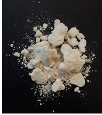
Figure 6.7: Precipitated calcium carbonate after being oven dried at 40 °C.
