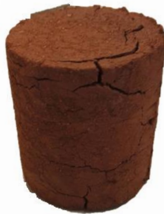
Figure 6.22: Formation of cracks after spraying the whole amount of cementing solution (equal to 80 % w_L ) on the sample surface in a single application.
