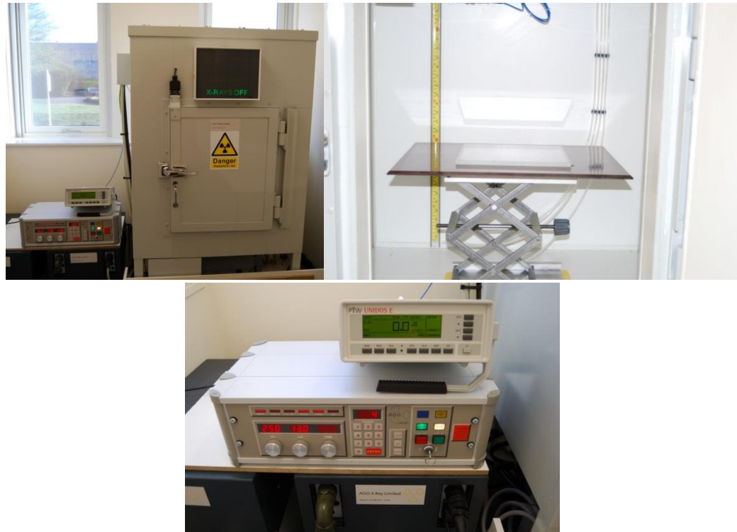
Figure 2.3: 250 kVp X-ray unit (CD160/1, AGO X-ray Ltd, Martock UK) located at PHE, Chilton (UK) where all x-irradiations were performed
