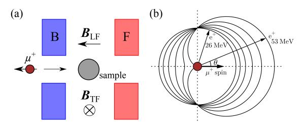
Figure 2.1: (a) A schematic of the experimental setup showing a muon entering the sample, situated between the forward detector F and the backward detector B. Also indicated are the directions of the applied magnetic field for the geometries. (b) The angular probability distribution  $W(\epsilon, \theta)$  for decay positrons emitted with kinetic energies between  $E_{\text{max}}/2$  and  $E_{\text{max}}$ .
