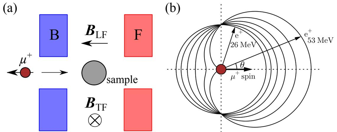
**Figure 2.1:** (a) A schematic of the experimental setup showing a muon entering the sample, situated between the forward detector F and the backward detector B. Also indicated are the directions of the applied magnetic field for the geometries. (b) The angular probability distribution  $W(\epsilon, \theta)$  for decay positrons emitted with kinetic energies between  $E_{\max}/2$  and  $E_{\max}$ .
