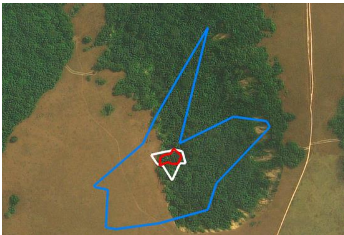
Figure 4.2 Local Convex Hull (95%, Neighbours: 30) of GPS collars in the stationary collar test. The blue polygon was created using the 3D points collected at 0.5 m, the white polygon was created using 3D points collected at 21 m and the red polygon was created using 3D points collected at 29 m.
