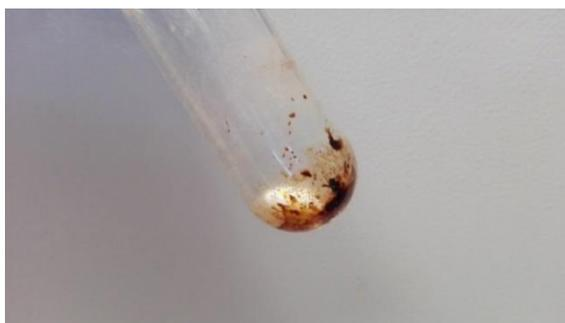
Figure 149: Polymeric tar produced by the reaction of KO<sup>t</sup>Bu with CF<sub>3</sub>CF<sub>2</sub>CF(CF<sub>3</sub>)(CH<sub>2</sub>CF<sub>2</sub>)<sub>2</sub>-7F
