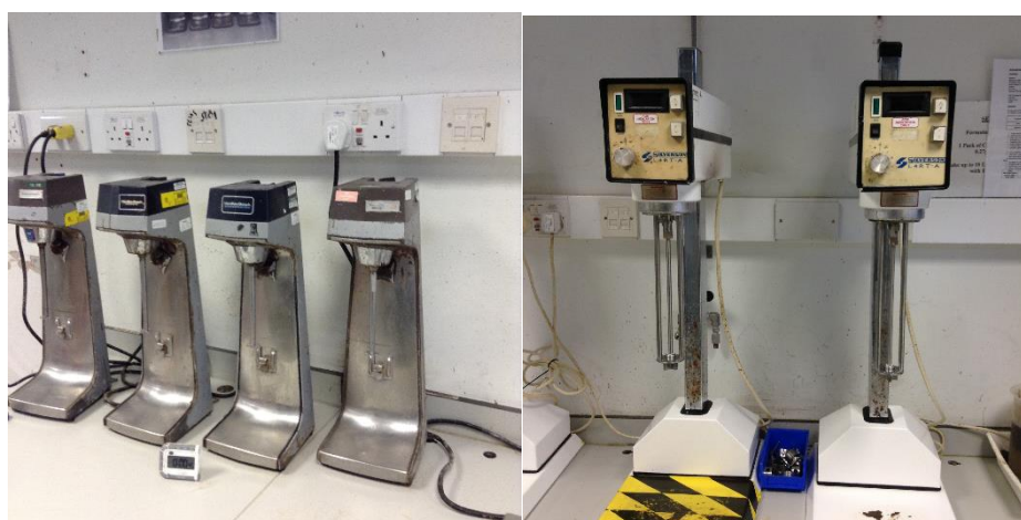
Figure 3.1 Mixer used for the formulation, with left hand image showing Hamilton Beach and right hand image showing the Silverson mixer.
