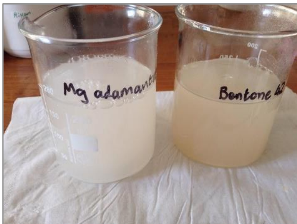
Figure 4.5 Comparison of samples with MgAl-Ada LDH after being ground + oil (left beaker), and Bentone 42 + oil (right beaker).
