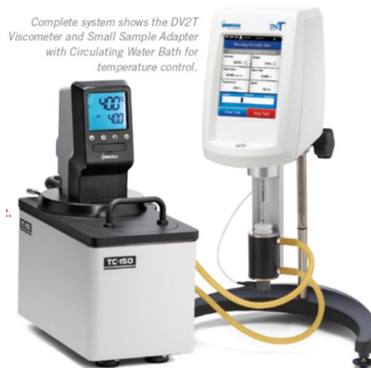
Figure 3.5 Brookfield DV2TRV with the circulating water bath. Modified from Brookfield 116
