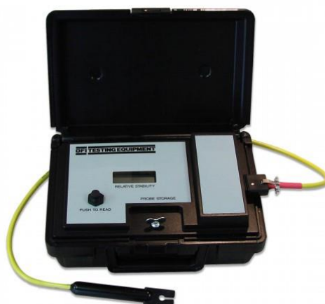
Figure 3.9 Electrical stability meter. Modified from OFITE 120 .
