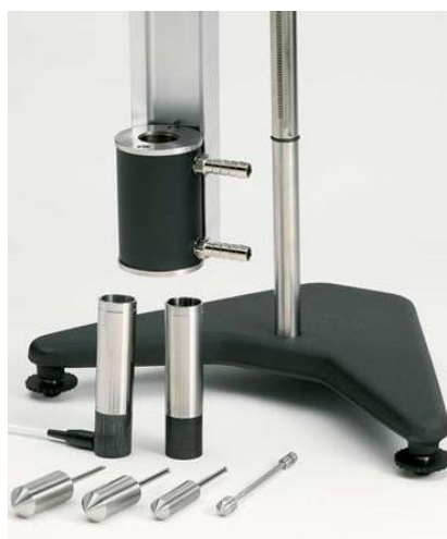
Figure 3.6 Small sample adapter kit. Modified from Brookfield 116
