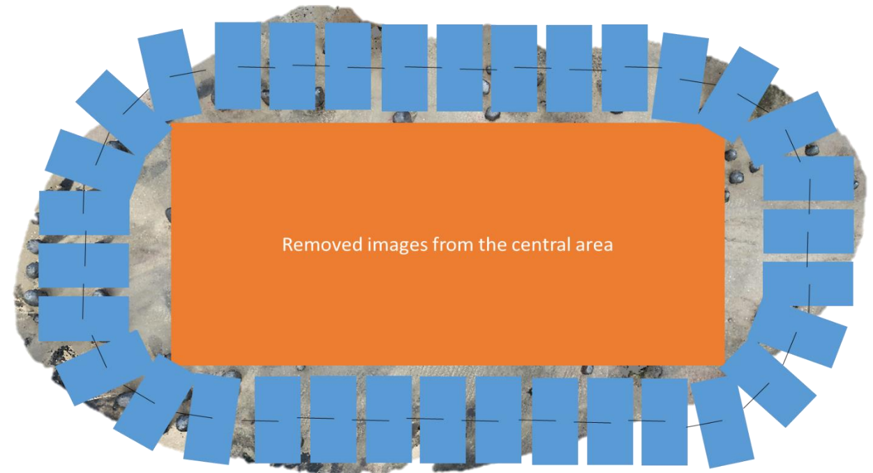
Figure 33: In order to get the aerial photographs to align with the terrestrial photographs, we removed the central block of images.
