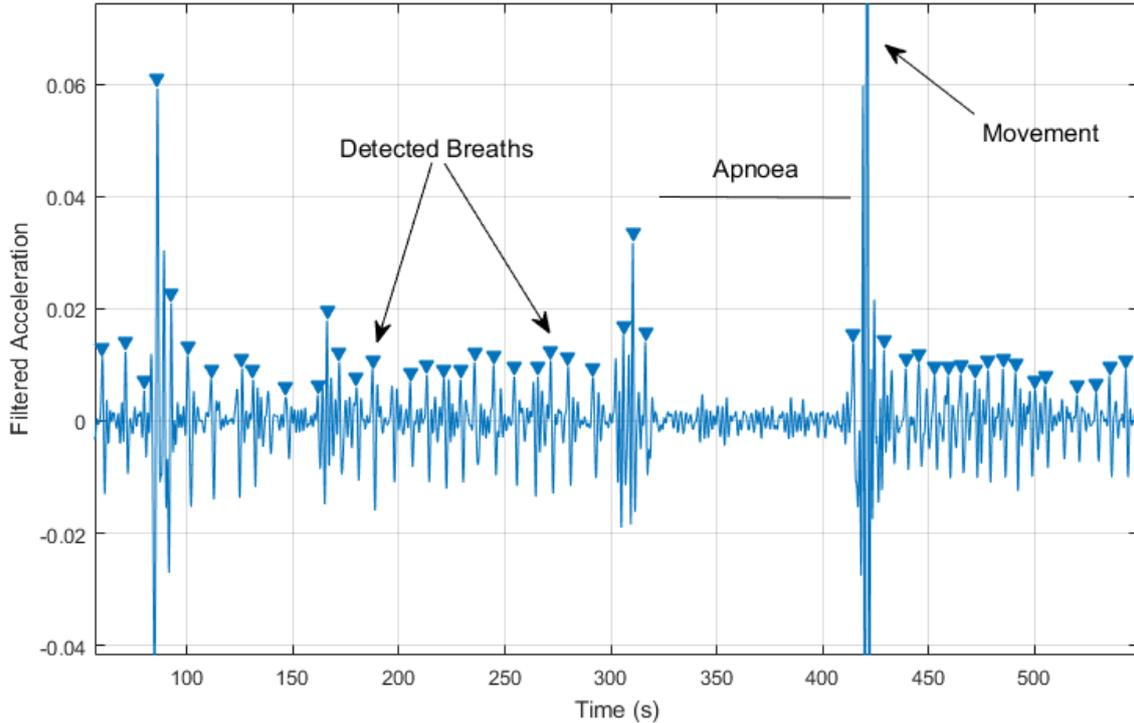
**Figure 6.3:** Example of breathing waveform as determined through accelerometers (g) indicating the peaks detected (blue triangles) through the detect peaks function in MATLAB. A period of apnea is also indicated by the lack of detected breaths. Each peak had a minimum peak prominence of 0.01 g and a 2.5 s blanking time (acceptable interval between peaks).
