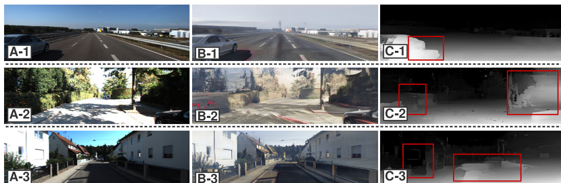
Figure 6.10: Examples of failures, due to light saturation and shadows. Issues are marked with red boxes.
