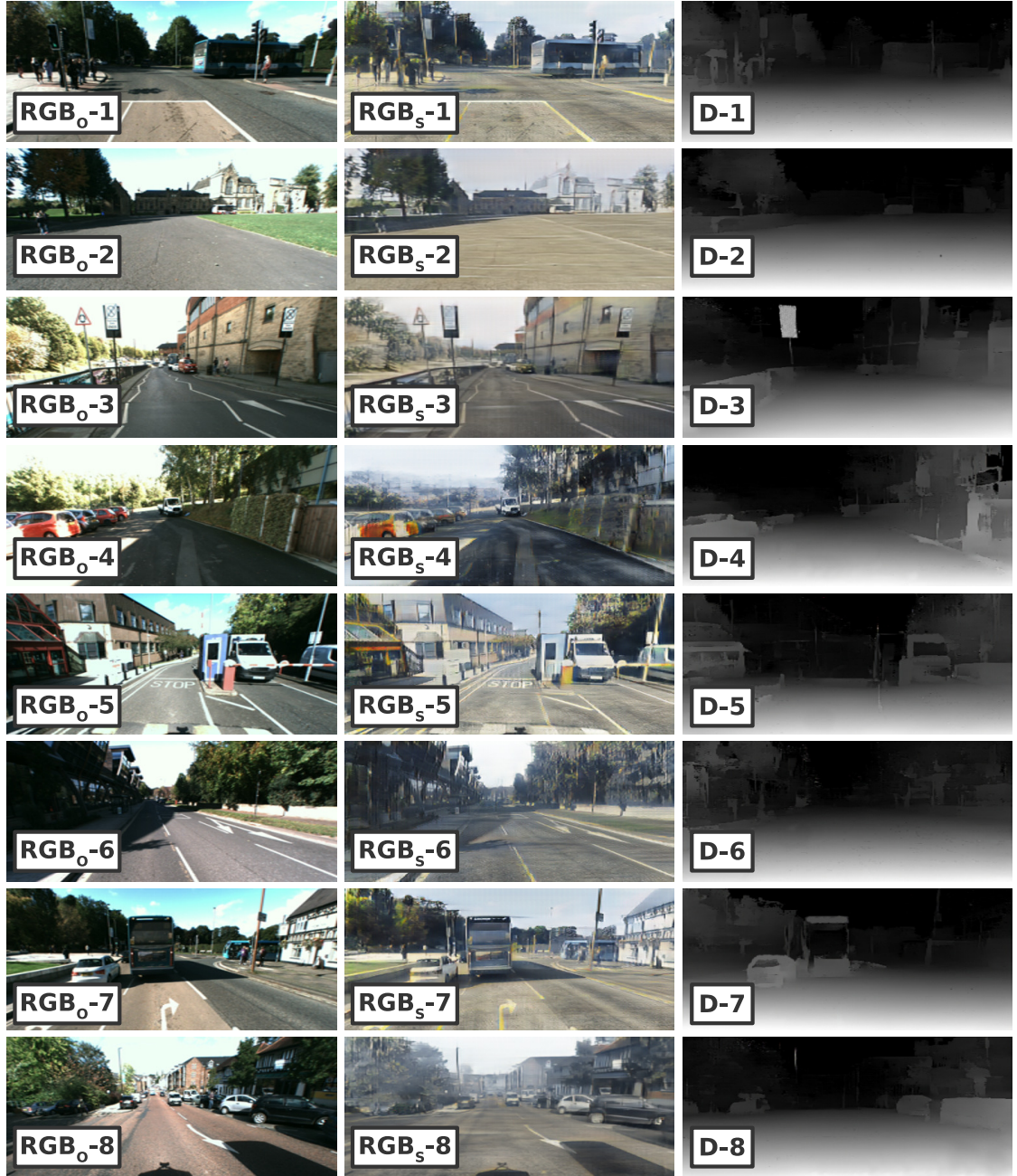
Figure 6.8: Qualitative results of our approach on urban driving scenes captured locally without further training. \mathbf{RGB}_O denotes the original real-world RGB images, \mathbf{RGB}_S represents the real-world images stylised into the synthetic domain and \mathbf{D} is the estimated depth.
