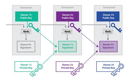
Figure 1. An illustrated version of Nakamoto's diagram of bitcoin transactions, 2008. Each transaction 'output' is linked to a previous transaction 'input' by the owner(0) signing the transaction data as well as the public key of the new owner(1) associated with a specific address and timestamping it.<sup>36</sup>
