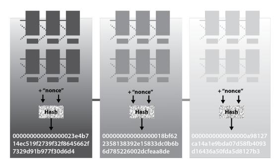
Figure 2. Transactions are grouped into blocks that are hashed with a 'nonce'. The hash output has to meet the requirement of the difficulty target, namely that it begins with a certain number of zeroes.
