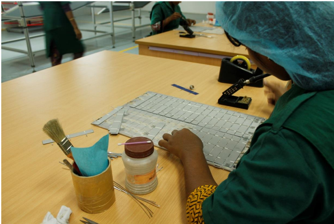
Figure 9:1 Assembling a solar panel
