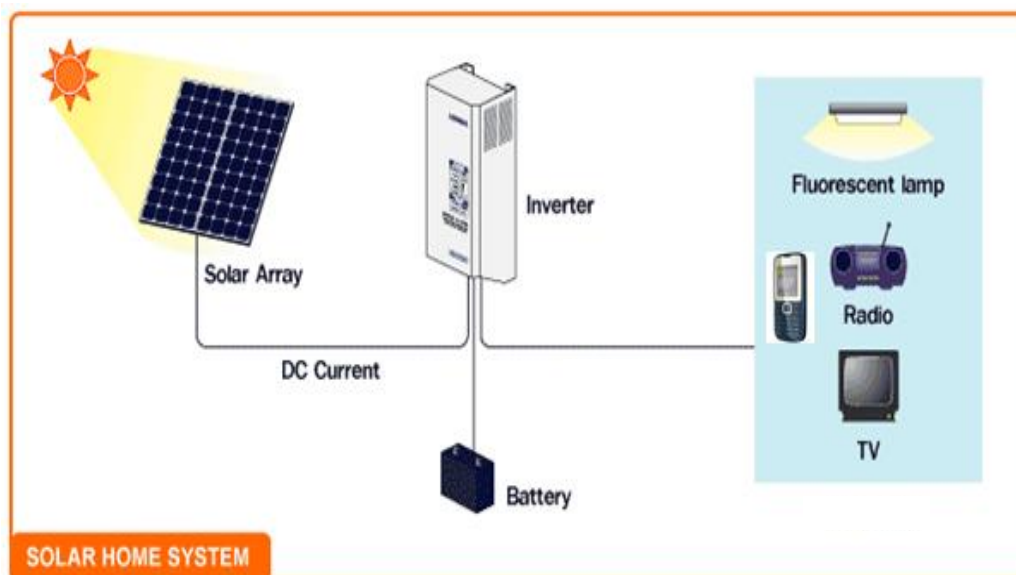
Figure 6:8 Components of a typical solar home system: Source: Author
