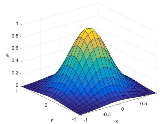
(d) Gaussian with  $\epsilon = 3$ .Figure 3.4: Three commonly-used RBFs at  $\{x\} = \{0, 0\}^T$  over a two-dimensional domain.
