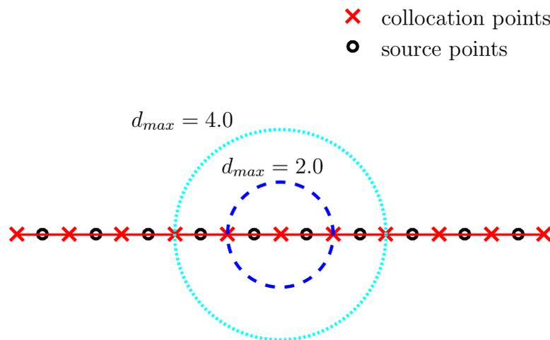
Figure 3.8: A portion of the one-dimensional bar with points distribution and different sizes of support domain.
