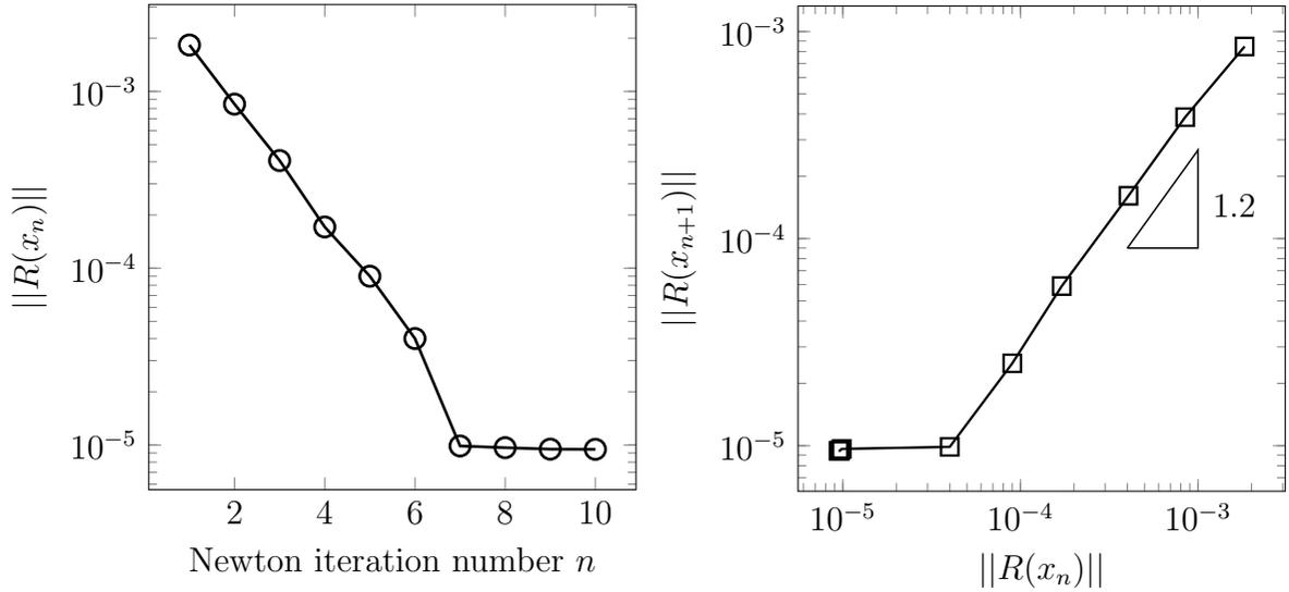
(a)  $\|R(x)\|$  versus Newton iteration number.(b) Convergence rate of  $\|R(x)\|$ .
