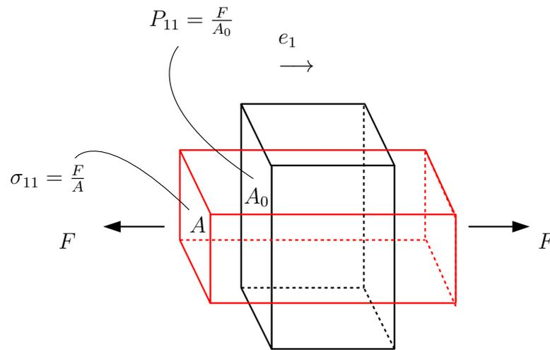
Figure 5.2: Stress components referred to the reference and current configurations.
