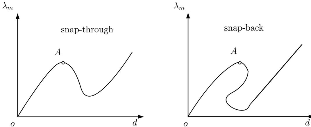
Figure 6.4: Unstable equilibrium: Snap-through and snap-back behaviour.
