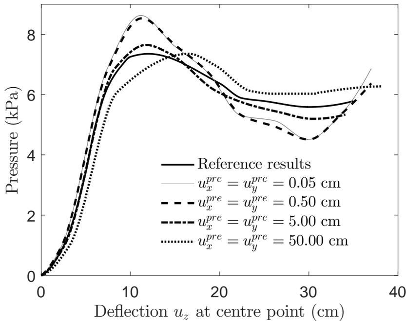
Figure 6.12: Pressure versus deflection at central point of the square hyperelastic membrane subjected to a uniform pressure.
