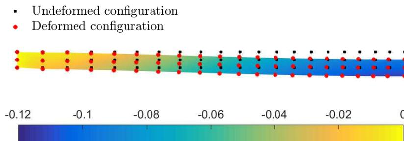
Figure 5.19: The reference and current configurations with displacement  $u_y$  of the plate with uniformly distributed load,  $q$ , and fixed at two ends.
