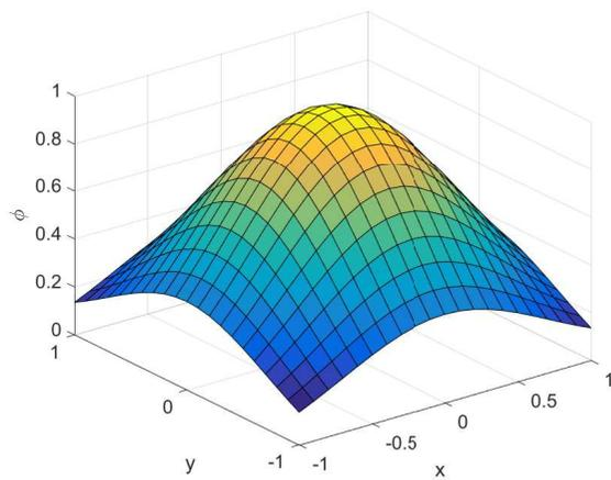
(c) Gaussian with  $\epsilon = 1$ .
