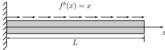
Figure 3.7: The geometry model of the one-dimensional bar.
