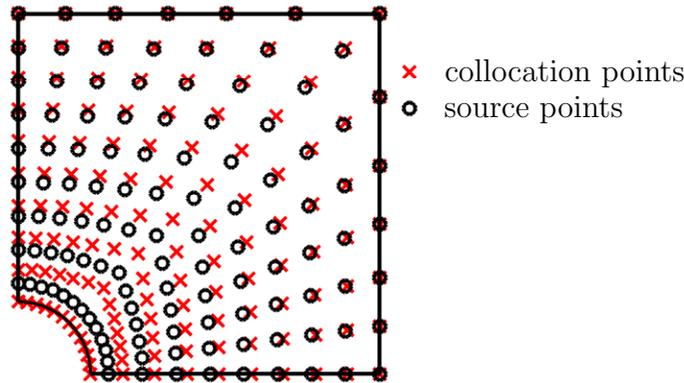
Figure 3.23: The discretisation of points of the infinite plate with a circular hole.
