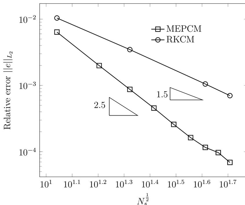
Figure 3.17: Convergence rate of  $\|e\|_{L_2}$  of the two-dimensional Poisson problem using the MEPCM and the RKCM.
