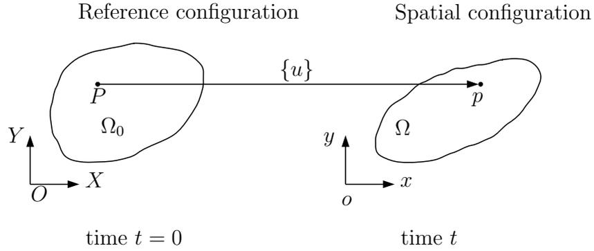
Figure 5.1: Configuration and motion of a continuum body.
