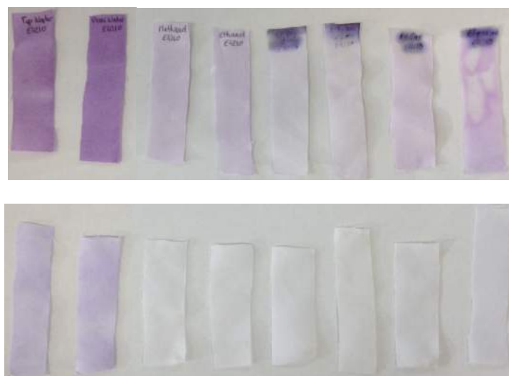
Figure 4.23: Influence of the solvent on the dye deposition onto polycotton with E4210 on the top and V200 on the bottom. Solvent used from the left to the right: Tap-water, Demi-water, Methanol, Ethanol, 1,2-propane diol (Pdiol), Ethylene Glycol, PdGW (58 % Pdiol, 17 % Glycerine, 25 % Water) and Glycerine.
