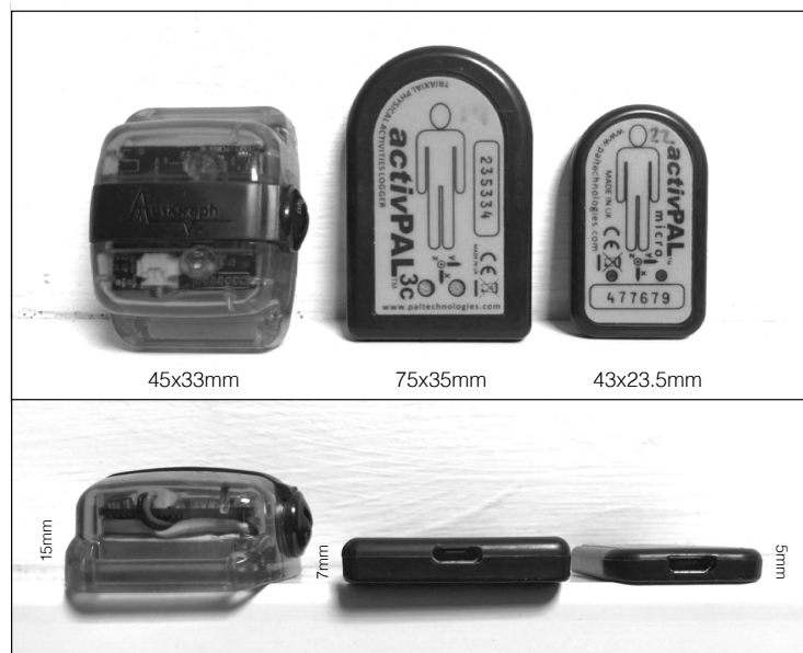
Figure 3.1. Side-by-side comparison of the dimensions of the ActiGraph GT3X (left), activPAL 3 (middle), and activPAL micro (right).
