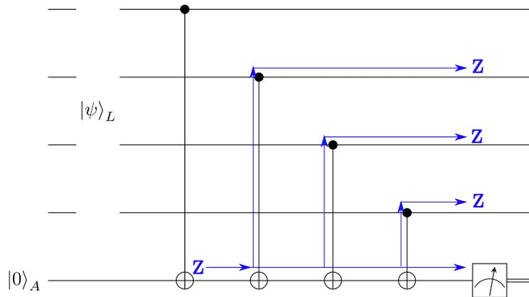
Figure 3.4: The extraction circuit for the  $Z_1Z_2Z_3Z_4$  stabilizer in the  $[[4, 2, 2]]$  code. Errors that occur on the ancilla qubit  $A$  can propagate to the code qubits. As an example, the propagation resulting from a  $Z$ -error that occurs after the first CNOT gate on the ancilla qubit is shown by the blue arrows.
