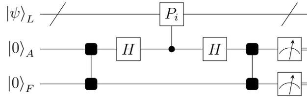
Figure 9.1: The flag method for syndrome extraction. A stabilizer operator  $P_i$  is applied to the register  $|\psi\rangle_L$ , and the result copied to an ancilla qubit  $A$ . Phase-flip errors on the ancilla are detected via two conjugate propagator gates that connect to a flag qubit  $F$ . The flag-check scheme is similar to the symmetric CPC gadgets we have covered in this thesis.
