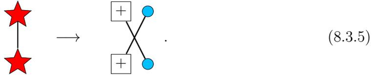
The phase-component of each qubit is connected to the bit-component of the other. This reflects the expected error propagation behaviour for cross-check edges.
