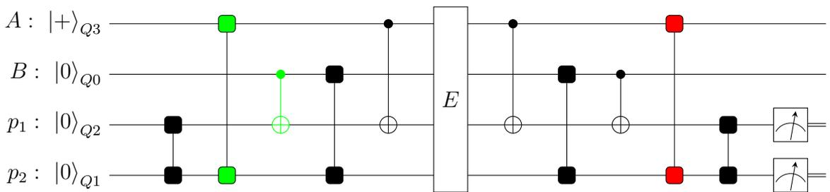
(b) A modified version of the  $[[4,2,2]]$  circuit in which the order of gates in the encoder and decoder has been rearranged. In this new form, the circuit can be simplified by noting that the action of the gates marked in green is the identity.
