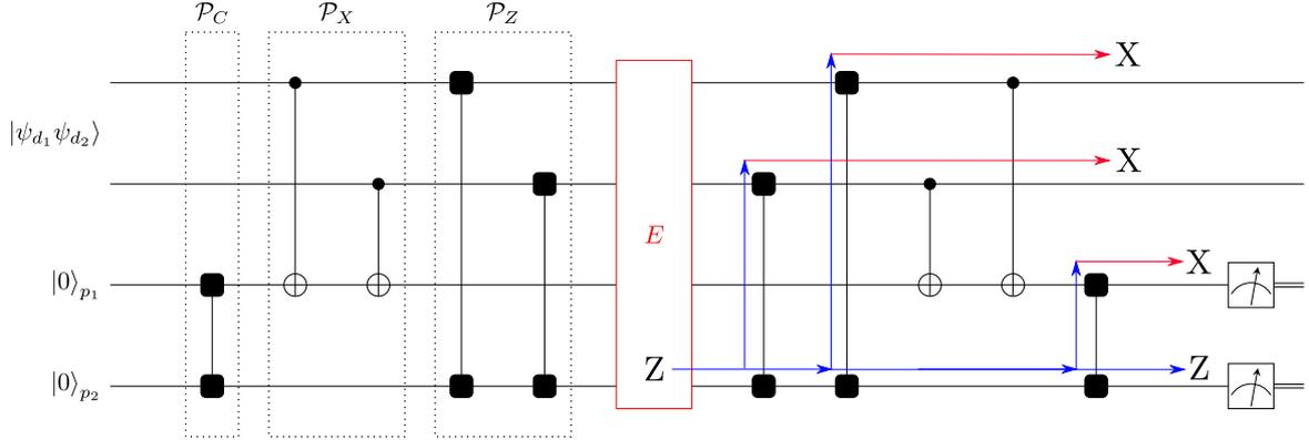
Figure 4.6: The  $[[4, 2, 2]]$  CPC code obtained by adding an additional cross-check stage  $\mathcal{P}_C$  to the encoder and decoder. The arrows show how the previously considered  $Z_{p_2}$ -error is now detected by the cross-check operator in  $\mathcal{P}_C$ . The  $Z_{p_2}$ -error is copied as a  $X_{p_1}$ -error to parity qubit  $p_1$  by the conjugate-propagator gate in  $\mathcal{P}_C$ . This  $X_{p_1}$ -error then triggers a ‘1’ syndrome in the  $M_{p_1}$  measurement.
