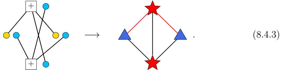
Once the classical code has the desired properties, it can be mapped back to the operational representation as shown to the right of the equation above. For this specific example, the two edges that were added to the classical factor graph map to a cross-check between the two parity qubits in the operational representation. The circuit this operational representation corresponds to is given by
