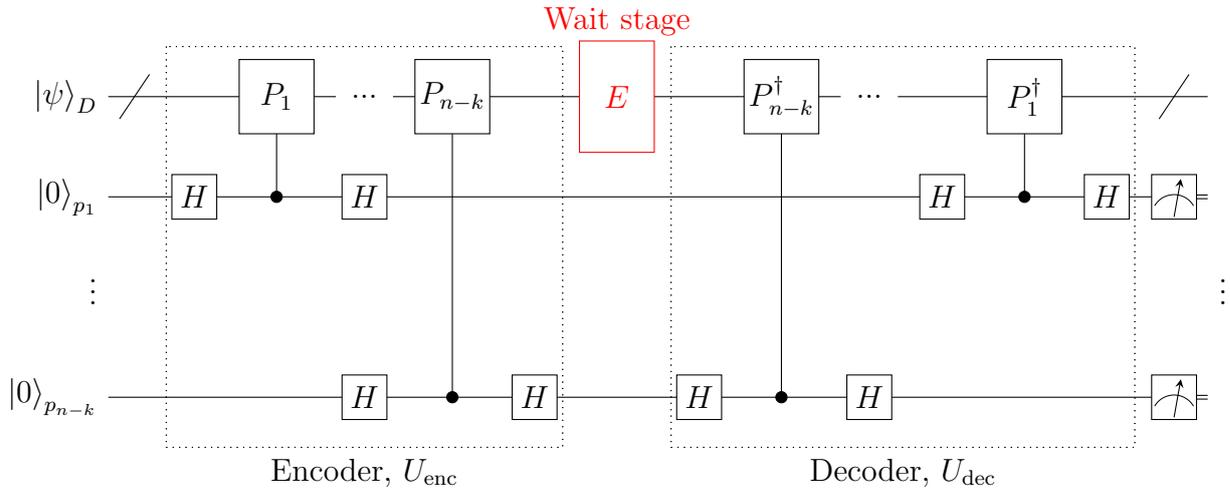
Figure 4.3: A CPC gadget which applies multiple parity checks  $\mathcal{P} = \{P_1, \dots, P_k\}$  to the register in a single cycle. A multi-check CPC code of this form retains the *encode-error-decode* structure, ensuring that any sequence of parity checks  $\mathcal{P}$  can be used without risk of decohering the register.
