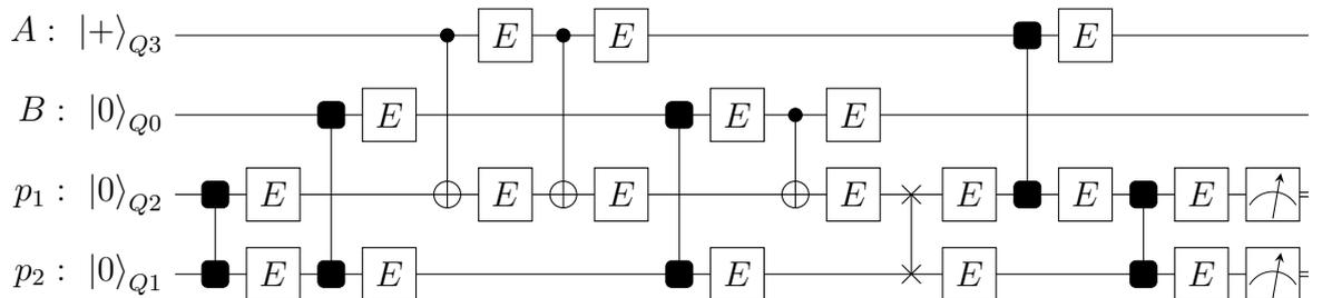
(d) When running the  $[[4,2,2]]$  code on a real device, it can no longer be assumed that errors occur only in the wait-stage between the encoder and decoder. For the  $[[4,2,2]]$  circuit in question, a single-qubit fault  $E$  after any gate will not propagate a multi-qubit error to the register without triggering a syndrome.
