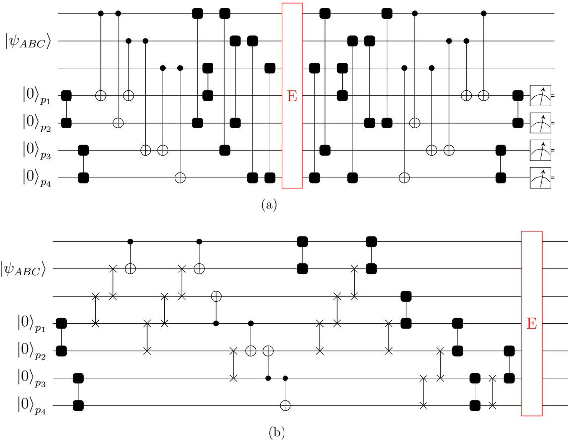
Figure 7.4: Circuit diagrams demonstrating SWAP gate compilation for a nearest-neighbour architecture. (a) The  $[[7, 3, 3]]$  code with the smallest two-qubit gate count prior to the addition of SWAP gates. (b) The encoder for the same circuit, with SWAP gates included. *This figure was originally published in [2].*
