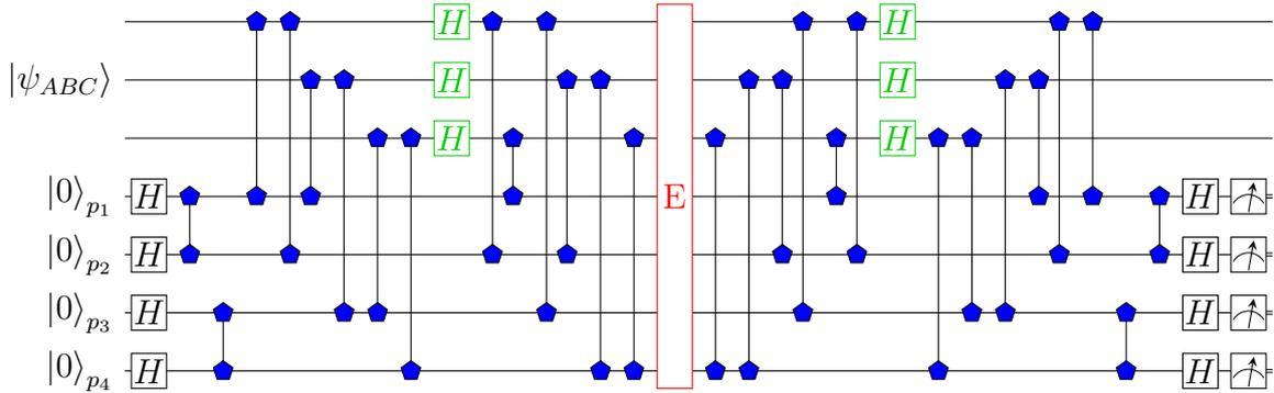
Figure 7.5: The native gate compiled form of the  $[[7, 3, 3]]$  CPC code with the lowest total gate count. Note that the SWAP operations have been omitted to save space. *This figure was originally published in [2].*
