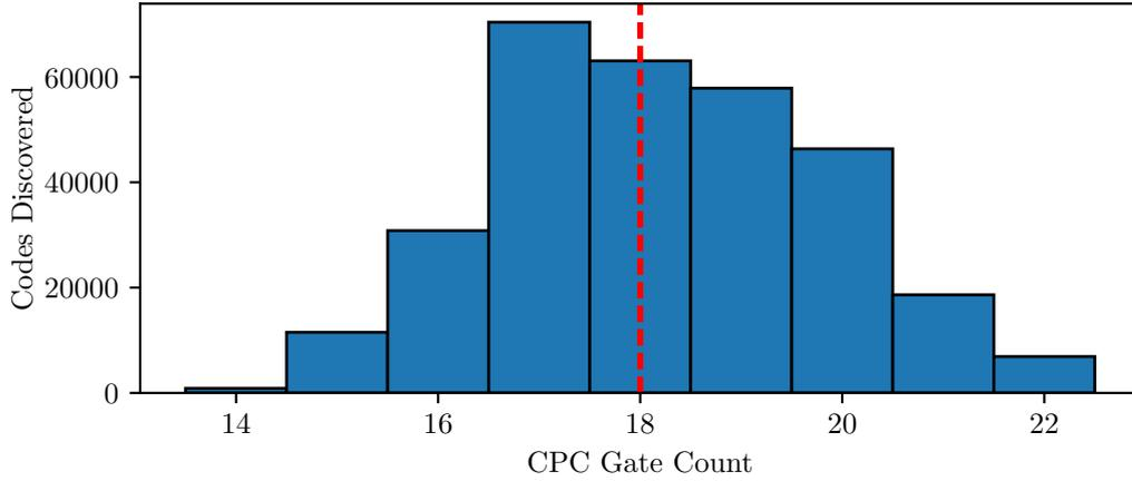
Figure 7.1: A histogram showing all of the  $[[7, 3, 3]]$  CPC codes discovered in stage 1 of the CPC design process, binned by encoder length. The CPC gate count is the combined total of CNOT and conjugate propagator gates in the encoder. The median length, marked in red, is 18. In comparison, the shortest  $[[7, 3, 3]]$  circuits have a CPC gate count of 14. *This figure was originally published in [2].*
