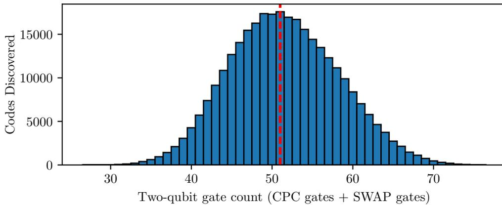
Figure 7.3: The distribution of  $[[7, 3, 3]]$  CPC codes binned by two-qubit gate count after compilation onto a nearest-neighbour architecture. The total gate count is defined as the number of CPC gates + SWAP gates in the encode stage of the circuit. *This figure was originally published in [2].*
