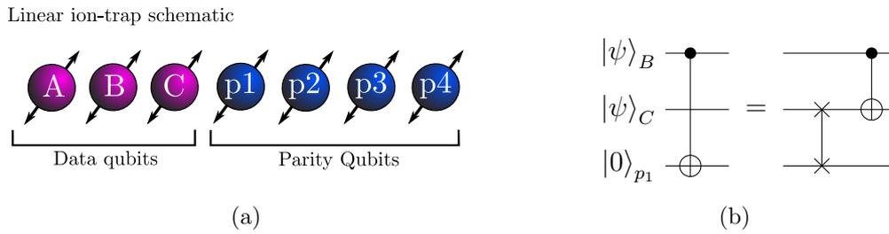
Figure 7.2: (a) A schematic of the seven-qubit linear ion trap. Three of the qubits have been labelled as data qubits and four as parity qubits as required by the  $[[7, 3, 3]]$  code. It is assumed that entangling gates can only be performed between nearest-neighbour qubits. (b) A CNOT gate between spatially separated qubits can be implemented using only nearest-neighbour interactions through the addition of SWAP gates. *This figure was originally published in [2].*
