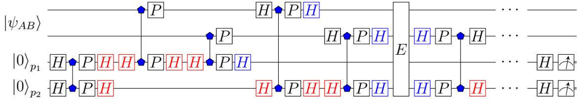
(b) The compiled circuit prior to simplification. Note that parts of the decoder have been hidden to save space. The pairs of Hadamards, labelled red, cancel to the identity. The blue  $H$  gates can also be discarded without affecting the operation of the code.
