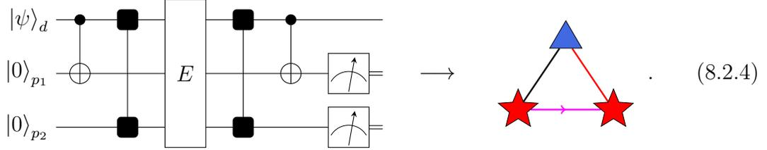
A  $Z$ -error in the wait-stage on qubit  $p_2$  will propagate to the register via the conjugate propagator gate, before being propagated to qubit  $p_2$  by the CNOT gate. The  $Z$ -error on qubit  $p_2$  is therefore detected by parity measurement  $p_1$  via an indirect pathway. This is illustrated by the pink virtual edge between the two parity qubits. In general, the adjacency matrix  $m_v$  for virtual propagation in a CPC circuit can be calculated as follows
