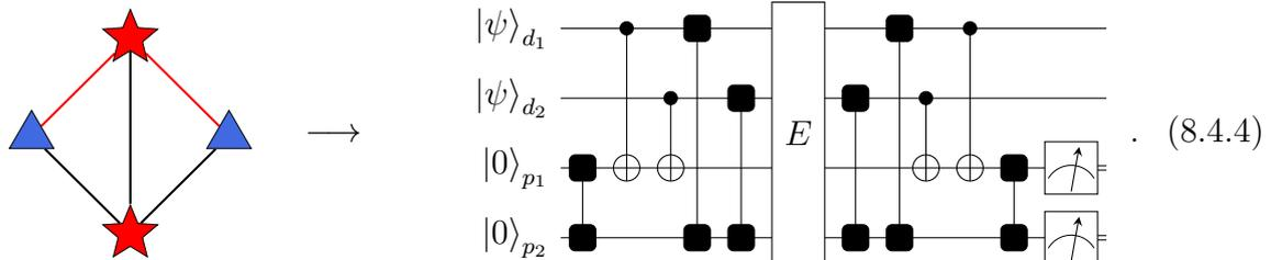
The above circuit is a  $[[4, 2, 2]]$  CPC code identical in form to the CPC code derived in section 4.2.
