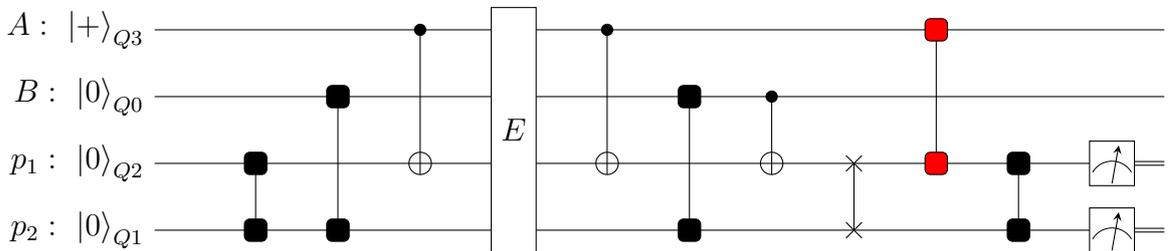
(c) A SWAP gate can be added to the  $[[4,2,2]]$  circuit to exchange the  $p_1$  and  $p_2$  parity qubits. This allows the ‘illegal’ operation marked in red in the decoder to be performed via a nearest-neighbour interaction.
