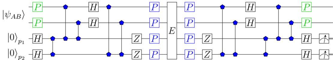
(d) The  $Z$  gates and blue  $P$  gates can be moved freely through the SP gates to the centre of the circuit. Due to their symmetry about the error window, the  $P$  and  $Z$  gates can be omitted from the code. The green  $P$  gates do not affect circuit operation and are also discarded.
