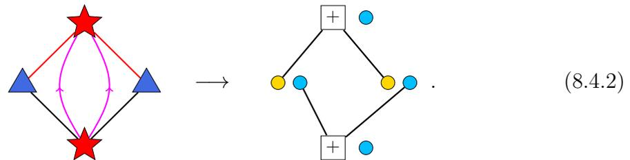
By inspection of the factor graph above, it is immediately clear that there are two bits that go unchecked, meaning the code has distance  $d = 1$ . This problem can be resolved by adding pairs of edges to the classical code until it has distance  $d = 2$ . An example
