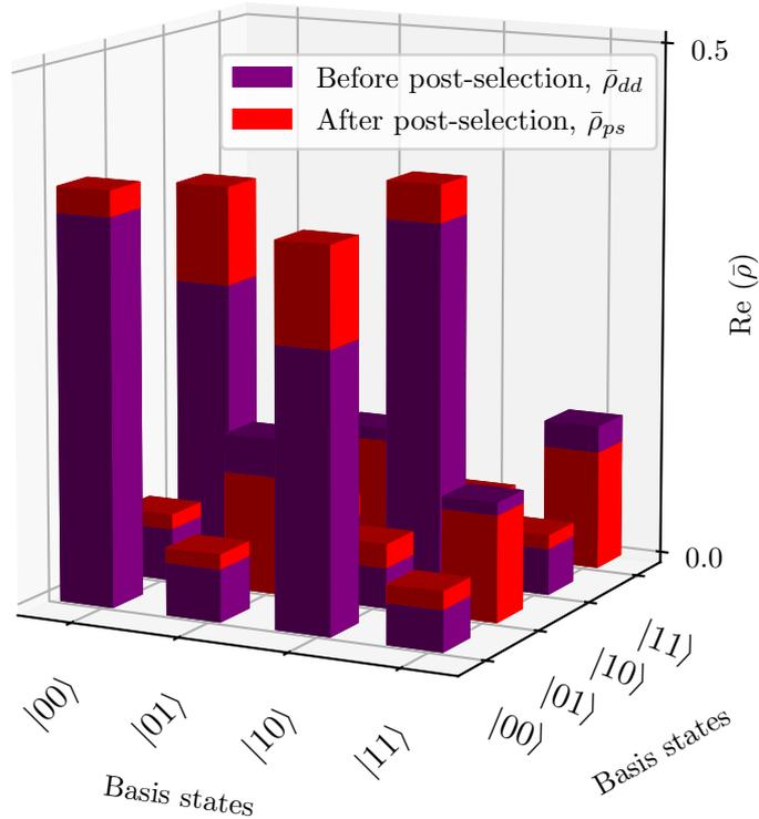
Figure 5.4: Plot of the real components of the density matrices  $\bar{\rho}_{dd}$  and  $\bar{\rho}_{ps}$  corresponding to the experimental output state. The height from the origin of the purple part of each bar shows the strength of the corresponding density matrix element before post-selection. The height from the origin of the red part of each bar shows the strength of the corresponding density matrix element after post-selection. *This figure was originally published in [2].*
