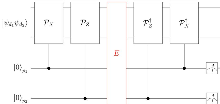
Figure 4.4: A preliminary CPC code formed by partitioning the encoder/decoder into two parity checking stages. The stage labelled  $\mathcal{P}_X$  detects  $X$ -errors on the register and the stage labelled  $\mathcal{P}_Z$  detects  $Z$ -errors on the register.
