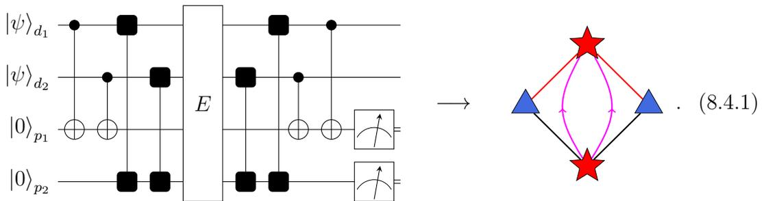
In the above, two virtual edges have been added between the parity qubits in accordance with the rule defined in equation 8.2.4. However, as these edges act in the same direction, they cancel each other out (see the simplification rule in table 8.1). Once the preliminary  $[[4, 2, 1]]$  CPC code has been mapped to the operational representation, it can be further mapped to a factor graph following the rules outlined in section 8.3, as shown below.
