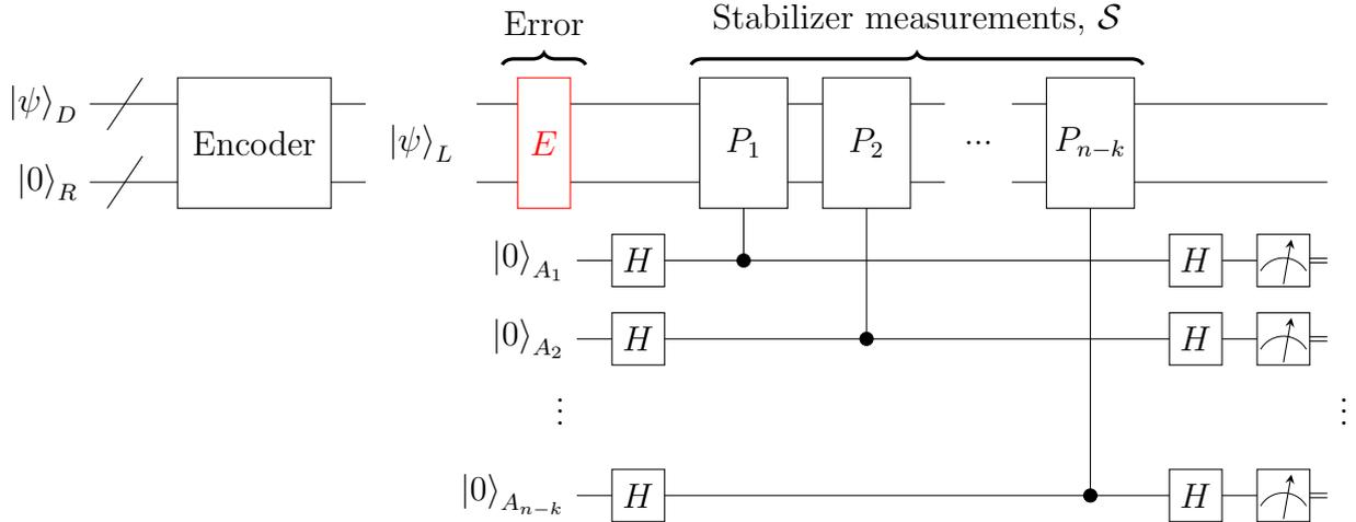
Figure 3.2: Circuit illustrating the structure of an  $[[n, k, d]]$  stabilizer code. A quantum data register  $|\psi\rangle_D = |\psi_1\psi_2\dots\psi_k\rangle$  is entangled with redundancy qubits  $|0\rangle_R = |0_10_2\dots0_{n-k}\rangle$  via an encoding operation to create a logical qubit  $|\psi\rangle_L$ . After encoding, a sequence of  $n - k$  stabilizer checks  $P_i$  are performed on the register to determine whether an error has occurred.
