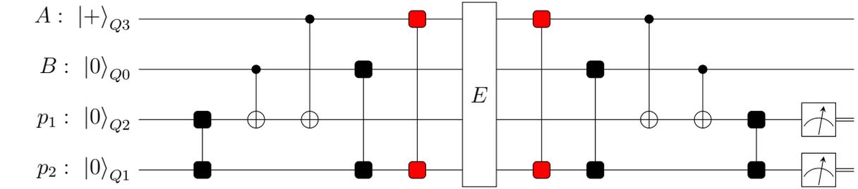
(a) The  $[[4,2,2]]$  CPC code with a  $|\psi_{AB}\rangle = |+_A 0_B\rangle$  input mapped onto the IBMQX4 chip. The red conjugate propagator gates are not possible according to the connectivity map for the IBMQX4 shown in figure 5.1.
