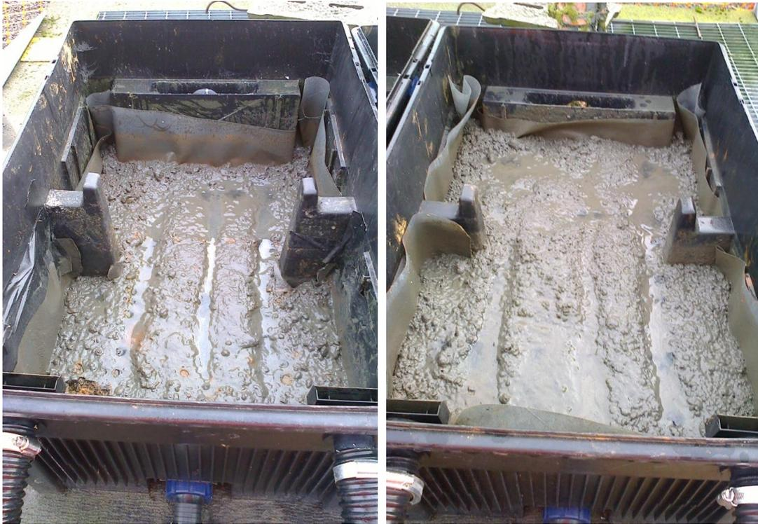
Figure 4.30: Comparison of the sludge build up on the ochre layer of the 5 cm (left) and 15 cm (right) units of Phase 2 of the pond filter trials.
