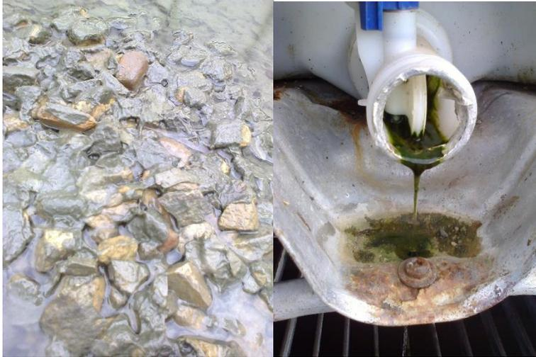
Figure 4.8: Sludge was observed on the gravel layer within the IBC trial unit (left) and algal growth occurred on the outlet pipe of the unit (right).
