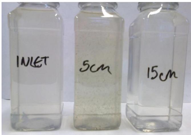
Figure 4.32: Comparison of effluent quality leaving the 5 cm and 5 cm pond filter units. A sample of the inlet effluent quality is also included. The samples were taken 14/11/16.
