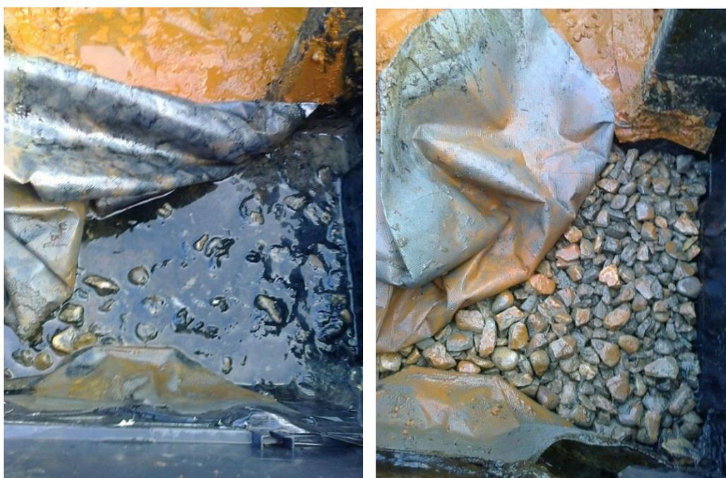
Figure 4.25: Comparison of the gravel layers in the downflow (left) and upflow (right) units. The downflow unit experienced sludge build up which is visible in the image above. The upflow unit did not experience this sludge build up.
