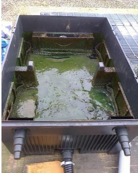
Figure 4.26: Sludge and algal build up on the adsorbent layer of upflow unit at the end of the phase 1 trial. Sludge and algal growth were also experienced on the downflow unit (not shown).
