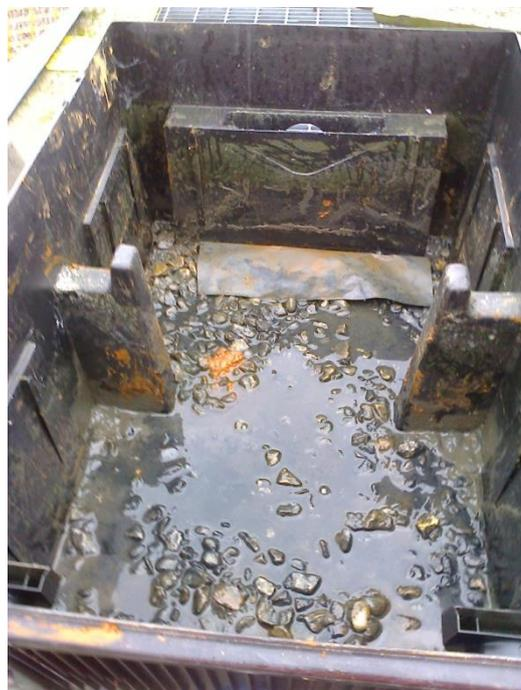
Figure 4.31: Sludge build up within the gravel layer of the 5 cm ochre layer unit is shown in the image above and was visible once the ochre layer was removed at the end of the Phase 2 trial period.
