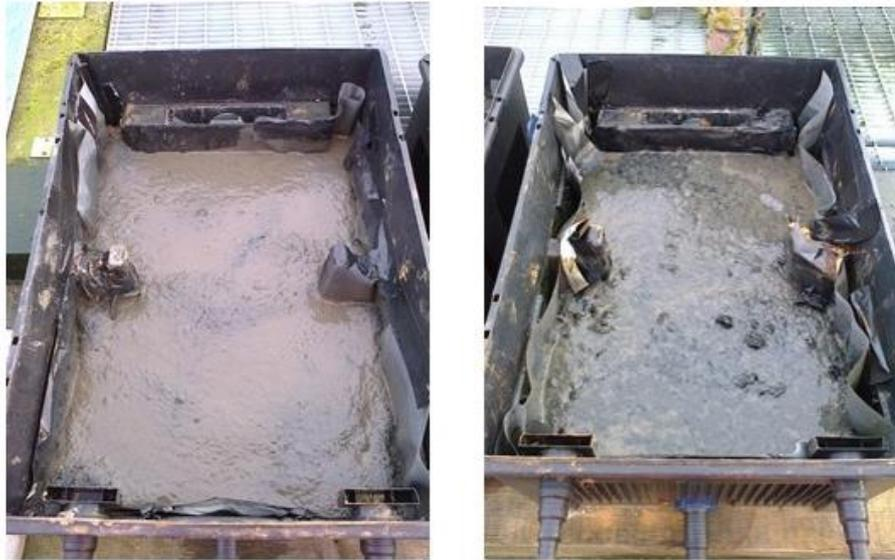
Figure 4.36: Comparison of the sludge layer on the sand (left) and ochre (right) units at the end of Phase 3 of the pond filter trials.
