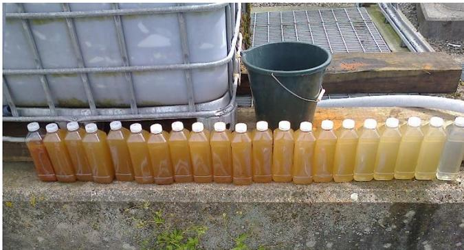
Figure 4.9: Samples taken of the first flush of effluent through the IBC unit (taken at the outlet of the unit). There were 20 samples taken in slowly and these are shown in the above image from the first litre on the left to the twentieth on the right. The final sample on the right of the image is a sample of the site's final effluent for comparison.
