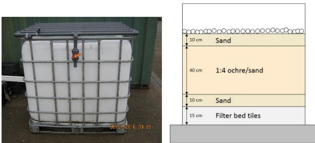
Figure 3.4: Left; empty IBC unit, right; intended layers to be packed within the IBC
