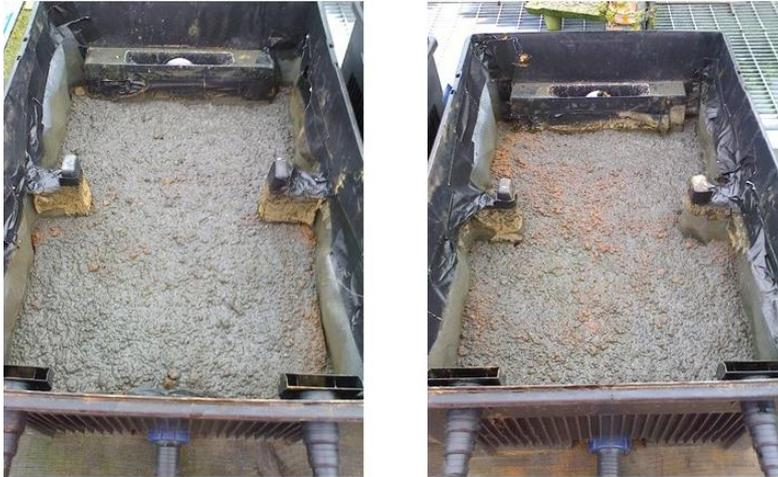
Figure 4.40: Observed sludge layer on the ochre layer of the Phase 4a units at the end of the trial.
