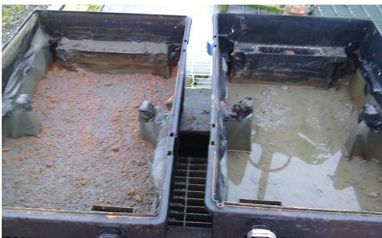
Figure 4.41: Sludge on the ochre layer of the Phase 4b units observed at the end of the trial.
