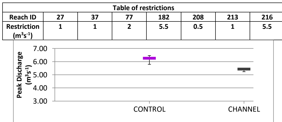
Figure 7.6 Graph showing results of channel gradient-driven flow restrictions according to table of restrictions above.
