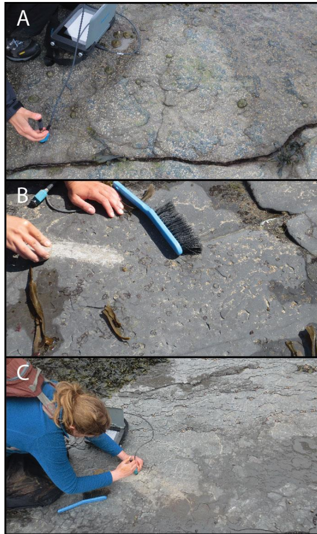
Figure 3.15 Acquisition of the rock hardness data with the Equotip durometer: A) taking readings from a weathered surface; B) removing the weathered surface with the carborundum stone; C) taking readings from an un-weathered surface.
