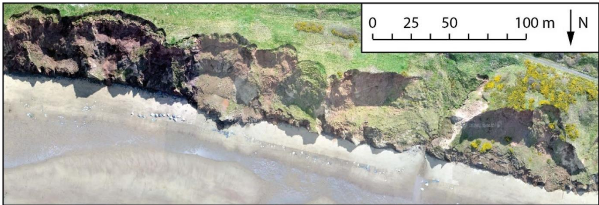
Figure 3.4 Landslide complex on cliff face composed of glacial till, Whitby Golf Club (Upgang), North Yorkshire; LiDAR 2016 orthophotograph mosaic.
