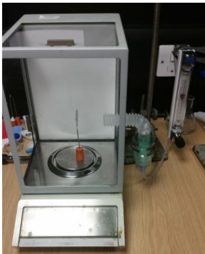
Figure 56: Image highlighting the experimental setup with the custom built stand, sample, nebulizer, tubing, and flow meter. The compressor unit is mounted on an adjacent bench
