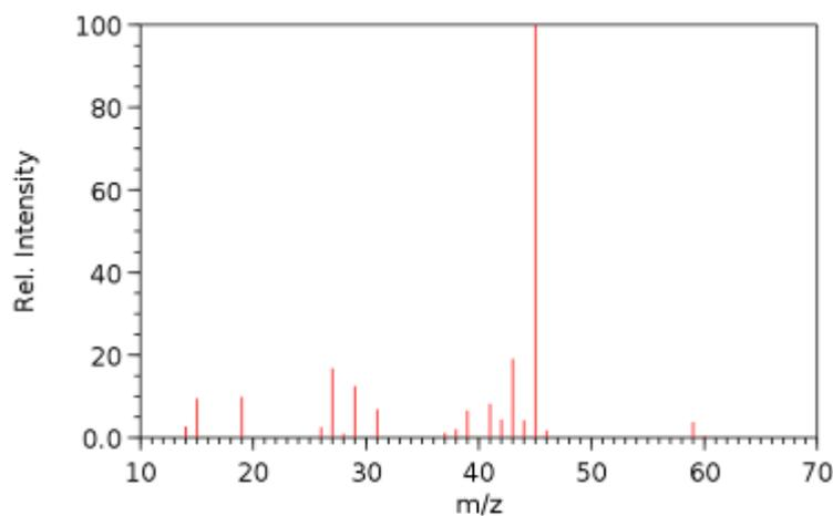
Figure 70: Literature mass spectrum of propan-2-ol taken from NIST database. Intensity of peaks is given relative to the base peak at m/z 45 Da.<sup>430</sup>
