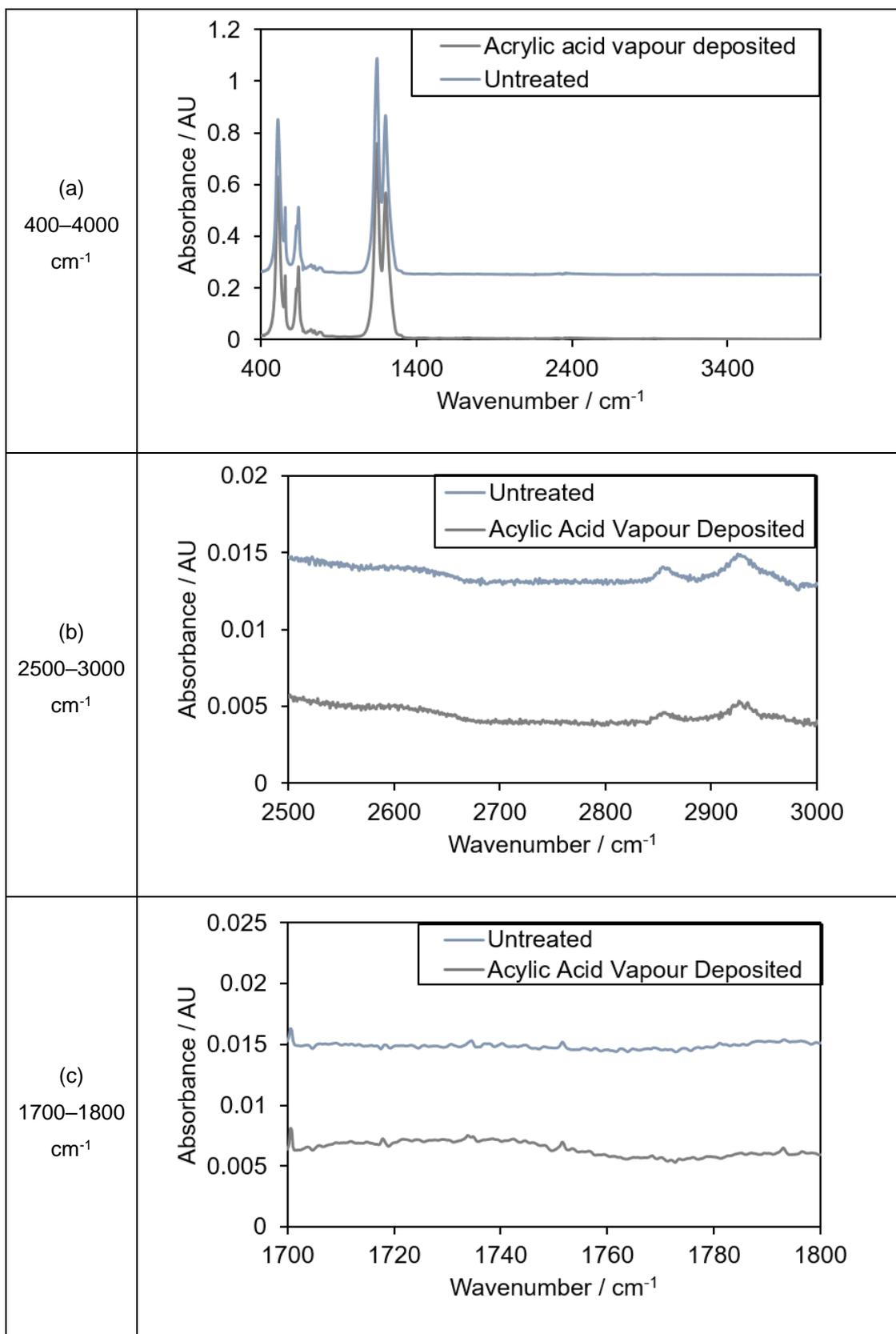
Figure 62: FTIR of untreated washed PTFE and DBD plasma-treated (nitrogen flowing through ammonia water,  $20 \text{ cm}^3 \text{ min}^{-1}$ , 14 kV, 3 kHz, 300 s) PTFE after 24 h exposure to AA monomer vapour. (a) full spectra;  $400\text{--}4000 \text{ cm}^{-1}$ , (b) carboxylic acid OH stretch region;  $2500\text{--}3000 \text{ cm}^{-1}$ , (c) carbonyl stretch,  $1700\text{--}1800 \text{ cm}^{-1}$ .
