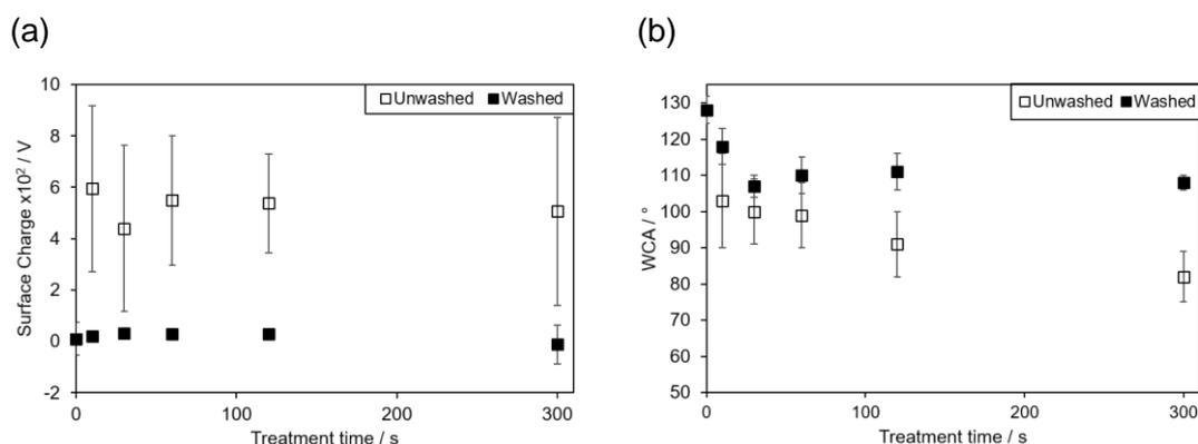
Figure 51: Effect of treatment time on (a) surface potential, and (b) WCA achieved after DBD plasma using flowing argon bubbling through water (14 kV, 3 kHz, 5–300 s, 20 cm<sup>3</sup> min<sup>-1</sup>), immediately after treatment (□), and after washing in propan-2-ol/cyclohexane (1:1 solution by volume, 2 min) and air drying (60 min, (■)). Error bars denote standard deviation of the sample.
