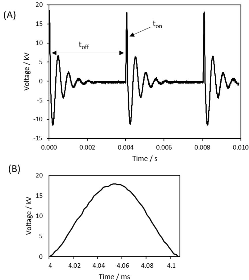
Figure 39: Characteristics of standard pulse of DBD rig. (A) was measured by Kelvin Appleby using Tektronix Ltd. MDO4104-3 oscilloscope, March 2016. (B) is a close up of the pulse shape, showing the applied 17.5 kV pulse time duration is 100  $\mu$ s (prior to ringing). This is measured using a separate circuit connect in parallel to the electrodes. The measured voltage is the applied voltage to the moveable electrode when there is no plasma ignited, see (C) in Figure 40.
