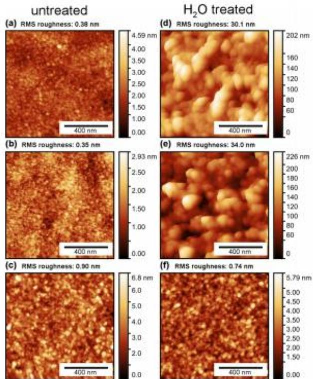
Figure 65: AFM images of untreated and H<sub>2</sub>O stored Al<sub>2</sub>O<sub>3</sub> coated Si (100) samples: (a) as synthesized; (b) 450 °C annealed; and (c) 900 °C annealed. (d-f) AFM images of the same samples as (a-c) after storage in 18 MΩ water for 47 days. Al<sub>2</sub>O<sub>3</sub> deposited on Si (100) surface using ALD from TMA and H<sub>2</sub>O at 150 °C.<sup>384</sup>
