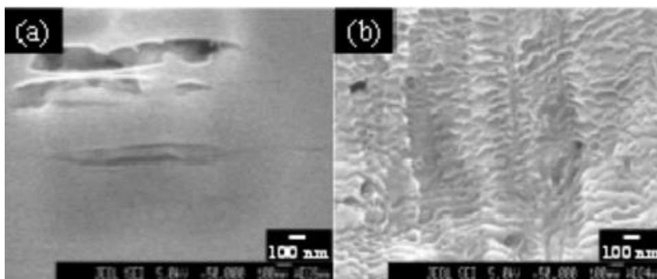
Figure 18: FE-SEM images at 50 000 magnification and 5.0 kV electron acceleration voltage of PTFE (a) as received, WCA  $118^\circ$ , and (b) treated with Ar/NH<sub>3</sub>-H<sub>2</sub>O plasma (100 W, 15 min, 0.8 mbar), WCA  $4^\circ$ .<sup>147</sup>
