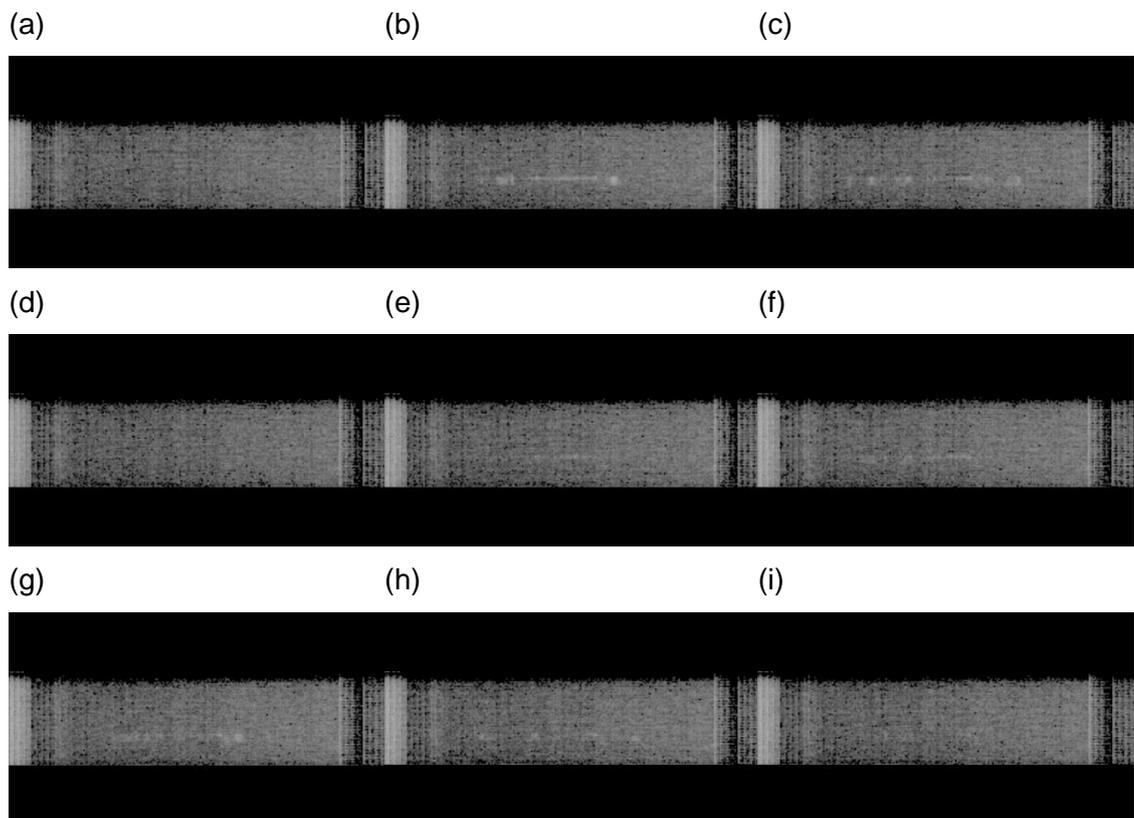
Figure 48: Frame by frame capture of DBD plasma (static air, 14 kV, 3kHz). Recorded using FASTCAM-APX RS Model 250 k. Record rate 36000 fps, and shutter speed  $2.8 \times 10^{-5}$  s. (a) no plasma; (b) and (c) positive voltage plasma; (d) no plasma; (e), (f), (g), and (h) lower intensity negative voltage “ringing” plasma; and (i) no plasma. Thanks go to Dr. Lisong Yang and Professor Colin Bain for their help in obtaining these images.
