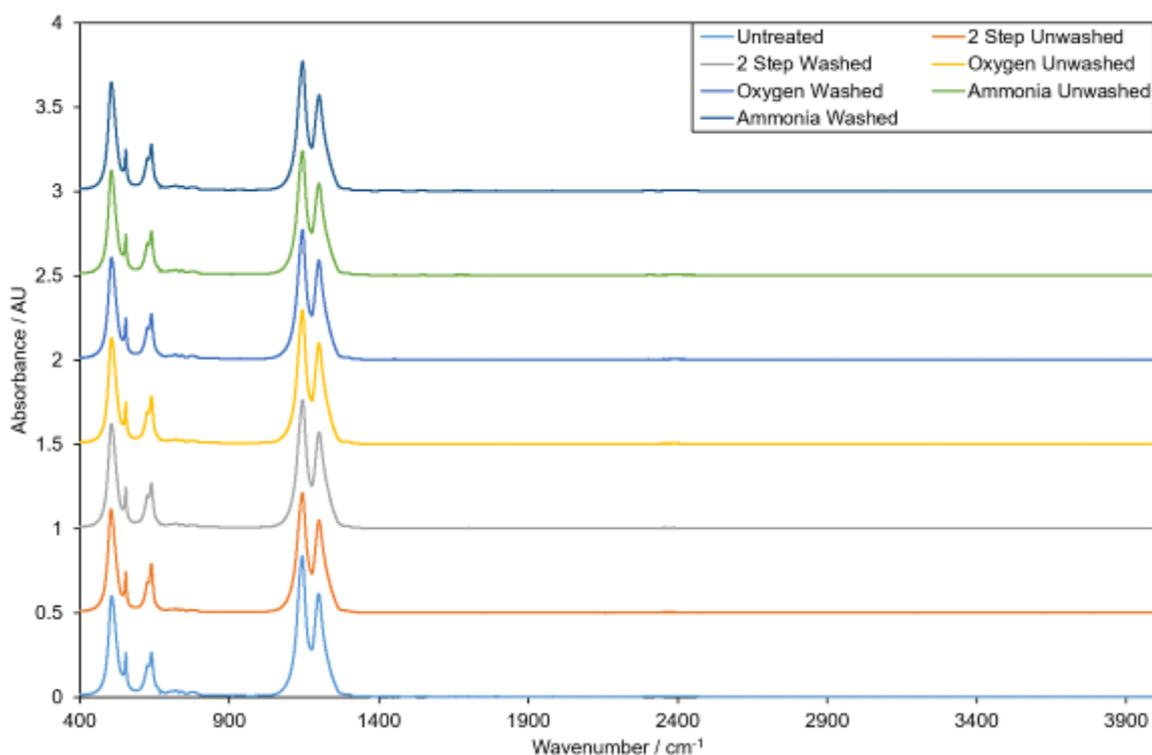
Figure 30: Stacked FTIR-ATR of untreated and plasma-treated PTFE.
