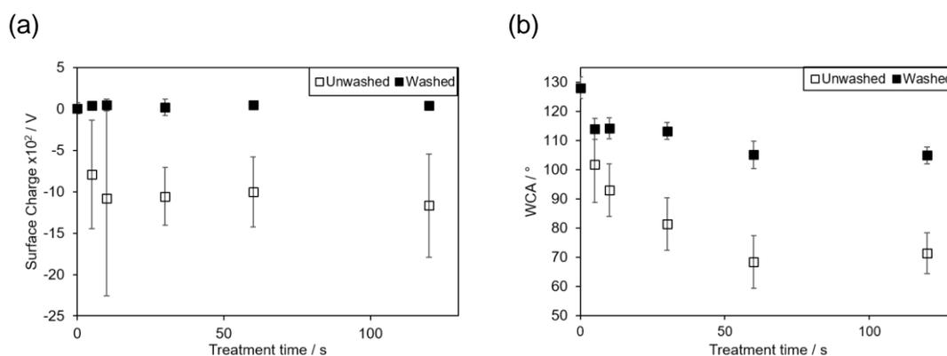
Figure 45: Effect of treatment time on (a) surface potential, and (b) WCA achieved after DBD plasma using flowing nitrogen (14 kV, 3 kHz, 5–120 s,  $20 \text{ cm}^3 \text{ min}^{-1}$ ), immediately after treatment ( $\square$ ), and after washing in propan-2-ol/cyclohexane (1:1 solution by volume, 10 s) and air drying (60 min,  $\blacksquare$ ). Error bars denote standard deviation of the sample.
