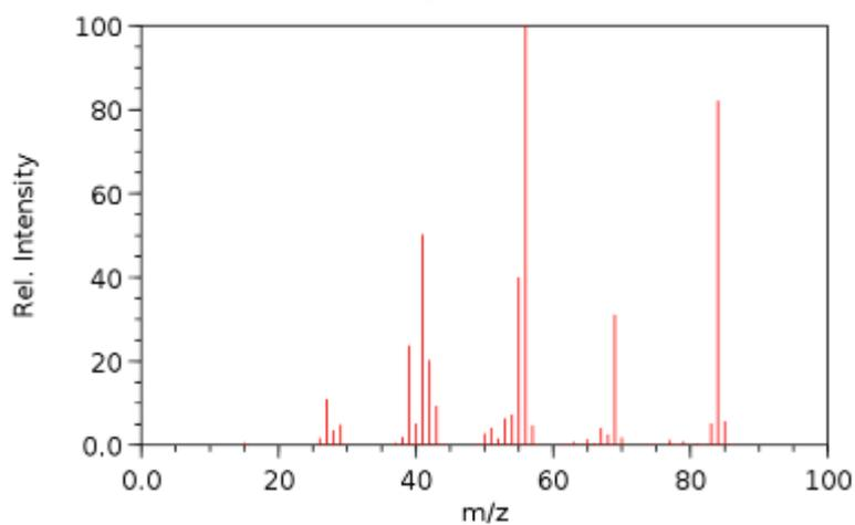
Figure 72: Literature mass spectrum of cyclohexane taken from NIST database. Intensity of peaks is given relative to the base peak at m/z 56 Da.<sup>430</sup>
