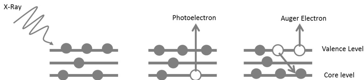
Figure 11: Schematic representation of photoemission process of XPS.<sup>106</sup> The wavy line represents the X-ray incident on the sample. The grey circles represent electrons in core and valence levels. The white circles indicate holes where electrons used to be.
