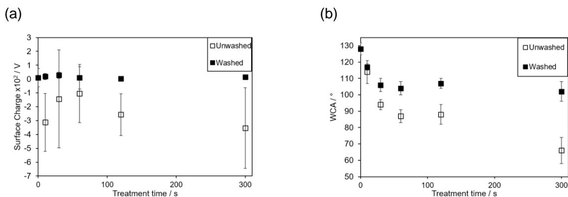
Figure 52: Effect of treatment time on (a) surface potential, and (b) WCA achieved after DBD plasma using helium bubbling through water (14 kV, 3 kHz, 5–300 s, 20 cm<sup>3</sup> min<sup>-1</sup>), immediately after treatment (□), and after washing in propan-2-ol/cyclohexane (1:1 solution by volume, 2 min) and air drying (60 min, (■)). Error bars denote standard deviation of the sample.
