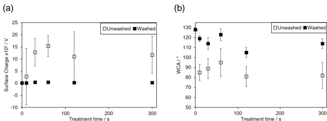
Figure 50: Effect of treatment time on (a) surface potential, and (b) WCA achieved after DBD plasma using nitrogen bubbling through water ( $14$  kV,  $3$  kHz,  $5$ – $300$  s,  $20$  cm<sup>3</sup> min<sup>-1</sup>), immediately after treatment ( $\square$ ), and after washing in propan-2-ol/cyclohexane (1:1 solution by volume, 2 min) and air drying (60 min, ( $\blacksquare$ )). Error bars denote standard deviation of the sample.
