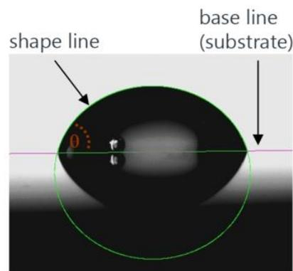
Figure 7: Image of droplet on a substrate surface. The baseline is shown in pink, and the calculated geometric model is shown in green. The CA is indicated by the orange angle labelled  $\theta$ . Image reported by Kruss-Scientific.<sup>22</sup>
