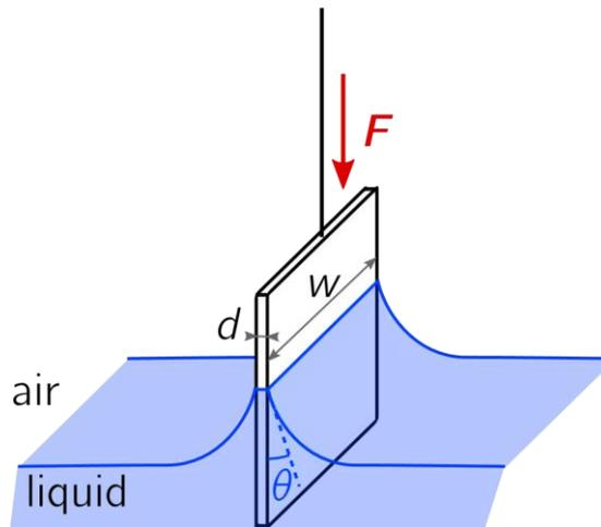
Figure 8: Schematic of Wilhelmy plate method. Shown is the vertical plate being pushed into the liquid, and labelled is the CA ( $\theta$ ). Source: WikiCommons.<sup>32</sup>
