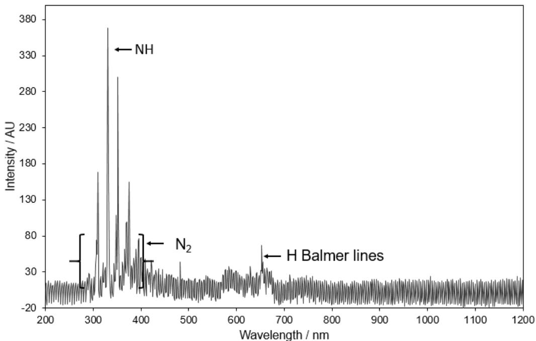
Figure 22: OES of NH<sub>3</sub> plasma (50 W, 5 mins, 0.2 mbar). Labelled are the significant peaks as labelled in NH<sub>3</sub> OES by S. Kang *et al.*<sup>202</sup>
