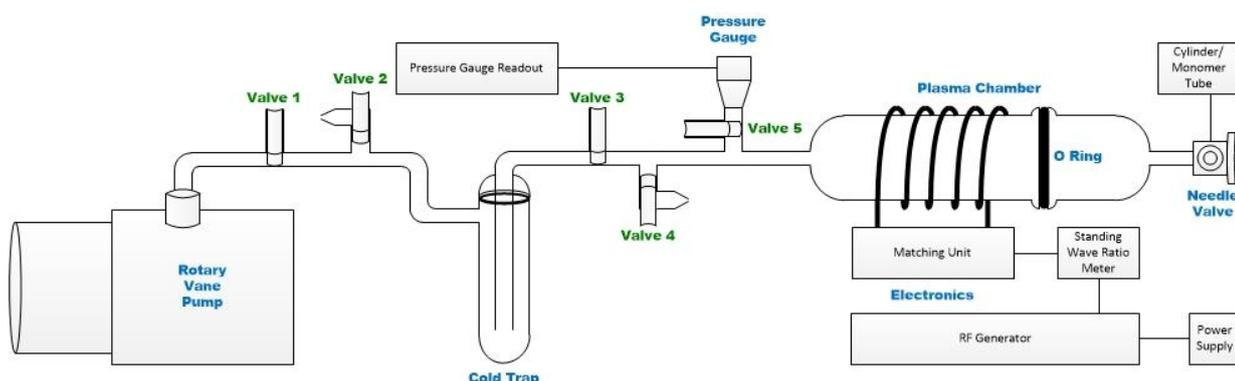
Figure 19: Schematic representation of low-pressure plasma reactor. Created by James Wizzell and reproduced with thanks.
