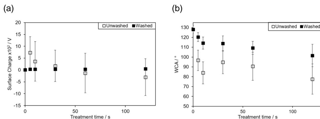
Figure 49: Effect of treatment time on (a) surface potential, and (b) WCA achieved after DBD plasma using air that has flowed through a water bubbler (14 kV, 3 kHz, 5–120 s, 20 cm<sup>3</sup> min<sup>-1</sup>), immediately after treatment (□), and after washing in propan-2-ol/cyclohexane (1:1 solution by volume, 10 s) and air drying (60 min, (■)). Error bars denote standard deviation of the sample.
