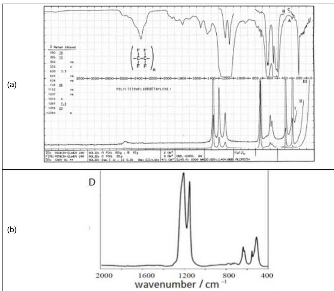
Figure 32: Literature FTIR spectra of PTFE. (a) FTIR and Raman spectra by D. Lin-Vien *et al.*<sup>210</sup> (b) FTIR absorbance spectrum by D.D. Fazullin *et al.*<sup>211</sup>
