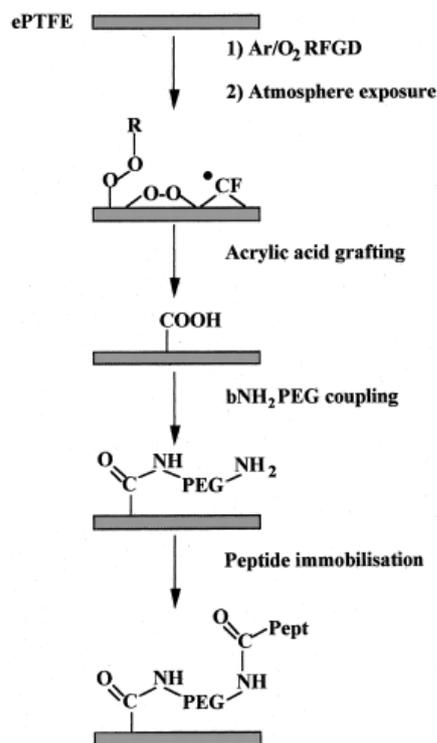
Figure 58: Schematic mechanism proposed by Ch. Baquey *et al.* of how a plasma step can be used in conjunction with a monomer grafting step for use in vascular graft applications.<sup>346</sup>
