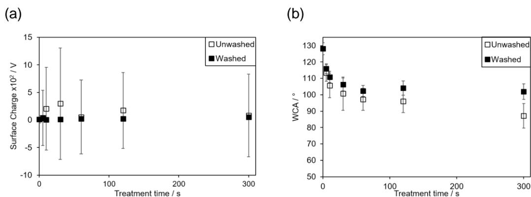
Figure 47: Effect of treatment time on (a) surface potential, and (b) WCA achieved after DBD plasma using flowing helium (14 kV, 3 kHz, 5–300 s, 20 cm<sup>3</sup> min<sup>-1</sup>), immediately after treatment (□), and after washing in propan-2-ol/cyclohexane (1:1 solution by volume, 10 s) and air drying (60 min, (■)). Error bars denote standard deviation of the sample.
