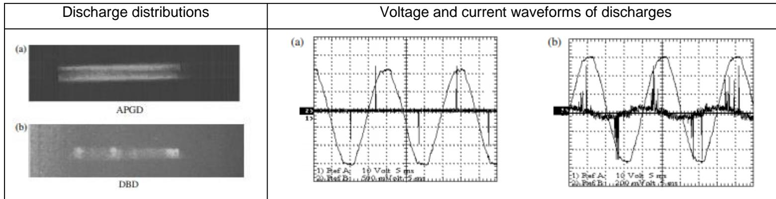
Figure 35: Shown is the (a) homogenous APGD discharge and (b) the non-homogenous filamentary DBD discharge with a 2 mm air gap between electrodes and an applied voltage of 6.5 kV.<sup>260</sup>
