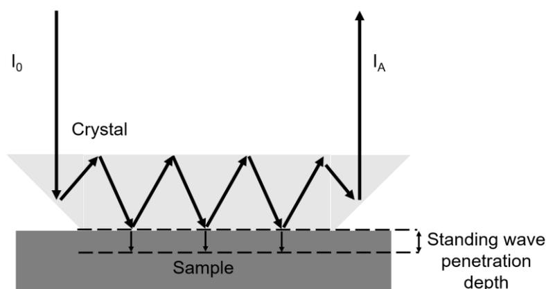
Figure 15: Total internal reflection of  $I_0$  within the Diamond cut KSR-5 (thallium bromiodide) crystal, and the resultant standing wave that penetrates the sample. Adapted from schematic by S. Morsch.<sup>89</sup>
