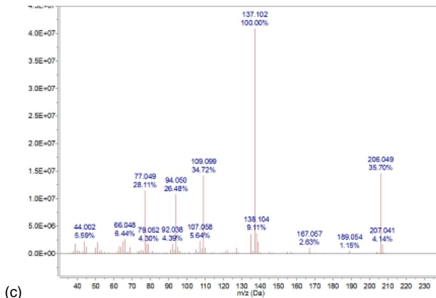
Figure 73: GC-MS results for solvent background (propan-2-ol and cyclohexane 1:1 v/v solution). Shown is (a) the graph showing the retention time of the solvent in the column, and both (b) the whole m/z spectrum (35–650 Da), and (c) the zoomed in image (35–235 Da).
