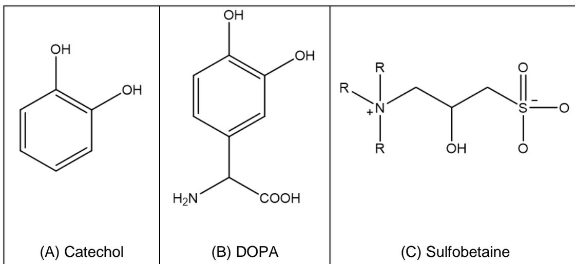
Figure 59: Basic structures of grafting monomers. (A) Catechol functional group, (B) DOPA molecule. (C) Basic sulfobetaine zwitterionic molecule.
