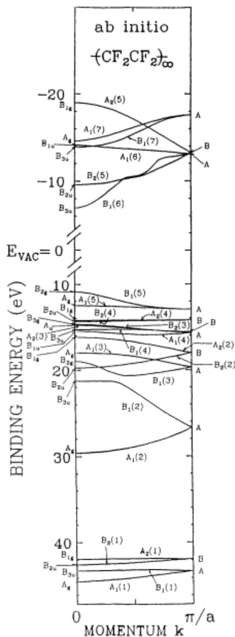
Figure 37: Energy band structure of PTFE chain in planar zig-zag formation (not helical) as reported by K. Seki *et al.*<sup>281</sup>
