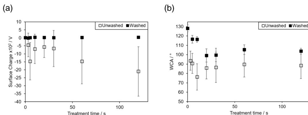
Figure 43: Effect of treatment time on (a) surface potential, and (b) WCA after DBD plasma air (14 kV, 3 kHz, 5–120 s), under static air conditions. Measurements made immediately after treatment ( $\square$ ), and after washing in propan-2-ol/cyclohexane (1:1 solution by volume, 10 s) and air drying (60 min, ( $\blacksquare$ )). Error bars denote standard deviation of the sample.
