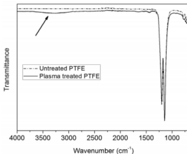
Figure 29: FTIR-ATR (Nicolet iS10, Thermo Scientific, fitted with ATR sampling accessory (Smart iTR), 32 scans and a resolution of  $2\text{ cm}^{-1}$ ) spectra of untreated and oxygen plasma-treated PTFE (200 W, 600 s, 0.09 mbar). Arrow points to region where the OH containing bands are present.<sup>176</sup>
