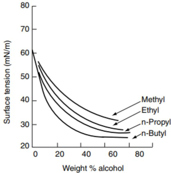
Figure 16: Effect of carbon chain length on the surface tension of water. Here illustrated using methanol, ethanol, propanol, and butanol. Taken from work by D. Myers.<sup>130</sup>
