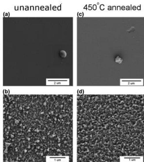
Figure 66: SEM images of unannealed (as deposited) and 450 °C annealed alumina surfaces: (a) as deposited; (b) as deposited after 63 days in water; (c) 450 °C annealed; and (d) 450 °C annealed after 63 days in water. Al<sub>2</sub>O<sub>3</sub> deposited on Si (100) surface using ALD from TMA and H<sub>2</sub>O at 150 °C.<sup>384</sup>
