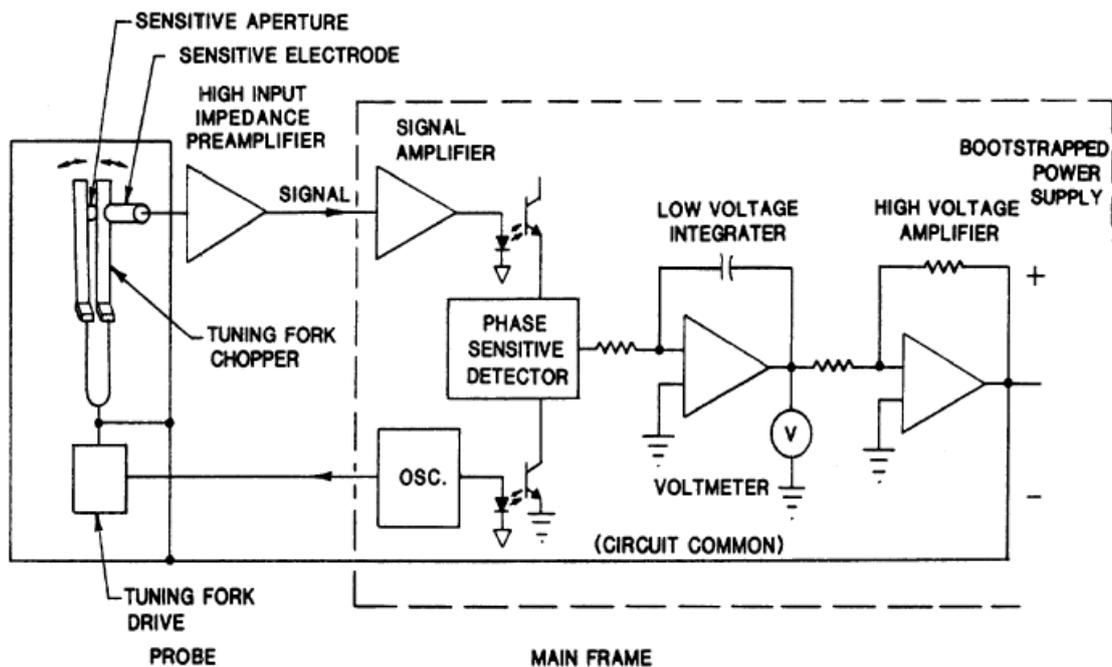
Figure 17: Simplified block circuit diagram of electrostatic voltmeter, Monroe Electronics Isoprobe 244.<sup>132</sup>
