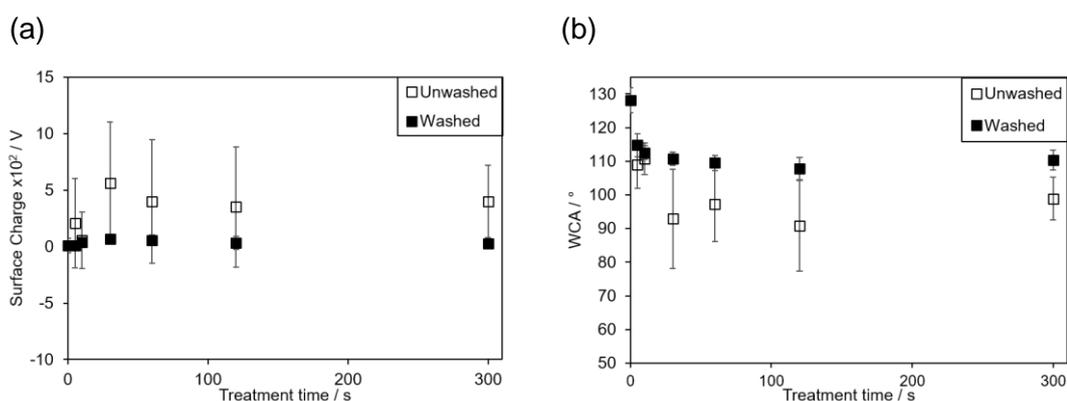
Figure 46: Effect of treatment time on (a) surface potential, and (b) WCA achieved after DBD plasma using flowing argon (14 kV, 3 kHz, 5–300 s, 20 cm<sup>3</sup> min<sup>-1</sup>), immediately after treatment (□), and after washing in propan-2-ol/cyclohexane (1:1 solution by volume, 10 s) and air drying (60 min, (■)). Error bars denote standard deviation of the sample.
