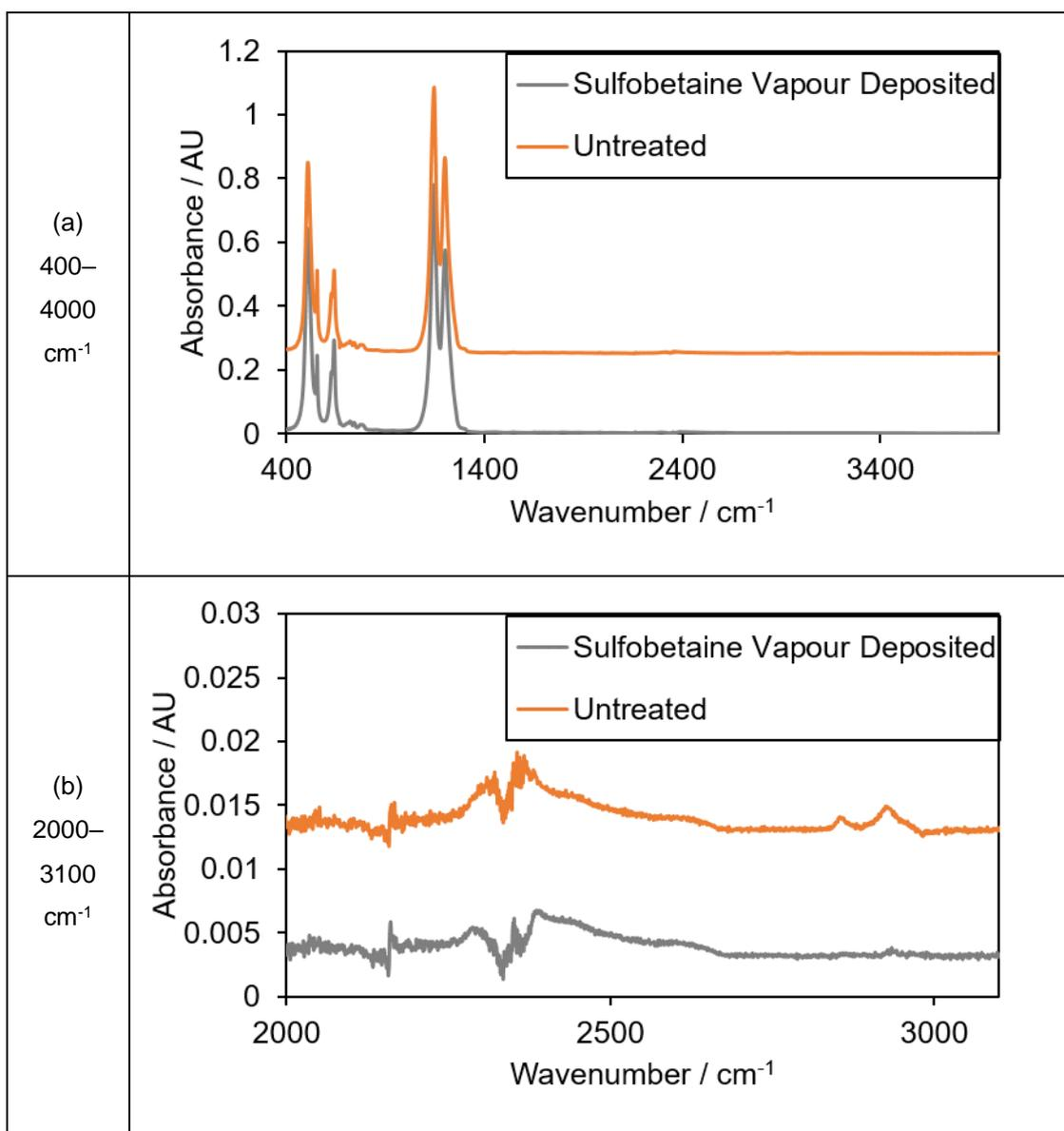
Figure 63: ATR-FTIR of untreated washed PTFE and DBD plasma-treated (nitrogen flowing through ammonia water,  $20\text{ cm}^3\text{ min}^{-1}$ , 14 kV, 3 kHz, 300 s) PTFE after 24 h exposure to aqueous sulfobetaine solution (1 wt%) vapour. (a) Full spectrum;  $400\text{--}4000\text{ cm}^{-1}$ , and (b) C-H stretch region;  $2000\text{--}3100\text{ cm}^{-1}$ .<sup>369</sup>
