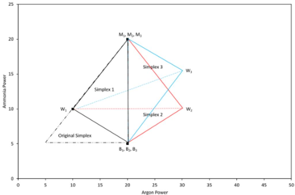
Figure 68: Simplex plasma power optimization map for fixed treatment time (120 s Ar plasma, then 120 s NH<sub>3</sub> plasma, 0.2 mbar) using a different simplex triangle size to improve the optimization further. The original simplex is shown by the dashed black triangle, this
