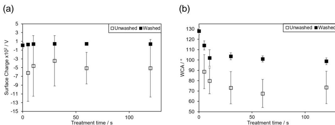
Figure 44: Effect of treatment time on (a) surface potential, and (b) WCA achieved after DBD plasma using flowing air (14 kV, 3 kHz, 5–120 s, 20 cm<sup>3</sup> min<sup>-1</sup>), immediately after treatment (□), and after washing in propan-2-ol/cyclohexane (1:1 solution by volume, 10 s) and air drying (60 min, (■)). Error bars denote standard deviation of the sample.
