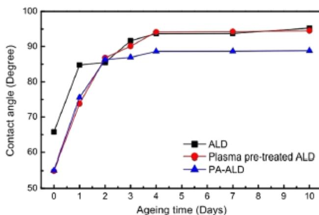
Figure 64: Effect of ageing time on plasma-treated ALD and ALD treated PET surfaces.<sup>383</sup>
