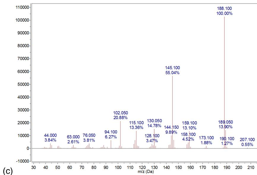
Figure 69: GC-MS results for solvent background (propan-2-ol alone). Shown is (a) the graph showing the retention time of the solvent in the column, and both (b) the whole m/z spectrum (35–650 Da), and (c) the zoomed in image (30–215 Da).
