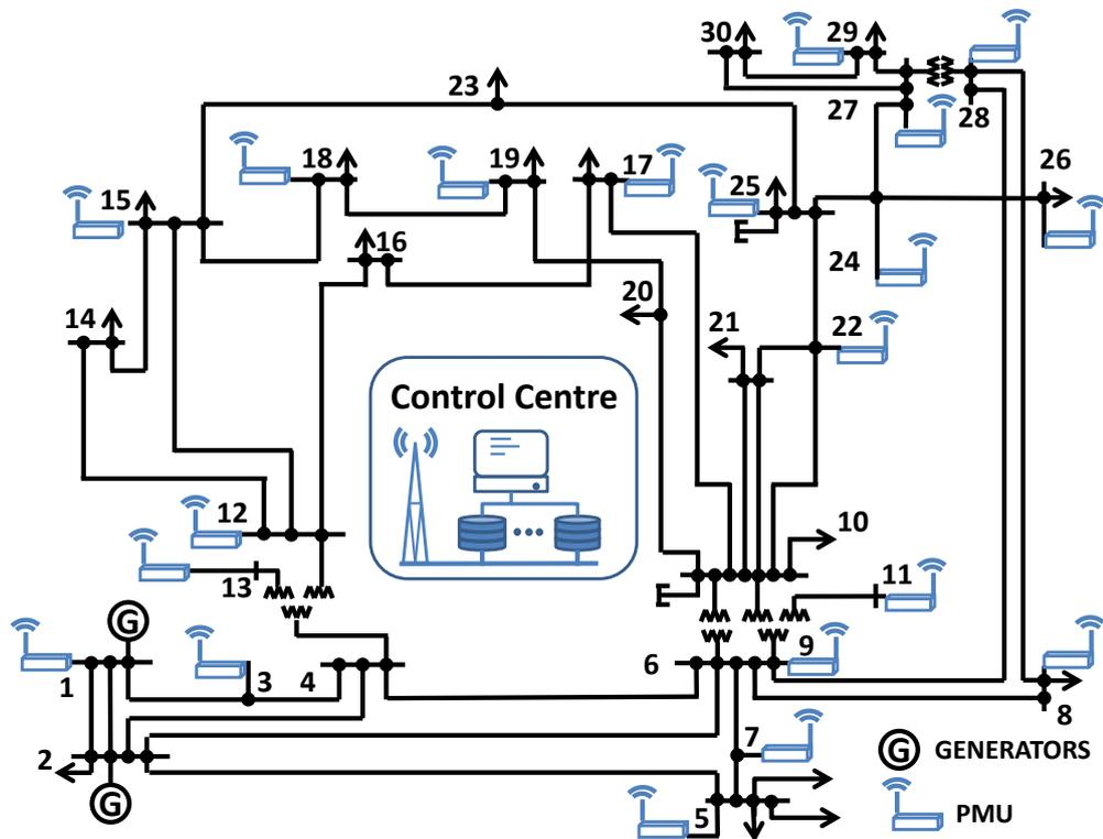
Figure 5.6: IEEE 30 bus power system with 21 PMUs.
