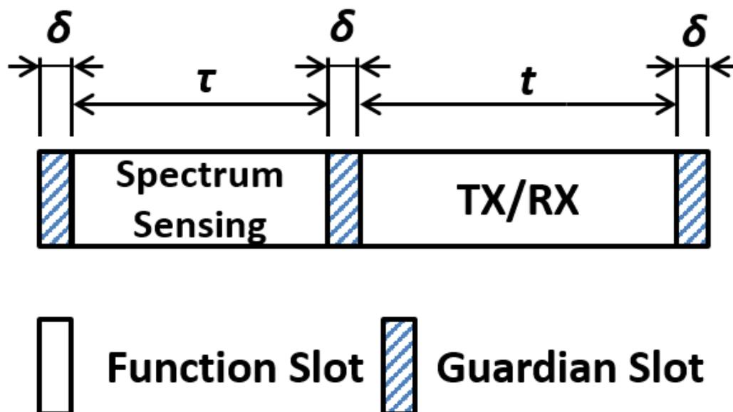
Figure 6.4: The frame of spectrum sensing enabled communication network consists of spectrum sensing slot, data transmission and reception slot and guardian slot.
