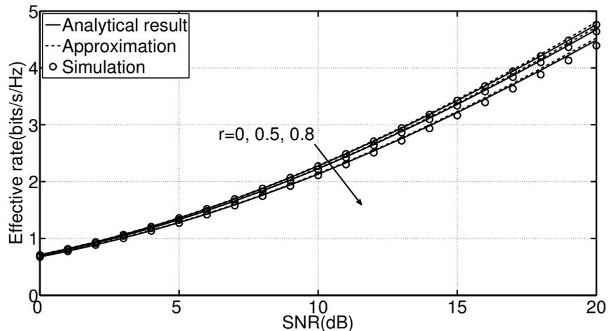
Figure 4.5: Effective rate under correlated generalized  $K$  fading channel with different correlation coefficients  $r = 0, 0.5, 0.8$  and  $N = 2$ , where approximation results are compared to analytical results and simulation results.
