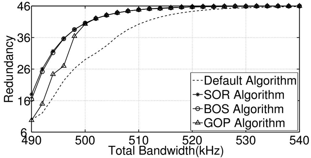
Figure 5.7: System observability redundancy performance in IEEE 30 bus case.
