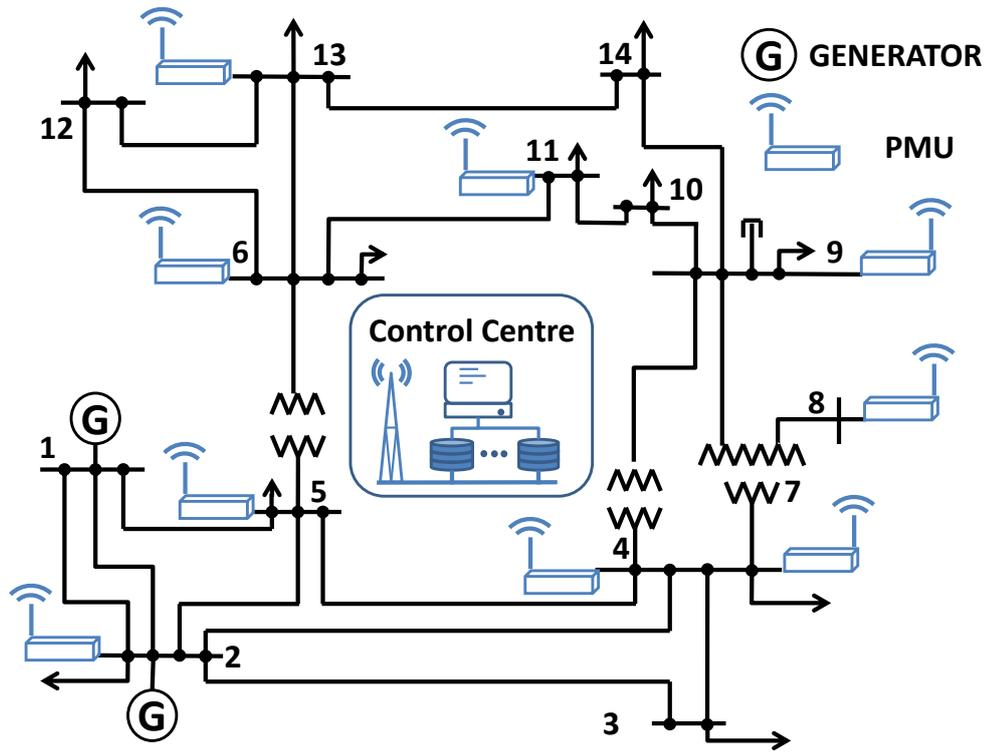
Figure 5.1: IEEE 14 bus power system with 9 PMUs.
