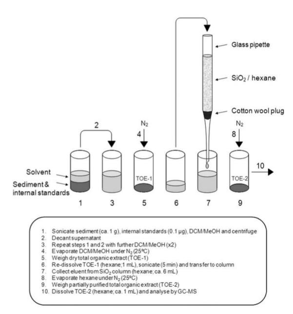
**Figure 3.1:** Diagram showing the process of extraction and partial purification of IP<sup>25</sup> from sediment extracted from GC01. (Taken from Belt, 2012).
