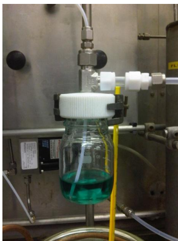
Figure 10 Small scale fluorination process set-up with magnetic stirring
