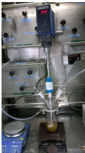
Figure 9 Large scale fluorination process set-up with mechanical stirring
