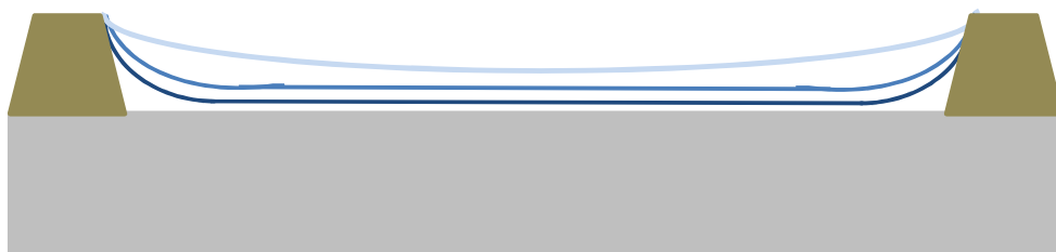
Figure 3.6: A schematic diagram showing the changing radius of curvature as the drying film thins. Darker blue lines represent later stages in the drying process.
