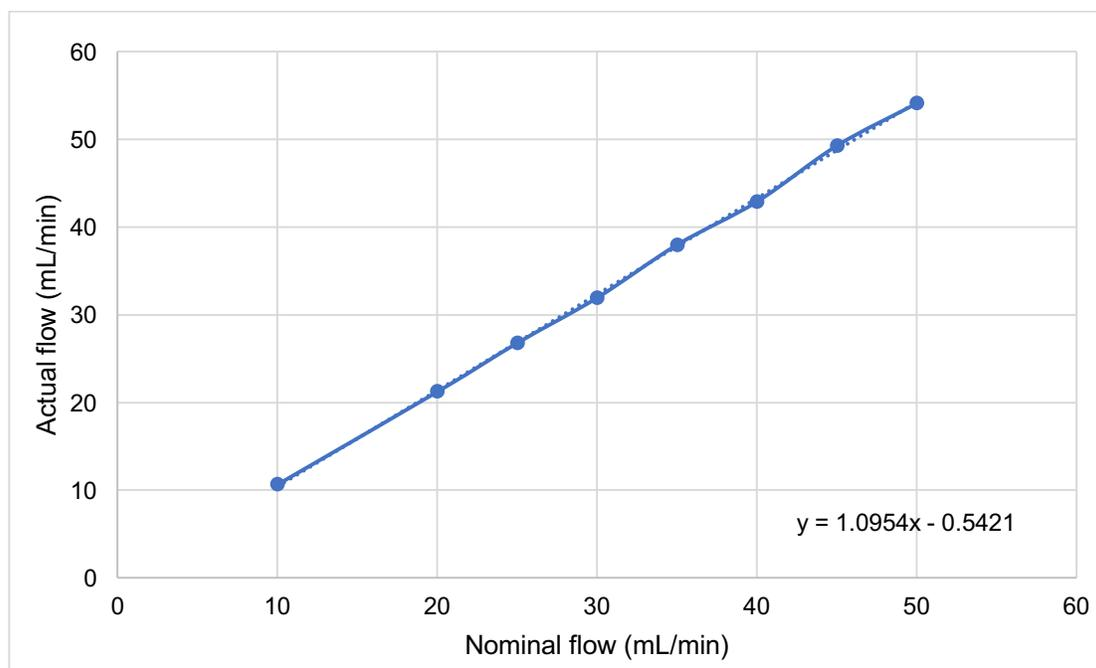
**Figure 4.** Experimentally-determined argon MFC calibration curve
