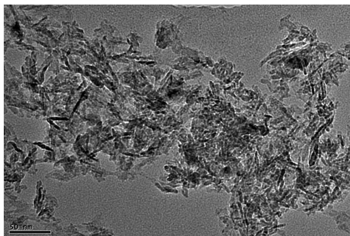
**Figure 10.** TEM image of sample CP2 (5% Co/Al<sub>2</sub>O<sub>3</sub> catalyst)
