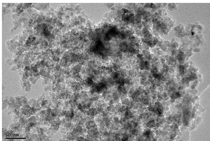
**Figure 9.** TEM image of sample CP1 (5% Co/SiO<sub>2</sub> catalyst)
