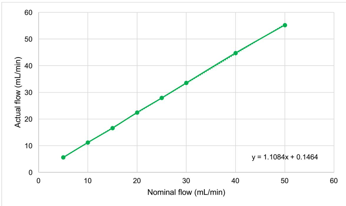
**Figure 6.** Experimentally-determined carbon monoxide MFC calibration curve
