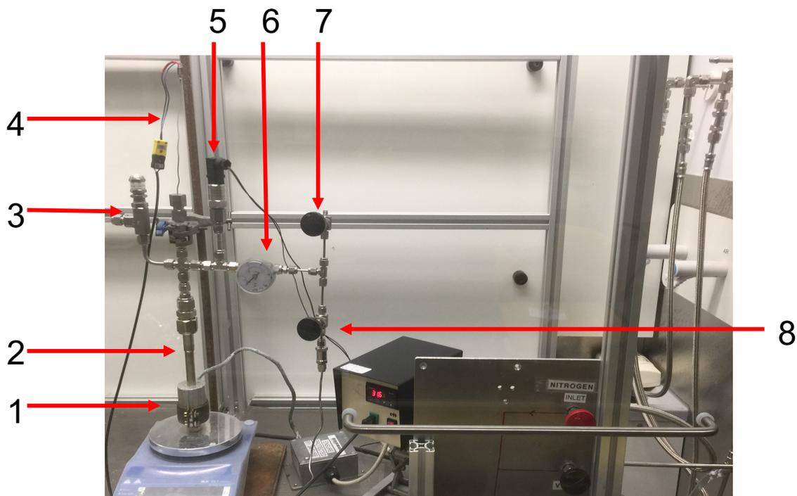
**Figure 3.** Picture of the reactor system used for catalytic testing of APFTS with components as labelled in Figure 2.
