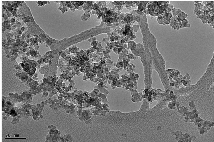
**Figure 11.** TEM image of sample CP3 (10% Co/SiO<sub>2</sub> catalyst)
