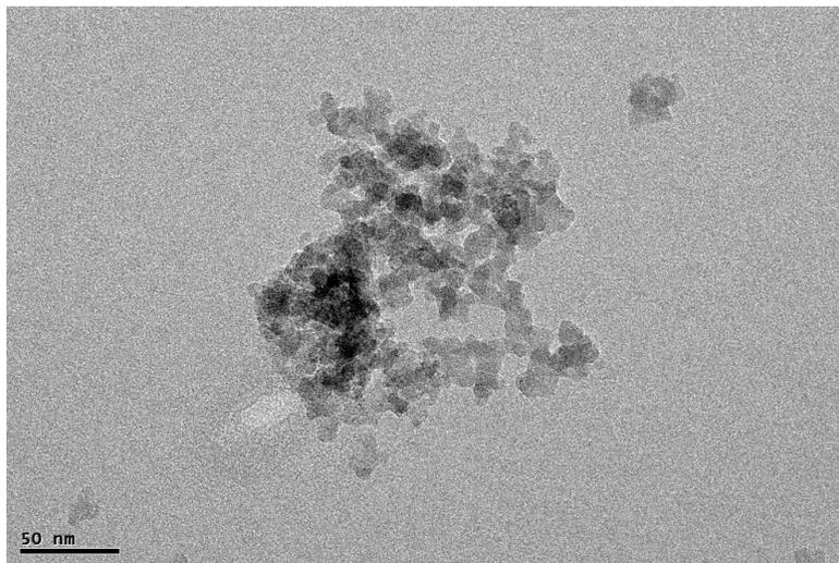
**Figure 12.** TEM image of sample CP5 (10% Co/SiO<sub>2</sub> catalyst)
