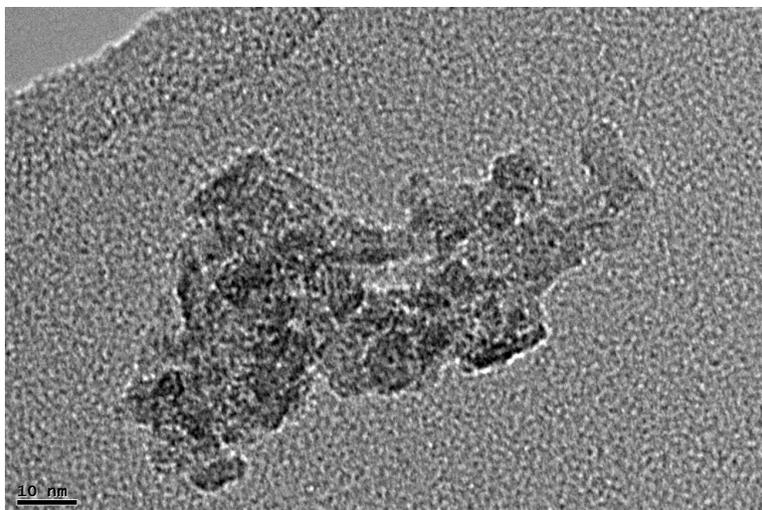
**Figure 13.** TEM image of sample CP6 (10% Co/Al<sub>2</sub>O<sub>3</sub> catalyst)
