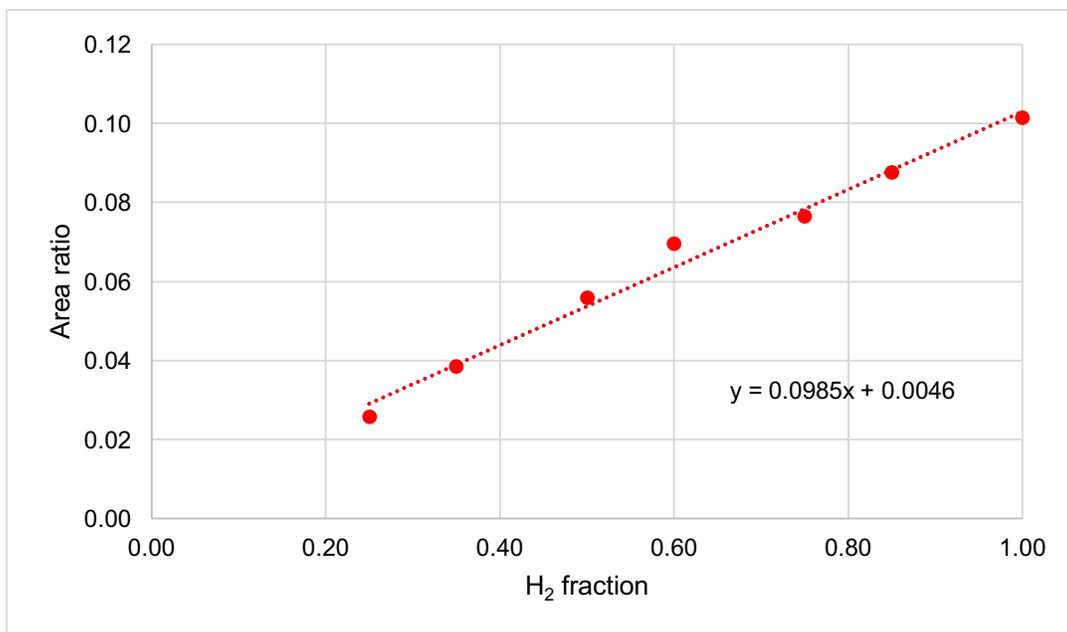
**Figure 8.** Experimentally-determined calibration curve to calculate the H<sub>2</sub> fraction converted based on the area ratio of H<sub>2</sub>/Ar
