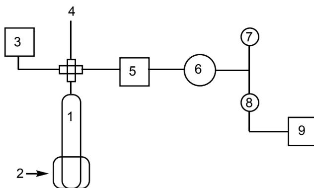
**Figure 2.** Reactor system used for catalytic testing of APFTS: 1) reactor tube, 2) band heater, 3) relief valve, 4) thermocouple, 5) pressure transducer, 6) pressure gauge, 7) outlet needle valve, 8) inlet needle valve, 9) gas manifold.
