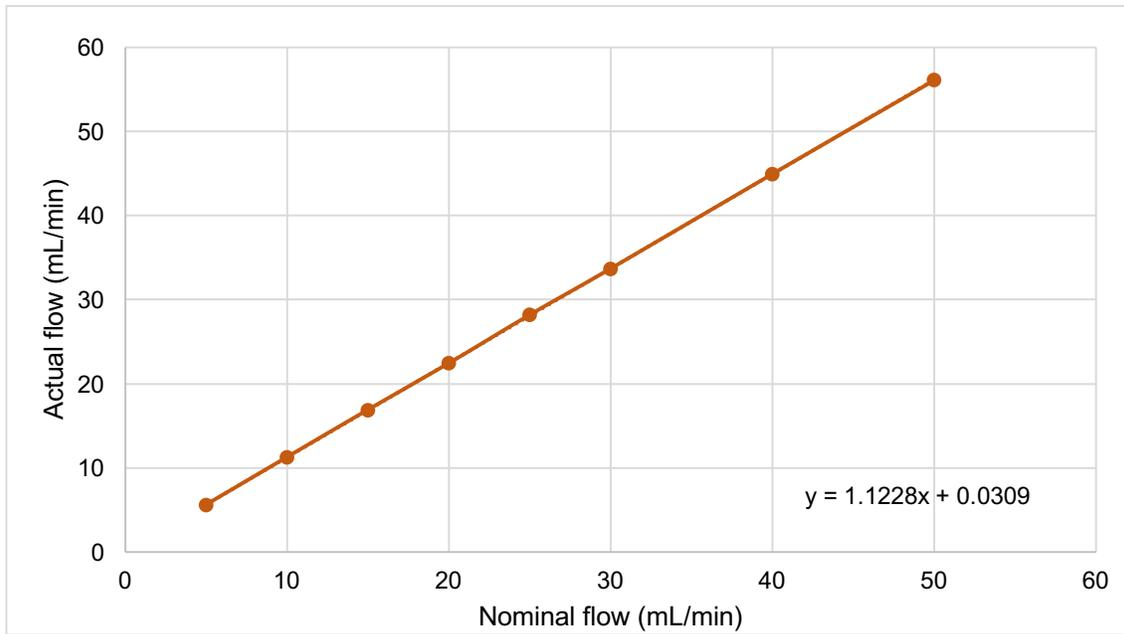
**Figure 5.** Experimentally-determined hydrogen MFC calibration curve
