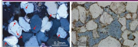
Thin section photo of a typical fluvial sandstone sample, note the extensive quartz overgrowth (red arrows) on the detrital quartz grains. Well 30/24-20z, depth 3126m.  $\phi = 5.2\%$ ;  $K = 0.72\text{mD}$
