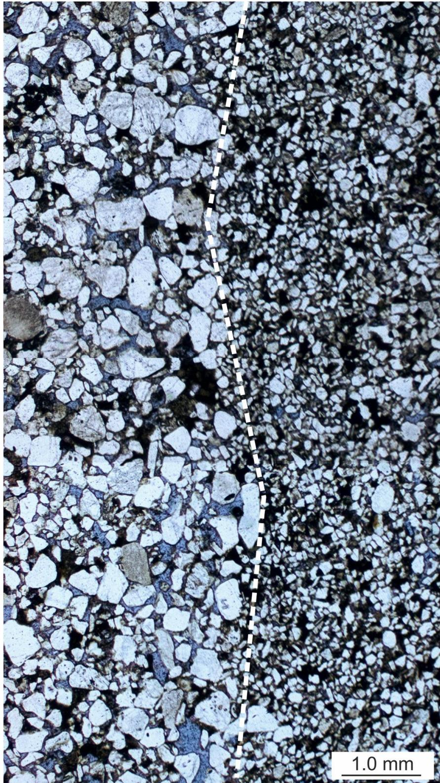
*Figure 5.11 Photomicrograph illustrating different abundance of infiltrated clays in representative pin-stripe lamination dune sandstones. Note the finer grain-size lamination (right) contains more pore-filling clays. Well 30/24-31, 3190.6 m, unit B08, aeolian dune sands.*
