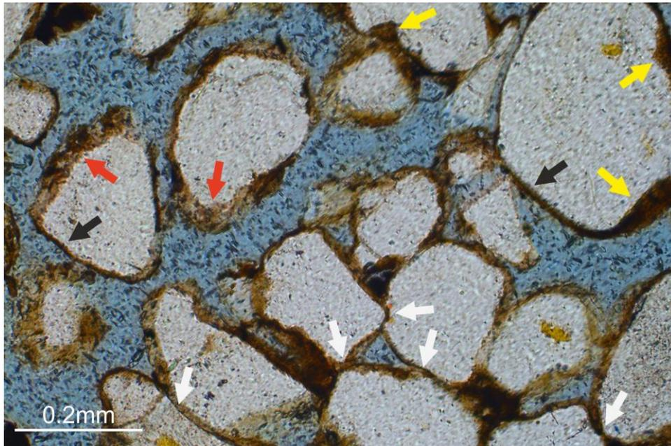
*Figure 5.10 The photomicrograph (plane-polarized light) illustrates the presence of grain coating I/S in the grain contact areas (white arrows), thicker coats in grain surface depressions (yellow arrows) and grain rough surface (red arrows), and thinner coats in non-depression areas (black arrows). Sample from well 30/24-31, 3190.6 m, unit B08, aeolian dune sands.*
