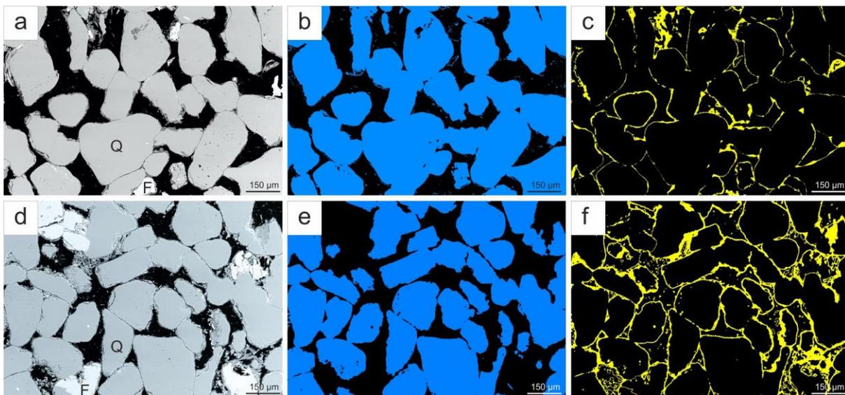
*Figure 5.7 The mineral phases maps for two typical aeolian sandstone samples which contain well-developed and continuous grain coating clays. (a) (b) (c) BSEM image, quartz-facies map and grain coating facies map of sample from Well 30/24-31, 3197.7 m, unit B08, aeolian facies; (d) (e) (f) BSEM image, quartz-facies map and grain coating facies map of sample from Well 30/24-28, 2891.1 m, unit B07, aeolian facies.*
