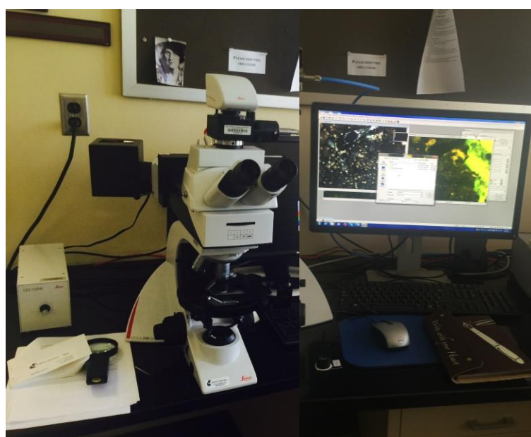
Figure 2-10: A Leica DM 2500P reflected-light microscope equipped with J & M Analytik TIDAS hardware and software
