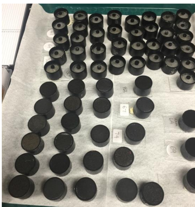
Figure 2-8: Pellets of whole rock and isolated kerogen samples prepared for organic petrographic.
