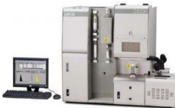
Figure 2-6: LECO C230 Carbon Analyser uses an induction furnace and measures carbon with a non-dispersive infrared (NDIR) detection (image from www.ellingtongeologic.com )
