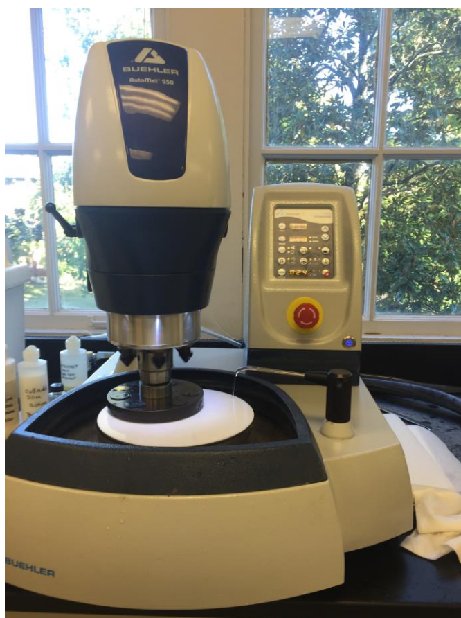
Figure 2-9: The Buehler Automet 250 Micropolish used to ground and polish the cured pellets up to 0.06 \mu\text{m} before microscopic observations.
