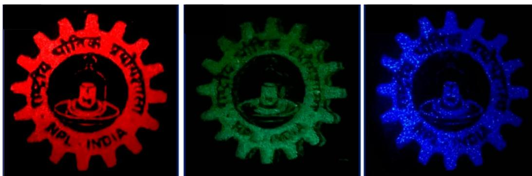
**Figure 1.51** The CSIR-NPL logo printed with  $\text{Eu}^{3+}$ -,  $\text{Tb}^{3+}$ - and  $\text{Ce}^{3+}$ -doped  $\text{Y}_2\text{O}_3$  nanorods, visualised under UV excitation. Adapted with permission from Ref. [125]. Copyright (2017) American Chemical Society.
