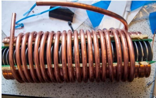
Figure 2.20 Early cooling design using pipework as the in-vacuum reservoir.
