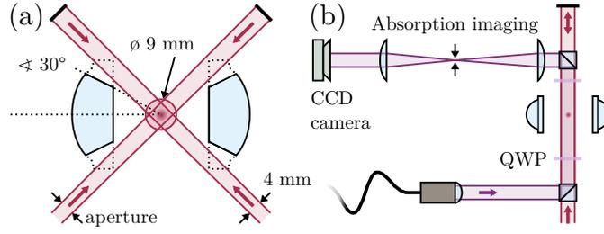
**Figure 3.8:** Realisation of the MOT and constraints imposed by in-vacuo lenses. (a) The in-vacuo lenses are cut at the edges to allow the radial MOT beams to intersect at an angle of  $90^\circ$ . To avoid reflections on the lenses, the radial beam diameter is truncated to 4 mm in the radial plane. (b) Due to limited optical access the axial MOT and an absorption imaging beam are overlapped using polarisation optics.
