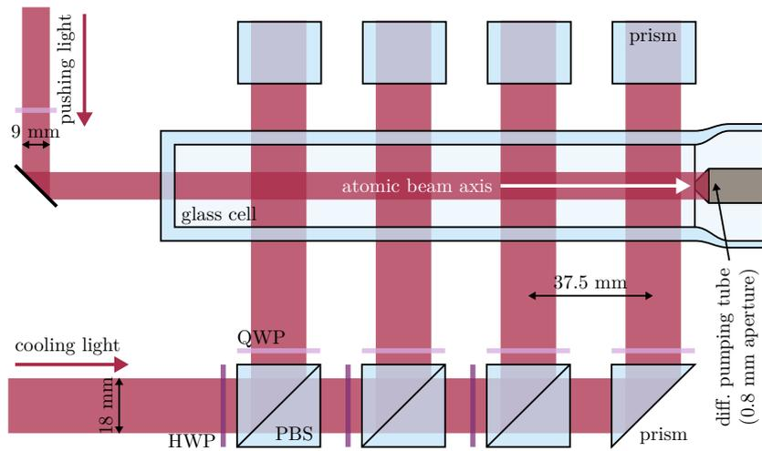
**Figure 3.7:** Optical setup of the 2D MOT. The cooling light is split into consecutive cooling regions using polarisation optics. Another four cooling beams are intersecting perpendicular on the atomic beam axis (not shown as out of the plane of the page). A pushing beam co-propagates along the atomic beam axis to increase atom flux. Both cooling light and pushing beam are circularly polarised and delivered by PM optical fibres.
