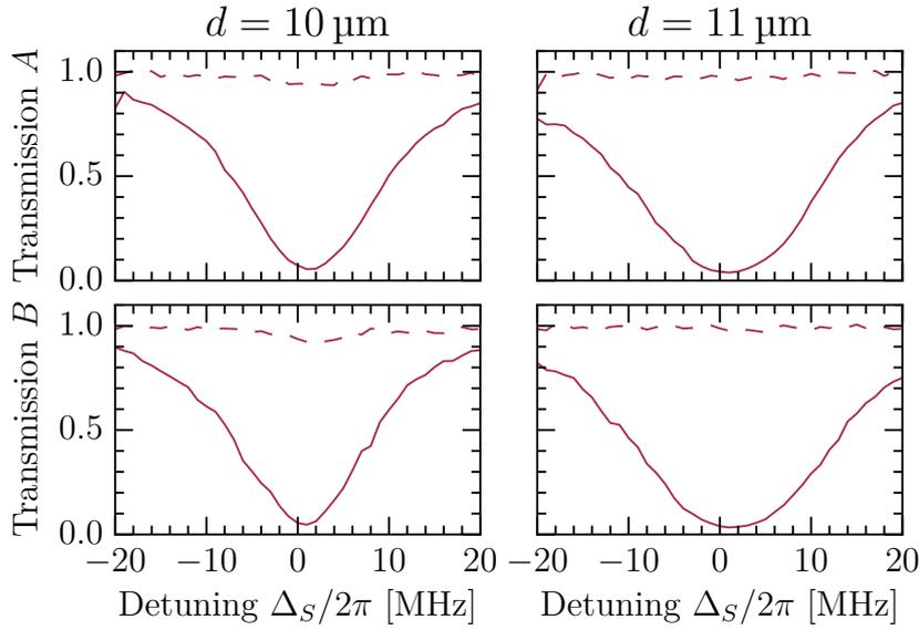
**Figure 5.5:** Cross-talk between photon channels. Transmission of signal light in channels *A* (top) and *B* (bottom) for separations of  $d = 10 \mu\text{m}$  (left) and  $11 \mu\text{m}$  (right). For the spectra shown as solid lines, both atomic media are present. For the dashed spectra, only the medium of the other channel is present. Minimal cross-talk is observed for  $d = 10 \mu\text{m}$ , but absent for  $d \geq 11 \mu\text{m}$ .
