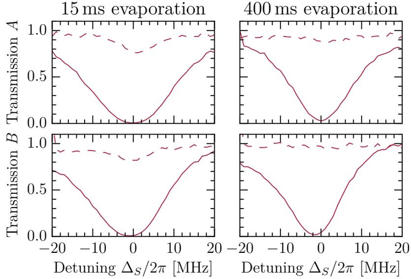
**Figure 3.19:** Effect of evaporative cooling on cross-talk in signal transmission for  $d = 10 \mu\text{m}$ . The solid lines correspond to spectra which are taken when the corresponding medium is present. The dashed spectra are recorded with the medium of the corresponding channel absent.
