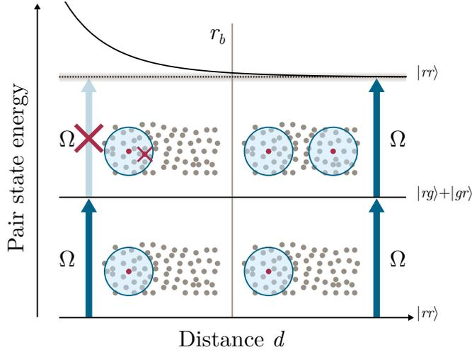
**Figure 2.1:** Dipole blockade between Rydberg atoms. Below a critical distance, the blockade radius  $r_b$ , the dipolar interactions between Rydberg atoms exceed the linewidth of the excitation field  $\Omega$  such that creation of multiple Rydberg excitations within a volume defined by  $r_b$  is prevented.
