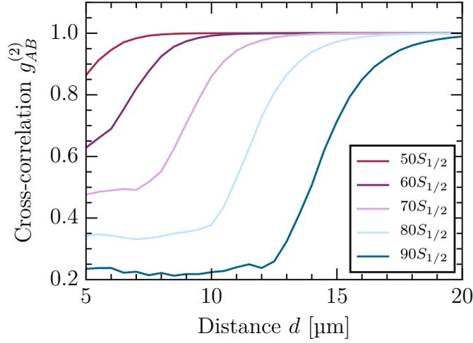
**Figure 5.10:** Simulation results for cross-correlation function for different inter-channel separations  $d$ . Results are shown for different Rydberg states  $|nS_{1/2}\rangle$  with principal quantum numbers  $n = 50$  to  $90$ .
