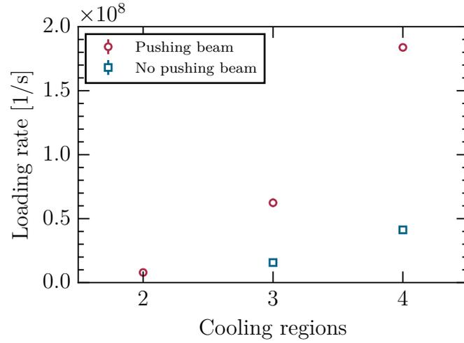
**Figure 3.9:** Influence of 2D MOT cooling volume on MOT loading rate. The loading rate increases substantially with the size of the cooling volume as more cooling regions are unblocked. The addition of a pushing beam copropagating with the atomic beam enhances the performance by a factor of  $\approx 4.5$ .
