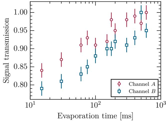
**Figure 3.20:** Cross-talk in resonant signal transmission as function of evaporation time. Scattering of signal light by atoms in the adjacent trap reduces as the ensembles shrink as a result of lower temperatures.
