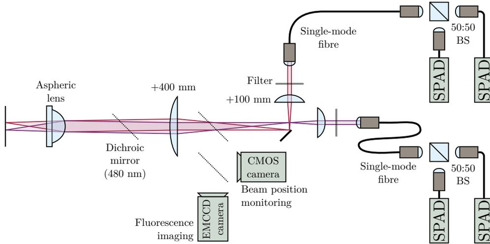
**Figure 3.15:** Single photon detection setup. Both signal modes are separated with an edge mirror at the focus of a 4:1 telescope and coupled into single mode fibres. Behind each fibre two SPADs are arranged in a HBT setup. Using flip mirrors the signal beam foci can be imaged onto a camera to monitor their position during alignment. Similarly, flip mirrors can be used to image the fluorescence of the microscopic cold atom clouds onto a EMCCD camera.
