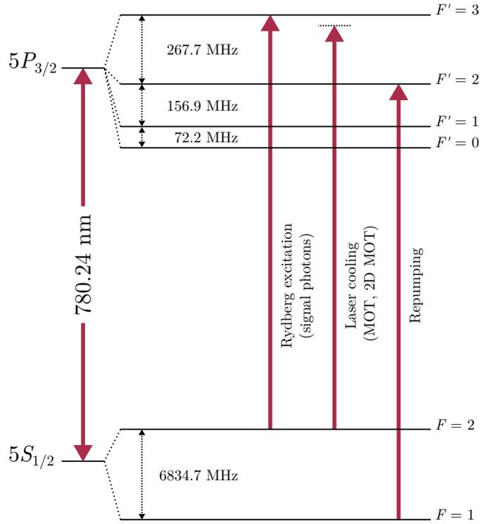
**Figure 3.4:** Level scheme of  $^{87}\text{Rb}$  D2-line and relevant transitions. Laser cooling and repumping for the MOT and 2D MOT occur between the usual  $F = 2 \rightarrow F' = 3$  and  $F = 1 \rightarrow F' = 2$  transitions. The signal light for Rydberg EIT is usually circularly polarised and thus addresses the closed  $F = 2, m_F = \pm 2 \rightarrow F' = 3, m_{F'} = \pm 3$  transition. Data for energy levels taken from D. Steck [215].
