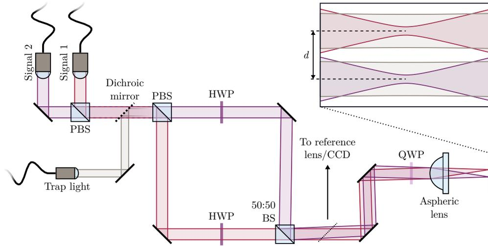
**Figure 3.14:** Optical setup for side-by-side photonic channels. Both signal beams are initially overlapped with the trap light on a dichroic mirror. The two channels are separated in a Mach-Zehnder like setup before recombination on a non-polarising beamsplitter. The channel separation  $d$  can be adjusted by changing the beams' incident angle on the aspheric lens using a mirror in the Mach-Zehnder path of channel  $B$ .
