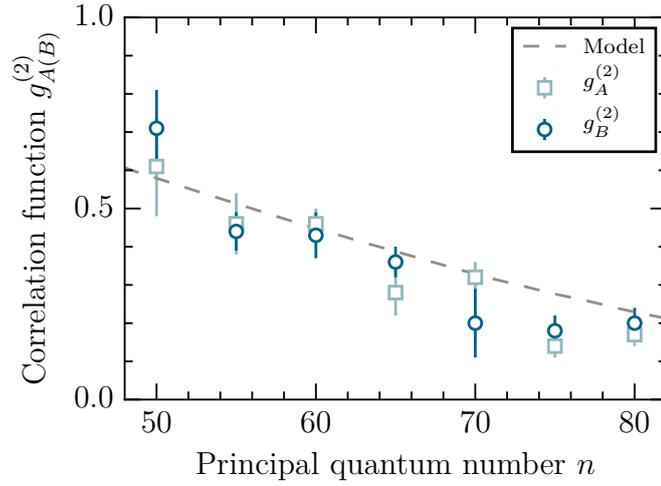
**Figure 4.11:** Photon statistics of retrieved signal light for storage in different  $|r\rangle = |nS_{1/2}\rangle$ . The correlation function  $g_{A(B)}^{(2)}$  is measured independently in two different channels  $A$  and  $B$  following storage for  $t_{st} \approx 170$  ns. The suppression below 1 indicates the retrieval of non-classical light for all  $n$  investigated. The grey dashed line shows the results of the model presented in section 4.3.2.
