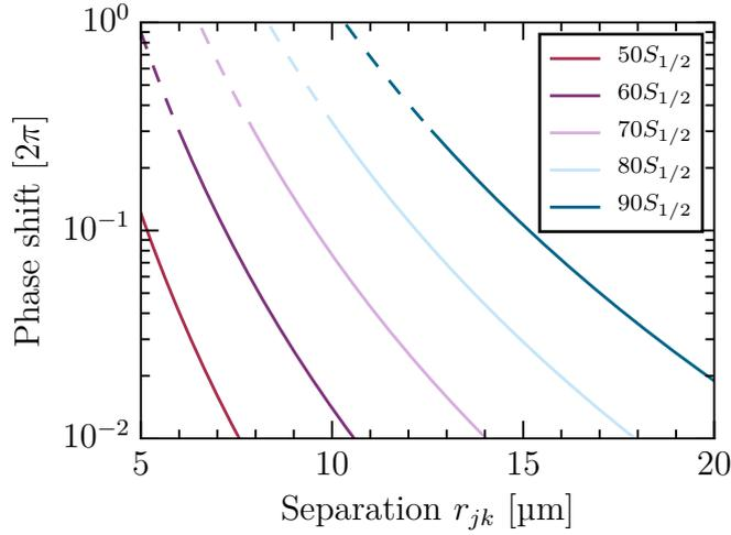
**Figure 5.3:** Interaction induced phase shift between two individual atoms separated by  $r_{jk}$ . VdW-induced phase shifts accumulated per 100 ns interaction time are shown for atom pairs in  $|nS_{1/2}\rangle$ . The dashed lines indicate where  $r_{jk} < r_b^{(6)}(nS_{1/2})$  for a linewidth of 7 MHz.
