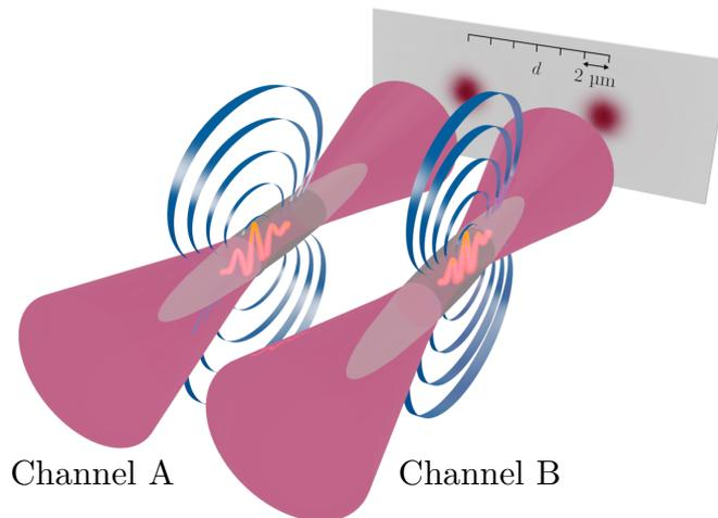
**Figure 5.1:** Implementation of spatially separated, strongly interacting photon channels. Two modes of signal light are tightly focussed into microscopic atomic media where photons are stored as collective Rydberg excitations. During storage the strong dipolar interactions (in this work VdW interactions) between Rydberg atoms are mapped onto the photons.
