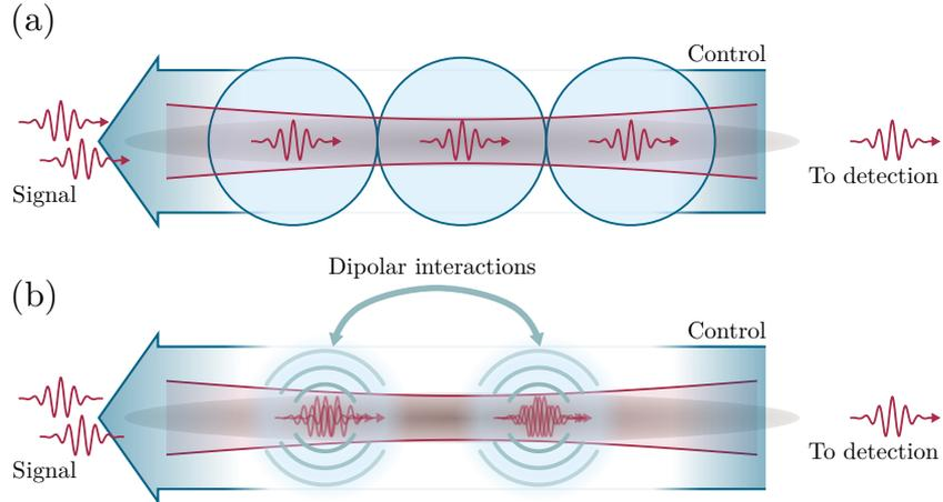
**Figure 2.5:** Effect of Rydberg blockade and interaction-induced dephasing on photon storage. (a) Excitation blockade limits the number of photons that can be stored as stationary collective Rydberg excitations within the blockade volume indicated by the blue circle to one. (b) Dipolar interactions imprint non-uniform phase shifts in the stationary collective excitations which lead to reduced photon retrieval in the original signal modes.
