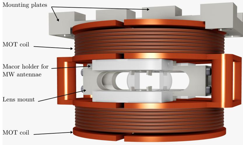
**Figure 3.2:** Overview of the in-vacuo assembly. High NA lenses and a set of electrodes for electric field control are mounted in a central titanium mount and surrounded by a pair of anti-Helmholtz coils for the MOT. Holders for microwave antennae attach to the coils. The entire assembly is connected to the vacuum chamber (not shown) via a titanium mounting plate.
