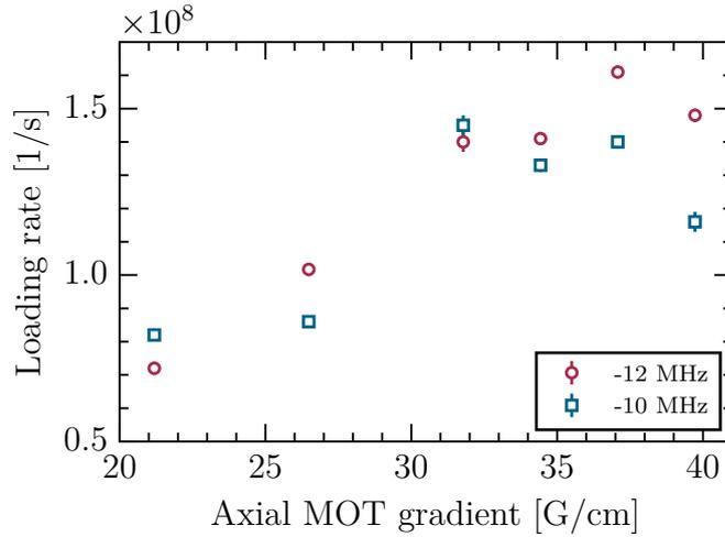
**Figure 3.12:** Influence of MOT magnetic field gradient on MOT loading rate. The loading rate is shown for MOT detunings of  $-10$  and  $-12$  MHz. The values correspond to the axial gradient, the radial field gradient is half.
