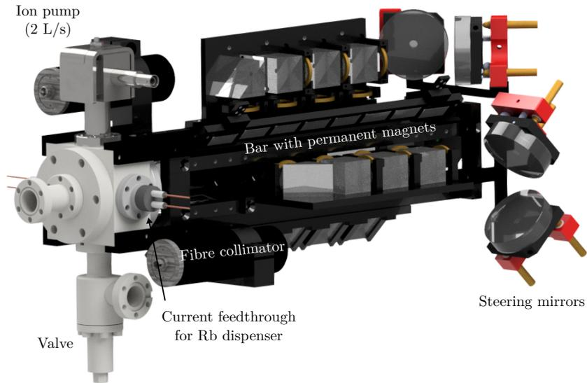
**Figure 3.6:** Overview of the 2D MOT setup. The 2D MOT is realised in a UHV glass cell which attaches to a rectangular block also hosting feedthroughs for the Rb dispensers, an ion pump and a valve for roughing pumps. A cage surrounding the vacuum system mounts the optics for the cooling light and bars with permanent magnets to generate an elongated quadrupole field.
