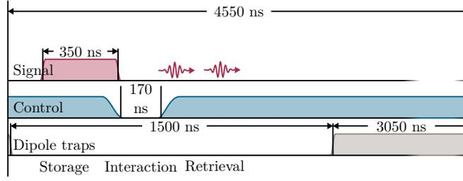
**Figure 4.10:** Experimental sequence to measure photon statistics of retrieved light. The coherent incoming signal pulse has a duration of 350 ns and photons are stored for  $t_{st} \approx 170$  ns while the dipole trap confining the atomic storage medium is switched off. This sequence is repeated 25 000 times before a new medium is prepared in the dipole trap.
