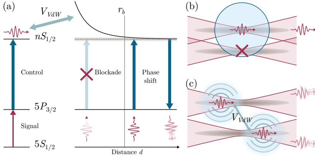
**Figure 5.2:** Effective long-range interactions between photons. (a) Two regimes can be distinguished. For a channel separations  $d < r_b$ , simultaneous storage of photons as collective Rydberg excitations in both channels is prevented (b). For  $d > r_b$ , the atoms contributing to the collective excitation acquire interaction-induced phase shifts which distort the photons' retrieval modes (c).
