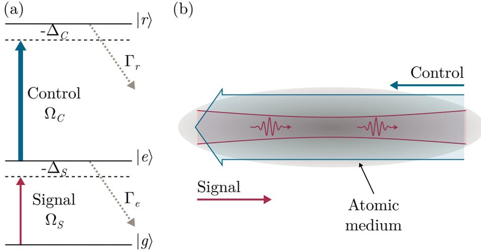
**Figure 2.2:** EIT in a three-level ladder system coupling to a Rydberg state. (a) Overview of relevant states and transitions with detunings and decoherence rates. The optical response of an atomic medium to a signal field coupling a ground state  $|g\rangle$  to an intermediate state  $|e\rangle$  can be controlled by a stronger control field coupling  $|e\rangle$  to a Rydberg state  $|r\rangle$ . (b) Example of a typical implementation of EIT in a cold atomic ensemble.
