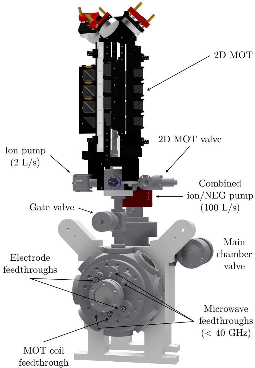
**Figure 3.1:** Overview of the vacuum system. The main science chamber is on the bottom, below the 2D MOT which is mounted vertically. A gate valve allows separation of both vacuum sections. Various electrical and microwave feedthroughs are attached to a cluster flange. Behind the main chamber a pumping section hosts a combined ion/NEG pump and a valve to connect further pumps during bakeout.
