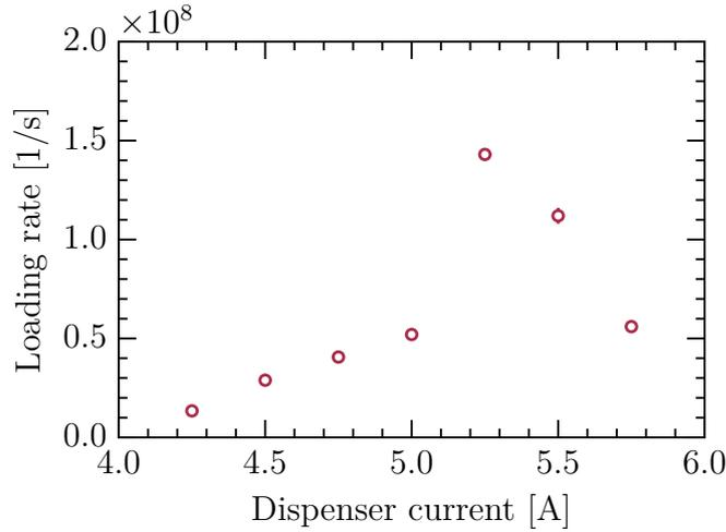
**Figure 3.10:** Influence of Rb partial pressure in 2D MOT on MOT loading rate. As the actual pressure cannot be directly measured, the loading rate is shown as a function of the current applied to heat the Rb dispensers.
