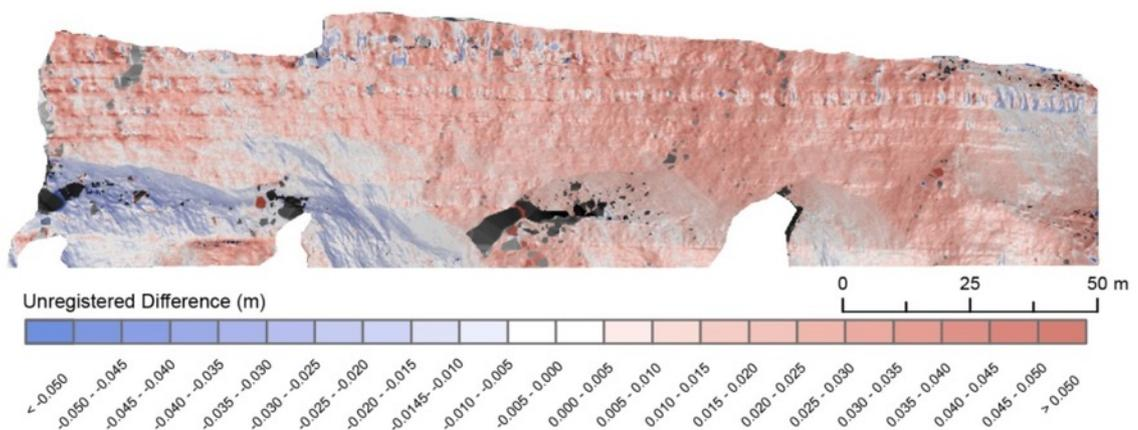
**Figure 4.9:** Change between two stable scans that are unregistered. While the scanner is securely installed, small variations in its orientation propagate the offset in measured point positions at targets distances from 350 m – 550 m. Regions of positive and negative change can be observed on surfaces that are inclined towards and away from the scanner position, indicating that a small rotation of the scanner may have occurred.
