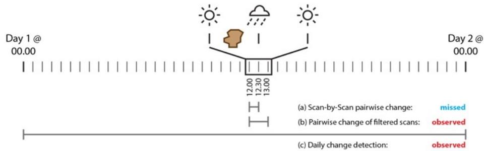
**Figure 4.36:** Conceptual illustration of the significance of removing partial scans. While parts of these scans provide accurate estimates of surface change, if a rockfall occurs in an area of no data, the failure will be missed using pairwise change. These scans must therefore be removed prior to change detection of the scan database.
