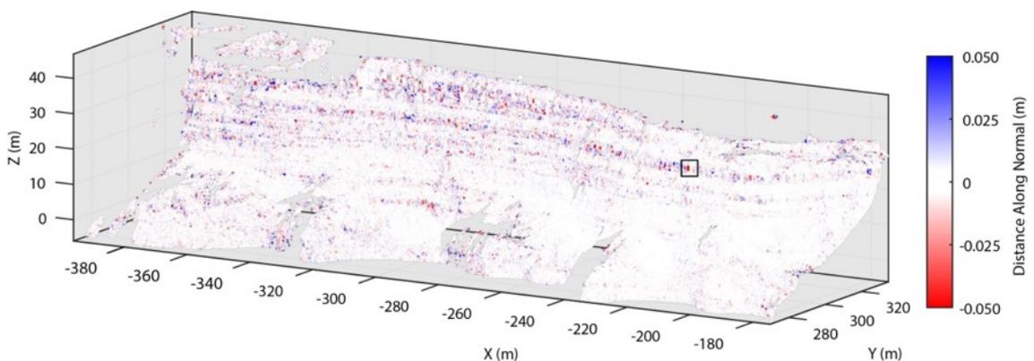
**Figure 4.27:** Distance along the normal between two scans. Edges present a significant uncertainty even after the filtering process. The black box indicates the example area used in subsequent figures.
