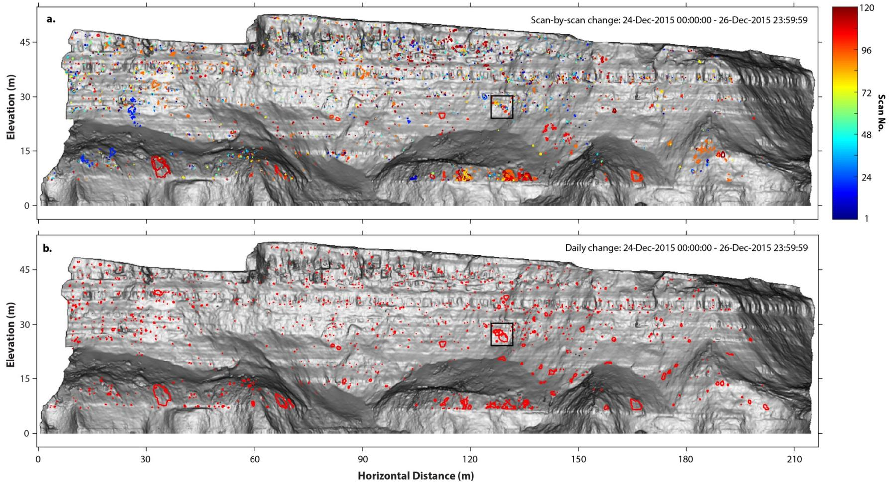
**Figure 4.34:** (a) Rockfall derived from pairwise change detection of 120 scans. This fails to detect many of the individual rockfall events that occurred within the square box, including a  $4.9979 \text{ m}^3$  event. This is caused by the omission of this area of cliff within partial-scans due to rainfall. (b) Rockfall derived from daily change detections over the same storm period.
