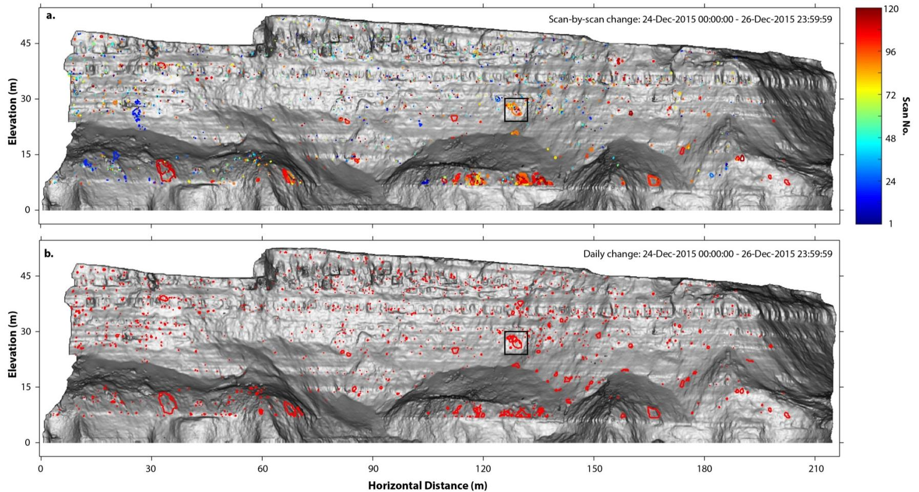
**Figure 4.35:** (a) Rockfall derived from pairwise change detection of a scan database that includes only point clouds with entire cliff coverage. This includes numerous small rockfall within the square box that are depicted as a single event in the daily change images. (b) Rockfall derived from daily change detections over the same storm period.
