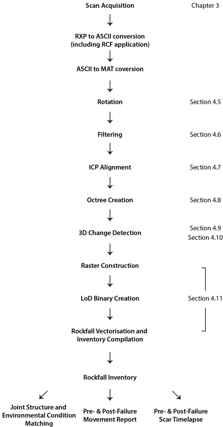
*Figure 4.1: Flow diagram representing each phase of the rockfall inventory compilation. All stages following ASCII to MAT conversion were written in MATLAB. ICP alignment used the pcregrid function, and rockfall vectorisation used the bwboundaries function.*
