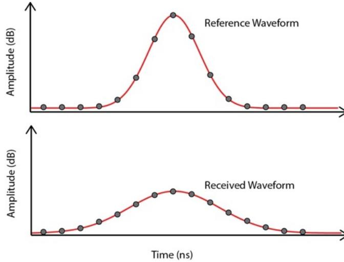
**Figure 4.4:** Comparison of the reference waveform structure to the received waveform, with each measurement separated by ca. 2 ns. High target incidence angles relative to the beam incidence angle can spread and skew the distribution of the received waveform. Increased target range also attenuates the returned signal. If multiple discontinuities are intersected within a single line-of-sight, multiple peaks are created. Deviations of zero indicate identical waveform structures.
