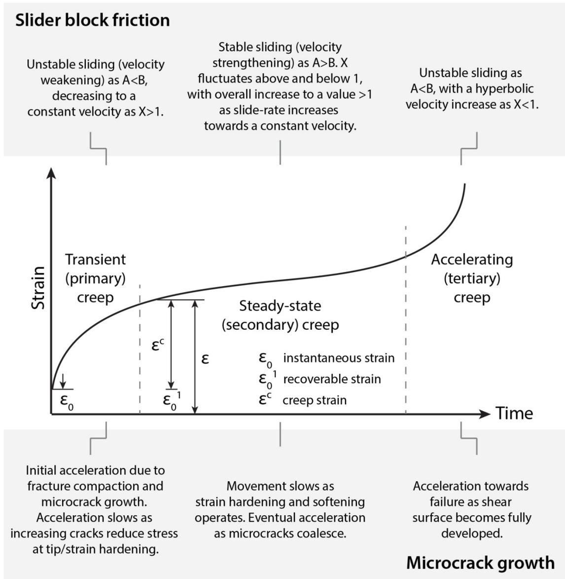
**Figure 2.2:** Schematic plot of the time-dependent strain component on a rock sample, exhibiting three phases of movement known as transient, steady-state and accelerating. Parameters  $A$ ,  $B$  and  $X$  of the slider block friction model account for observed variation (top). Microcrack growth (bottom) in conjunction with strain hardening and softening is also displayed.
