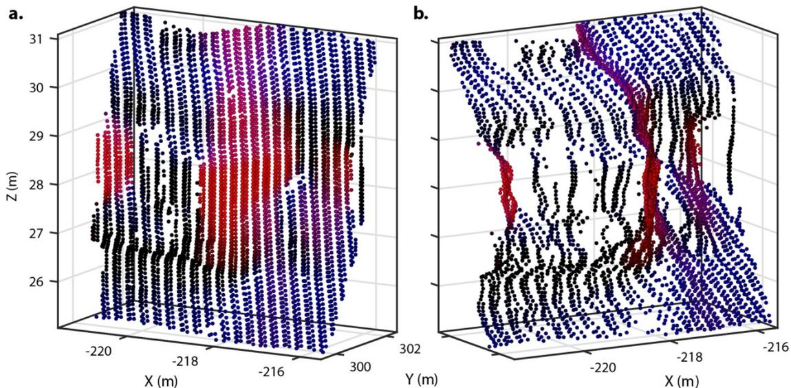
**Figure 4.28:** (a) Subset of bedded sandstone, coloured by the surface normal. Red points define planes orthogonal to the scanning direction. (b) When rotated away from the scanning direction, points that are incoherent within and between scans, and averaged between surfaces, become evident.
