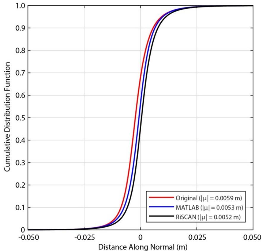
**Figure 4.14:** Cumulative distribution of the change for the unregistered point clouds, MATLAB aligned and RiSCAN PRO MSA aligned. While the mean offset in the unregistered point cloud data is 0.0059 m, this is reduced to similar levels using with ICP using both MATLAB and RiSCAN PRO.
