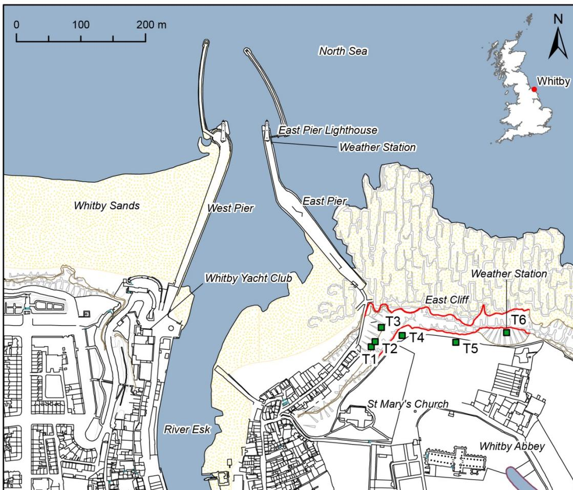
**Figure 3.1:** Map of Whitby with the area scanned delineated with red lines. The Riegl VZ-1000 scanner used in this study is installed within East Pier Lighthouse, located at the end of East Pier. The targets installed for the SiteMonitor4D system, in addition to the weather stations, are illustrated (T1 – T6). Whitby Abbey lies 180 m from the cliff top. Map produced using shapefiles from Ordnance Survey © Crown Copyright and Database Right 2016. Ordnance Survey (Digimap Licence).
