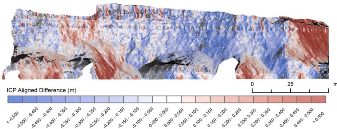
**Figure 4.10:** Change between two stable scans that are registered using ICP to minimise the point-to-point distance. Here, no downsampling is applied to either point cloud. As such, inconsistencies in the point distribution between scans compromise the accuracy of the alignment procedure. The colour scheme here is the same as that applied in Figure 4.9; point-to-point ICP therefore exacerbates the small offset in the position of the scans around the vertical axis.
