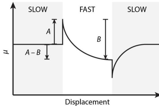
**Figure 2.1:** Experimentally observed frictional response to an exponential increase in sliding velocity, followed by an exponential decrease in sliding velocity. During the initial velocity increase, a direct increase in friction ( $A$ ) occurs, known as the direct velocity effect. An evolutionary decrease in friction ( $B$ ) then occurs. Adapted from Scholz (1998:37).
