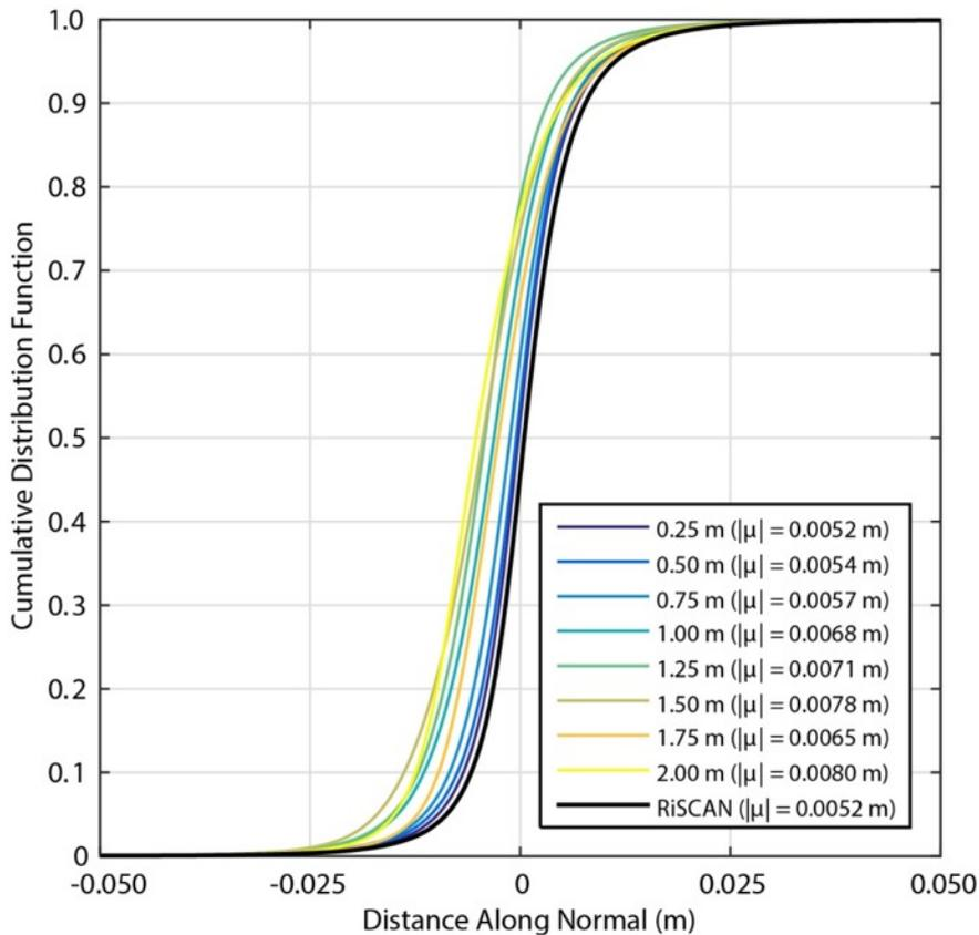
**Figure 4.13:** Cumulative distribution of the change for every point between two scans aligned using ICP (point-to-plane). Each coloured line represents a different scale of downsampling. A downsampling of 0.25 m produces the same mean absolute error ( $\mu$ ) value 0.005 m as MSA through RiSCAN PRO.
