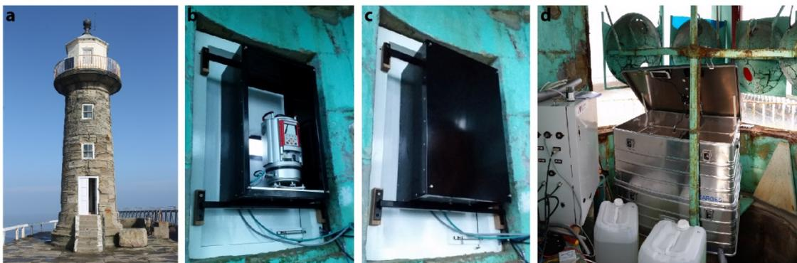
**Figure 3.8:** (a) Image of East Pier Lighthouse at the end of East Pier before the installation took place. This side of the lighthouse faces towards the cliff, (b-c) A Riegl VZ-1000 is mounted within an aluminium frame with a secure removable panel at the back. The scanner measures the cliff through a glass panel suited to allowing the laser to pass through with minimal interference, and (d) Two batteries are used to power the system, charged by methanol fuel cells.
