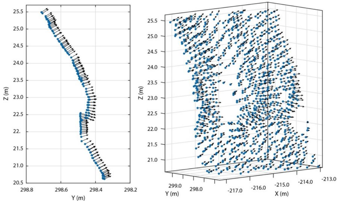
**Figure 4.20:** An example of the normal vectors estimated for at an interbedded sandstone protrusion 20 m up the cliff face. Normal estimation is robust to variations in the density and distribution of points within this area.
