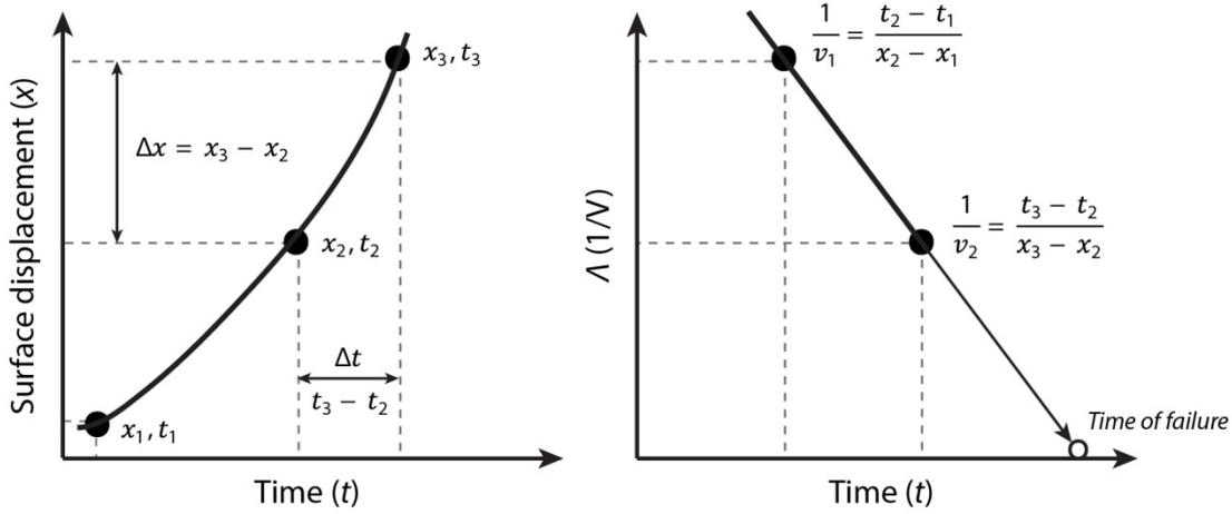
**Figure 2.4:** Left. Hyperbolic acceleration of surface displacements prior to failure. Here velocity is measured using the displacement at each measurement interval. Right: For the same displacement, the reciprocal of velocity,  $\Lambda$ , also termed ‘Inverse Velocity’ is shown. Extrapolating to the point where  $1/V$  is approximately zero provides an estimate of failure time.
