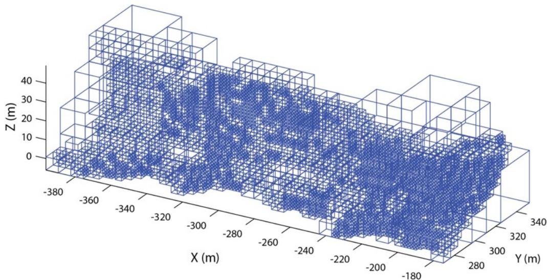
**Figure 4.16:** Octree structure created for the first scan of East Cliff. This structure is a reference to which subsequent point clouds are assigned. Unlike voxels, this approach to segmentation is robust to variations in point density across the cliff face. Since no major alteration to the topographic structure of the rock face occurred, all points in subsequent point clouds were assigned to this same structure.
