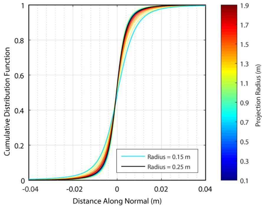
**Figure 4.24:** Cumulative distribution function of change between two point clouds, between which no observable change occurred. As such, the distribution of points should be as close to 0 m change as possible. Each line represents a different cylinder radius that is used. 0.15 m exhibits the highest deviation away from change values close to zero.
