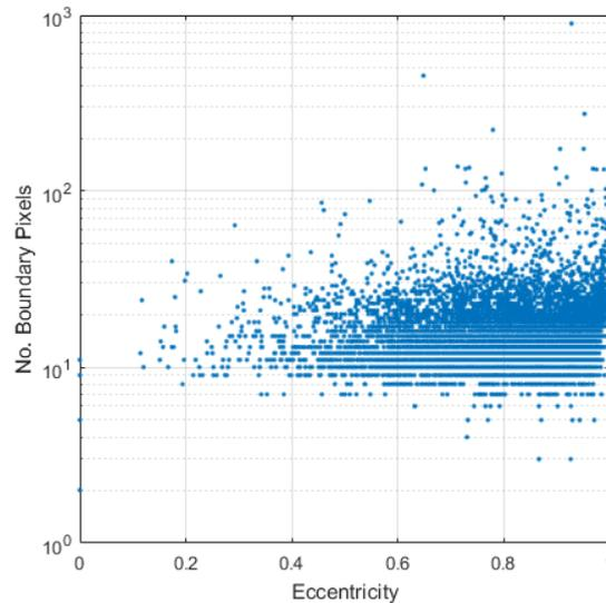
**Figure 4.33:** Eccentricity of failures measured against the number of boundary pixels. A higher ratio of boundary cells relative to the total number of cells in the failure (eccentricity) results in a greater volumetric uncertainty.
