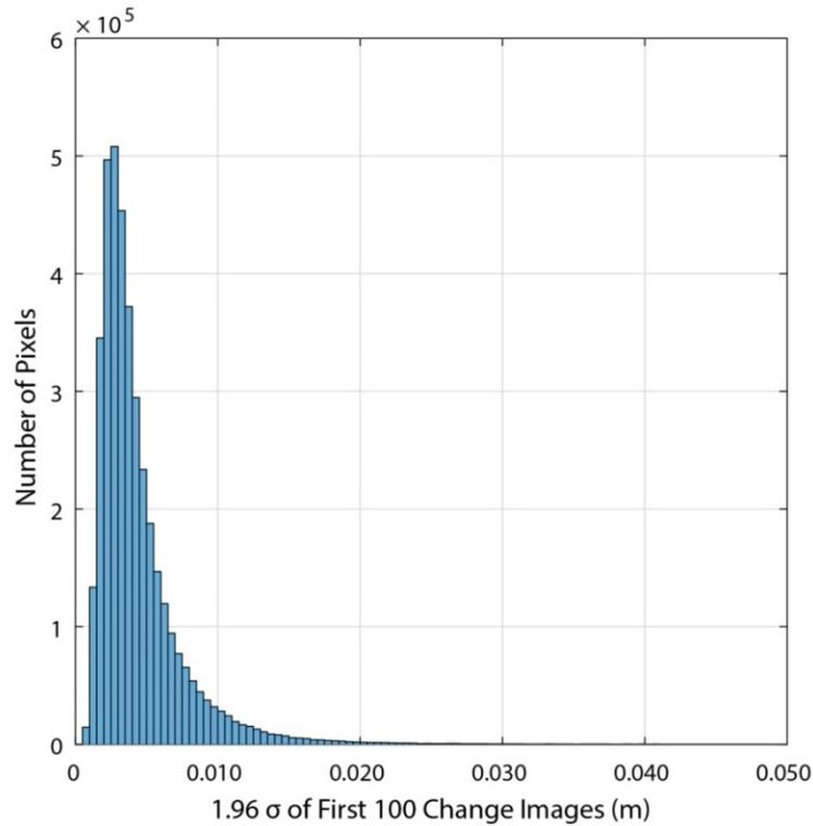
**Figure 5.1:**  $1.96 \sigma$  of the first 100 change rasters (0.0005 m bin widths). These values fall below the 0.03 m LoD used to mask rockfall. This shows that the accuracy of the 3D change detection techniques, developed in Chapter 4, is not reduced though interpolation.
