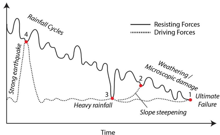
**Figure 2.6:** Conceptual figure showing the timescales and roles played by preparatory and triggering factors in landslide evolution. Red dots indicate when progressive failure can occur due to the equalisation of driving and resisting forces. Modified from Gunzburger *et al.* (2005, Figure 2) and Gischig (2011, Figure 1.1).
