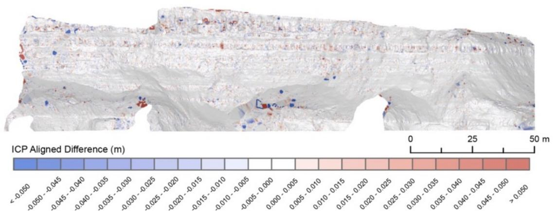
**Figure 4.12:** Change between two stable scans that are registered using ICP to minimise the point-to-plane distance. Here, 0.25 m downsampling was applied. The dependence of alignment accuracy on surface orientation exhibited in Figure 4.10 and Figure 4.11 is removed. The colour scale here is the same as that applied in Figure 4.10.
