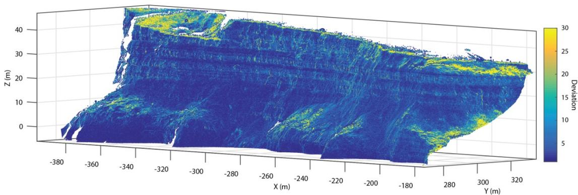
**Figure 4.5:** Distribution of deviation values across the cliff face. The highest values coincide with the presence of multiple surfaces within a single line of sight, in particular at the near-horizontally bedded sandstone protrusions and vegetation. While deviation increases with target range, this effect is small relative to the incidence angle.
