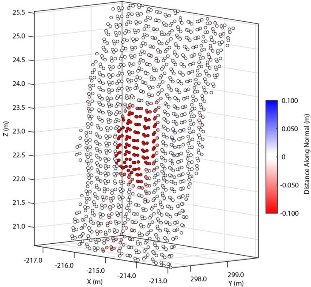
*Figure 4.30: An example of a rockfall calculated using the distance along the normal.*
