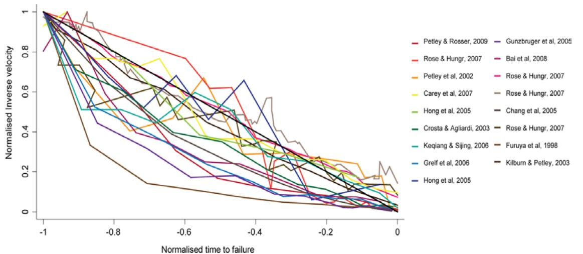
**Figure 2.5:** Comparison of published pre-failure deformation data. Normalised time and inverse-velocity values allow direct comparison between sites. The solid black line represents a perfectly linear trend in  $A$ - $t$ , expected in first-time brittle failures. Asymptotic trends characterise ductile failure, or failure along existing sliding surfaces. Source: Froude (2011:121).
