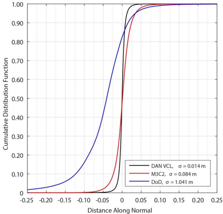
**Figure 4.31:** Cumulative distribution function for the change detections of multiple pairs of stable scans, such that the theoretical distribution of distance along normal values should be zero. The methods used are DEMs of Difference (DOD; blue line), M3C2 (red line) and Distance Along the Normal, Variable Cylinder Length (DAN VCL; black line).
