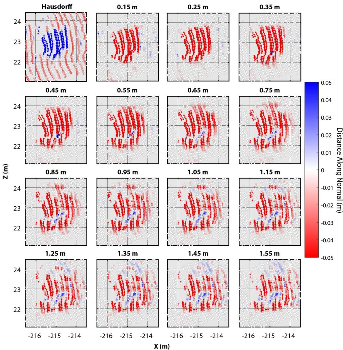
**Figure 4.26:** Distance along the normal approximated using a variety of cylinder radii from 0.15 – 1.55 m. These are compared to an unsigned Hausdorff distance in the top-left. As the cylinder radius increases, the rockfall scar expands by averaging change across a wider area. This also has the effect of introducing forward movement (blue) into the rockfall scar.
