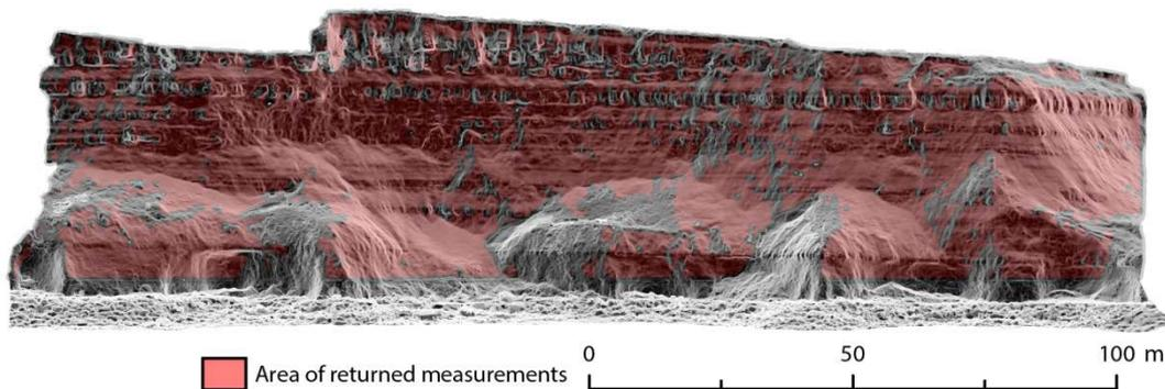
**Figure 3.11:** Area scanned by the permanent monitoring system used in this study (red) draped over a complete slope model of the entire cliff captured from multiple positions along the foreshore. The total area measured is 8 561 m<sup>2</sup>, 89% of the cliff face total (9 592 m<sup>2</sup>).
