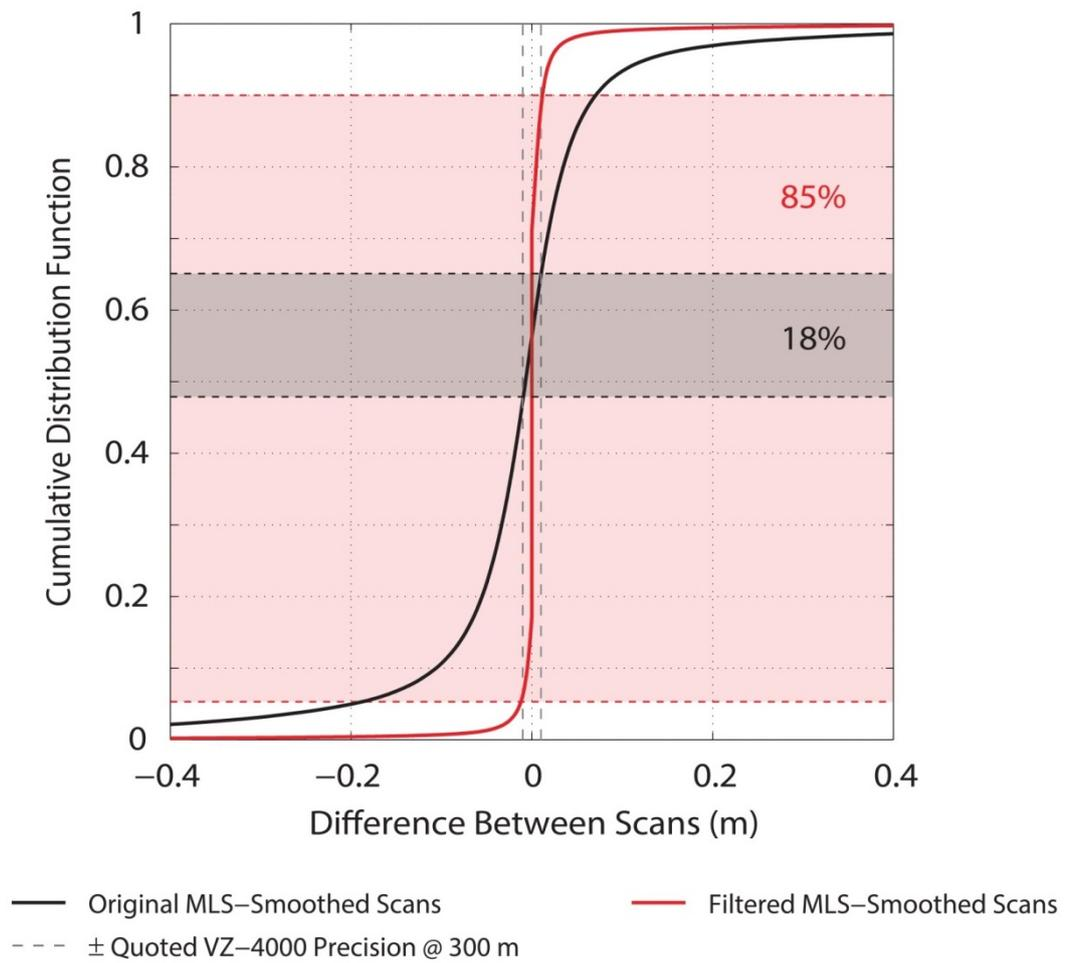
**Figure A.E.6:** Change detection between two scans of an open-pit high wall, between which no change occurred. Here, 3D MLS shows an improvement in precision, such that 85% of the point clouds fall within Riegl's quoted precision under test conditions at the minimum target range (300 m). This is increased from 18% using the raw point cloud data.
