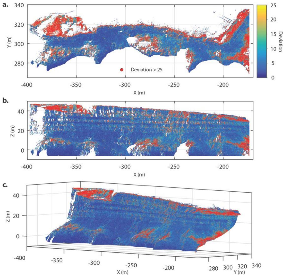
**Figure 4.8:** Deviation across the cliff with values  $> 25$  coloured red and removed from each point cloud prior to change detection. (a) Aerial perspective showing the sensitivity of vegetation at the cliff top and on top of the buttress to deviation. (b)  $x$ - $z$  plane directly viewing the cliff. Holes in the point cloud are now apparent, with their edges delineated in red. (c) View from the angle of scanning.
