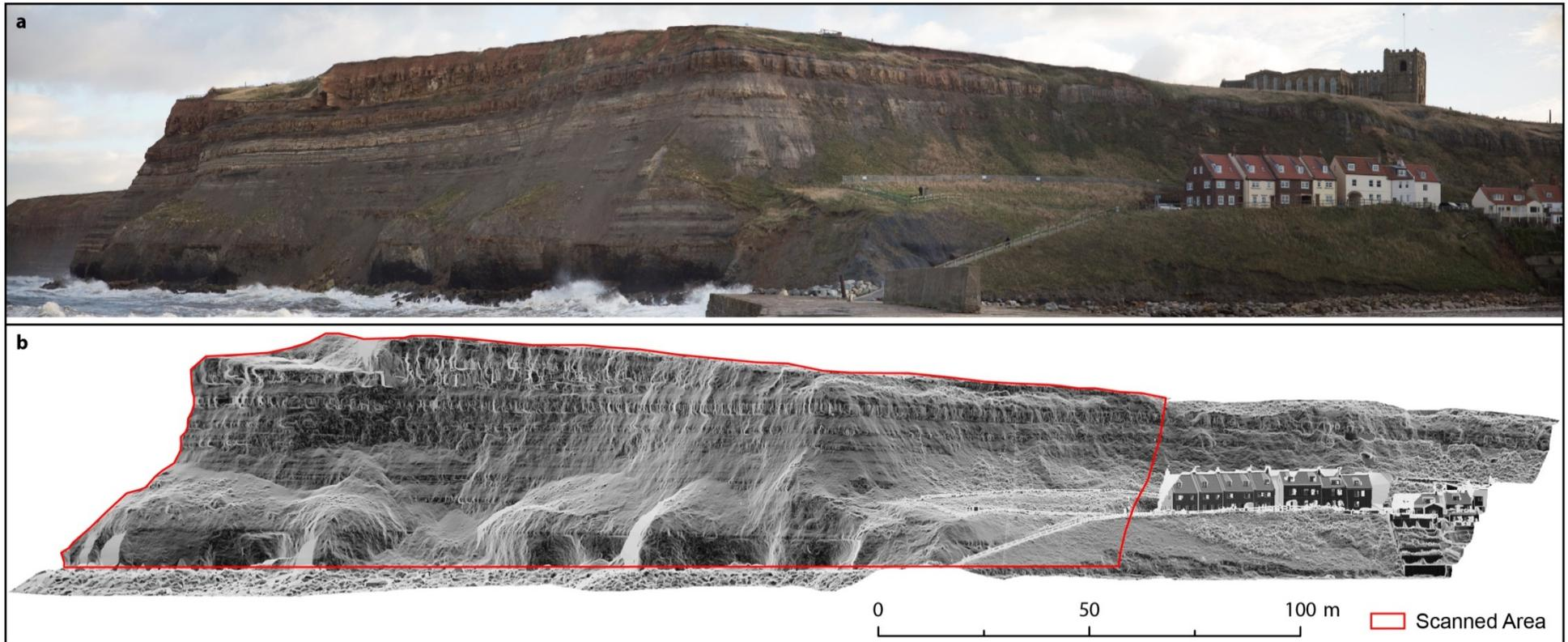
**Figure 3.10:** (a) Panorama photo taken at high tide, 5.7 m. East Cliff is left-of-centre, with targets positioned along the rockfall protection barrier right-of-centre. St. Mary's Church is also visible. (b) 0.10 m slope model acquired from the lighthouse in February 2015. Red line denotes scanned area during monitoring campaign.
