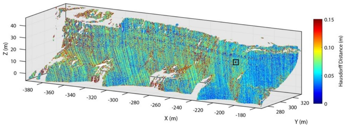
**Figure 4.25:** Hausdorff distance estimation between two point clouds where a rockfall occurred. This metric yields change between scan lines, highlighted by the striping effect, and change that is sensitive to point density, highlighted by the distance decay from left (distal) to right (proximal). However, this provides an accurate measure of the scar shape that is useful for refining the parameters used in the change detection in this research.
