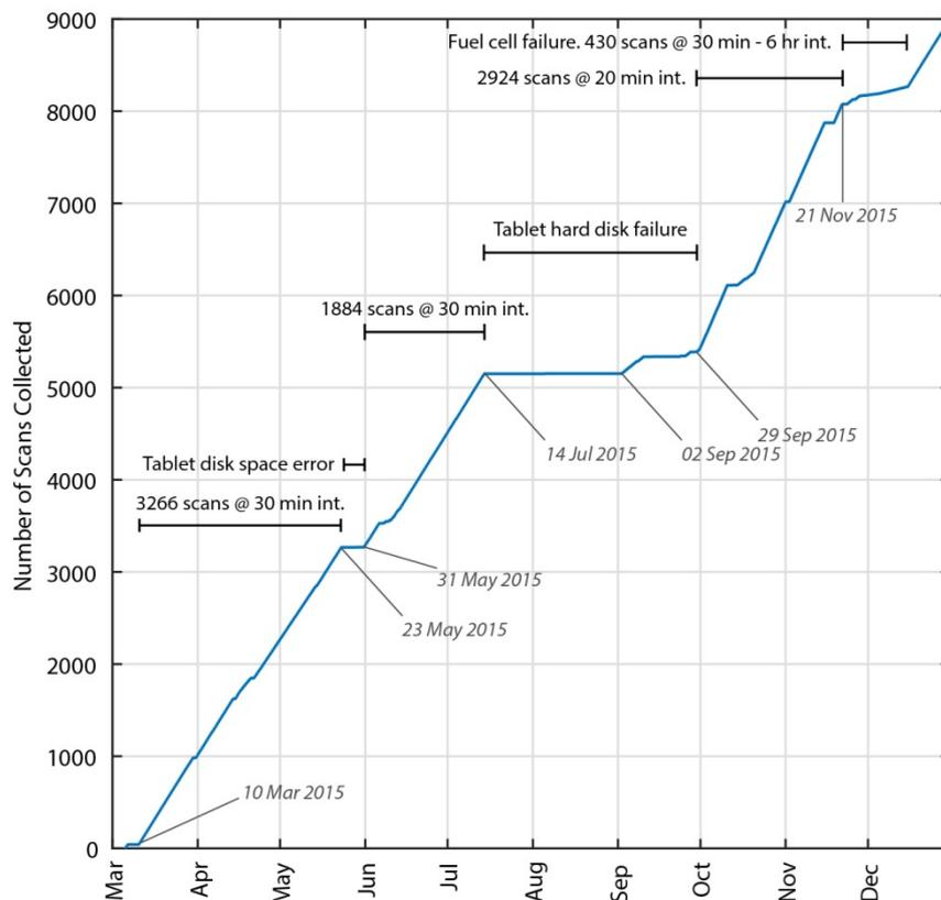
**Figure 3.12:** Cumulative number of scans collected between 5<sup>th</sup> March 2015 and 30<sup>th</sup> December 2015. The gradient of the line reflects the acquisition rate, either 20 minutes or 30 minutes. Breaks in the gradient reflect system maintenance difficulties discussed in *Section 3.10*.
