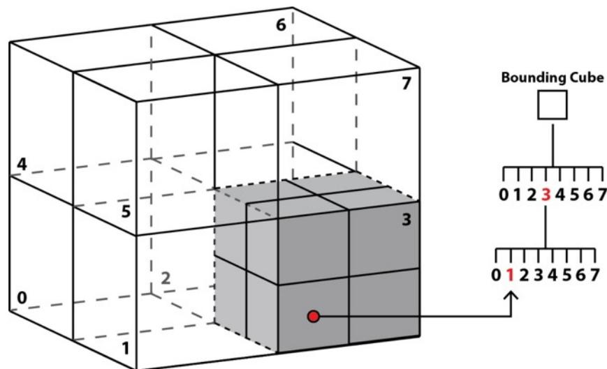
**Figure 4.15:** Principle of octree subdivision, where the location of a point within the cloud (red) is identified by an  $m \times 8$ -bit code, where  $m$  is the number of subdivisions. Here, there are two subdivisions, which generate a  $2 \times 8$  identifier for the point. Adapted from Figure 2 in Girardeau-Montaut (2005).
