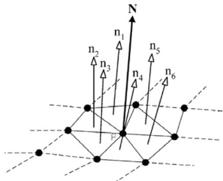
**Figure 4.19:** Normal estimation by averaging the normal directions of six triangles that surround the query point (centre). This method is optimised for scans with very low point spacing and uniform scan line spacing.
