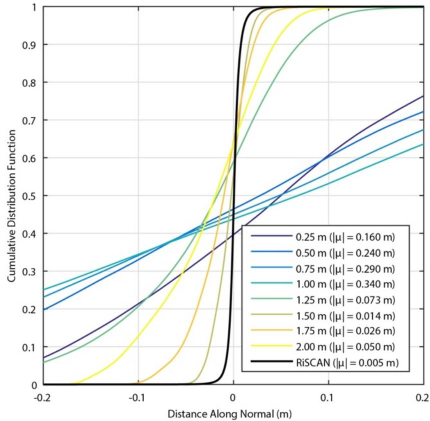
**Figure 4.11:** Cumulative distribution of the change for each point between two scans aligned using ICP (point-to-point). Since no observable change occurred between the scans, the distribution should approach zero across the point cloud. MSA using RiSCAN PRO (black) produces a mean absolute distance ( $\mu$ ) of 0.005 m, significantly lower than point-to-point ICP. An increase in the spacing of the downsampled point clouds benefits the alignment.
