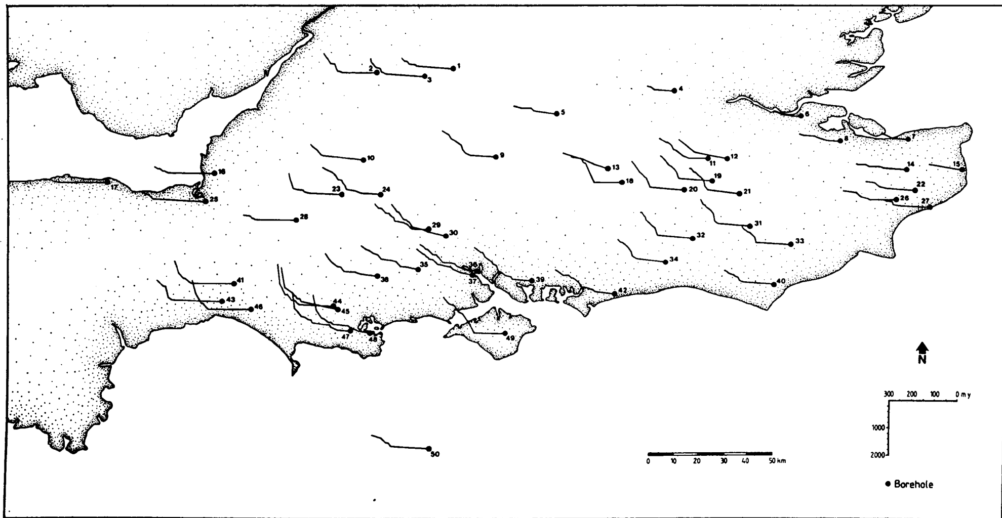
Fig. 2.16 Subsidence plots for all the backstripped boreholes in southern England. Borehole numbers are summarized on Table 2.1.
