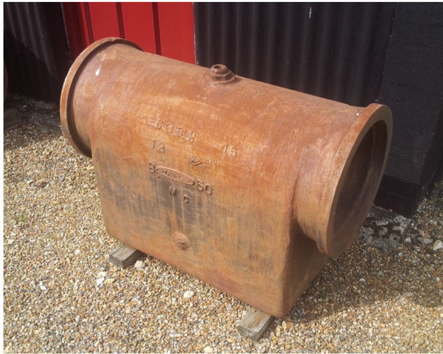
Figure 12 - Photograph of a water trap used for separating water from town gas (Fakenham Gas Museum, 2014)
