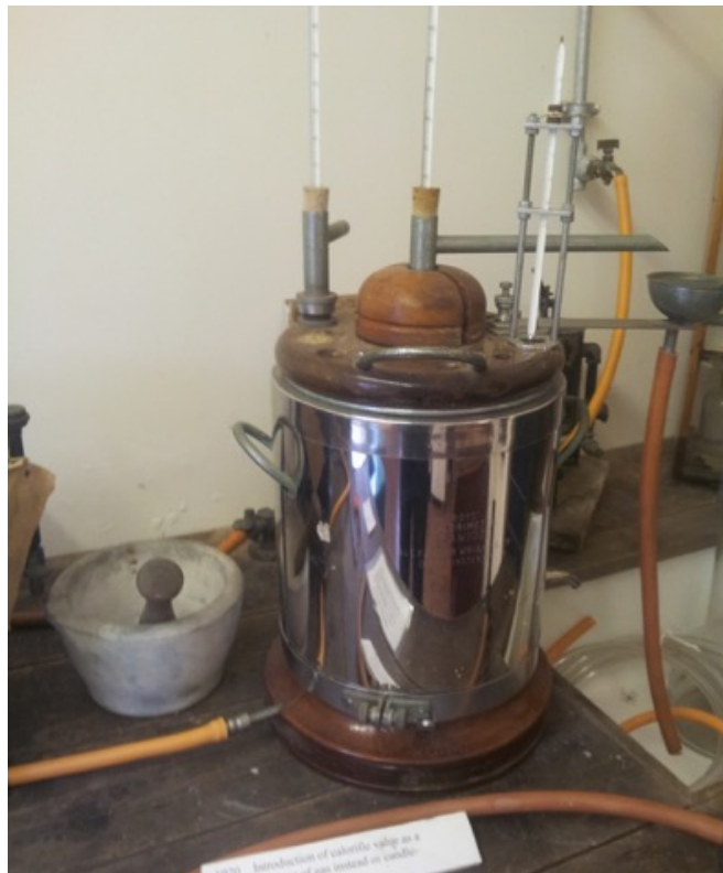
Figure 8 - Photograph of a town gas 'calorimeter' (Fakenham Gas Museum, 2014)
