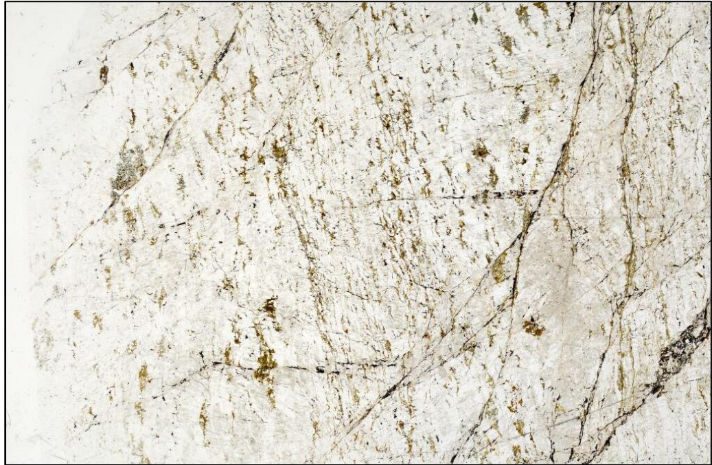
Figure 405. Mylonite (S73582) thin section under PPL. Contains British Geological Survey materials © NERC 2016. No scale available
