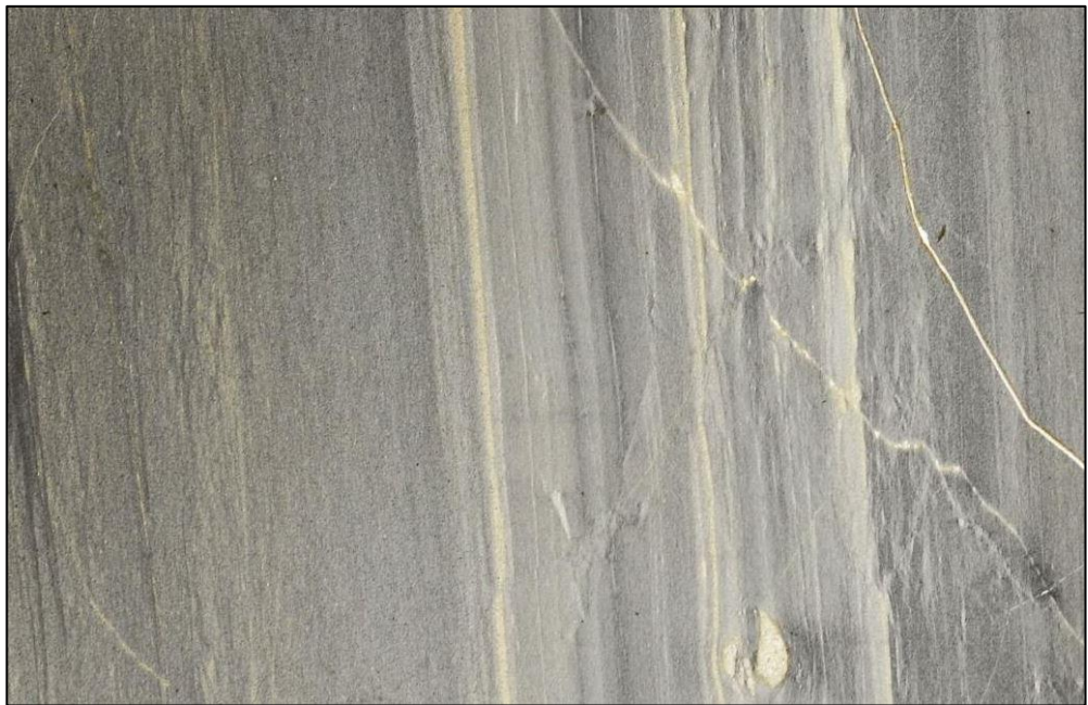
Figure 407. Baked shale (S72034) thin section under PPL. Contains British Geological Survey materials © NERC 2016. No scale available
