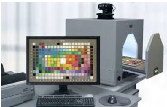
Figure 38 Example of calibration procedure with DigiEye, image taken from manufactureswebsite 87
