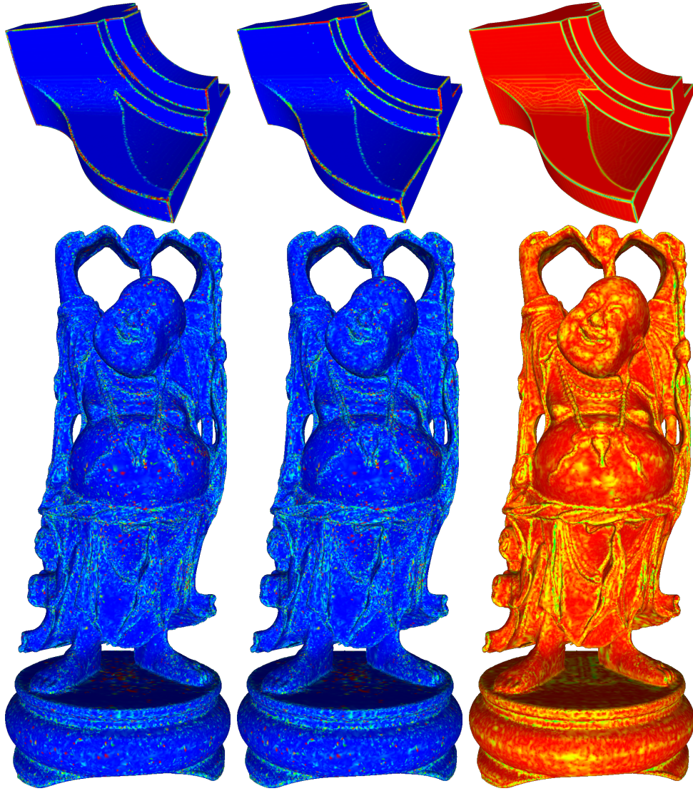
Fig. 7.9: Comparison of real meshes (left) to their smooth counterparts (center), Metro comparisons (right).
