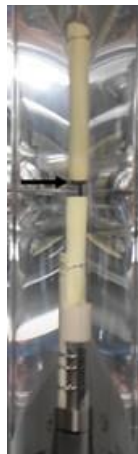
Figure 7.6: Tip of feed rod darkened with a graphite pencil to minimise the disparity in levels of heat absorption of sintered and molten \text{Bi}_{0.8}\text{V}_{0.2}\text{O}_{1.7} .
