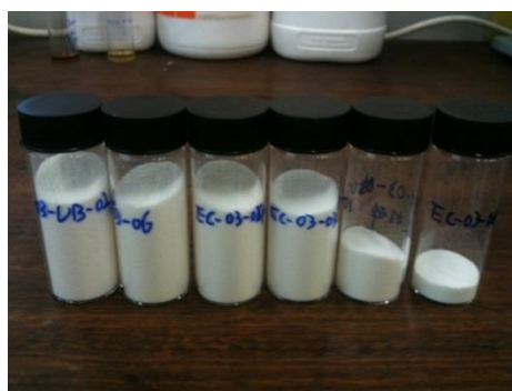
Figure 4.1: Micro-capsules containing different healing agents
