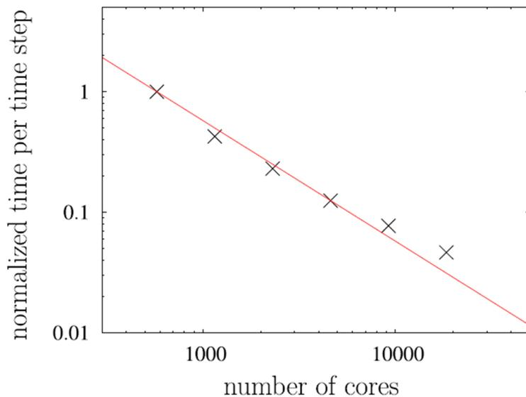
Figure 1.6: Strong scaling is observed for GENE on Hector [24], but as the number of cores exceeds 10000, the scaling weakens. The red line shows a linear scaling with the number of cores.
