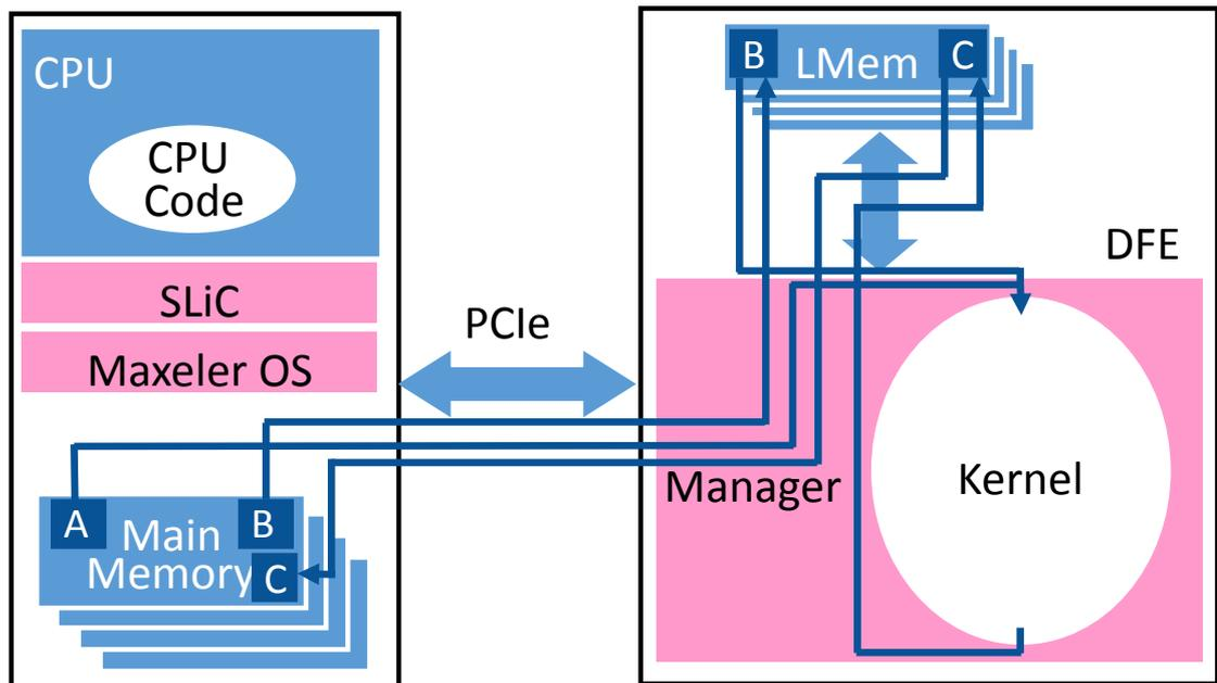
Figure 5.2: Schematic showing the data movement of the matrices A, B and result C between the CPU, DFE LMem and kernel.
