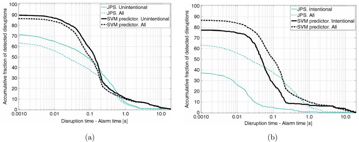
Figure 1.15: Warning times (disruption time minus alarm time) for all the disruptive pulses from JET campaign C1 till campaign C19; (a) the cumulative percentages of unintentional and all detected disruptions for the FPGA SVM method are compared with the JET JPS alarm results, (b) the cumulative percentages of intentional and all detected disruptions for the FPGA SVM method are compared with the JET JPS alarm results [76].
