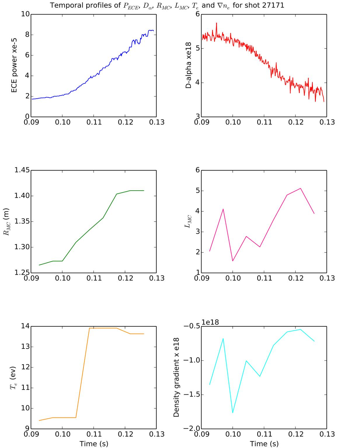
Figure A.1: Temporal profiles of ECE power (top left),  $D_\alpha$  emission (top right), radial location of MC window (middle left), density scale length (middle right), electron temperature at MC window (bottom left) and density gradient (bottom right) for shot 27171.
