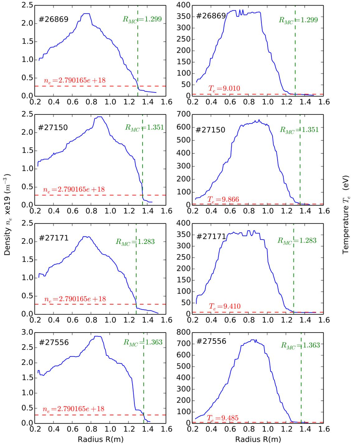
Figure 3.11: Radial density and temperature profiles for shots 26869, 27150, 27171 and 27566 for frequency channel six at  $t = t_0$ .
