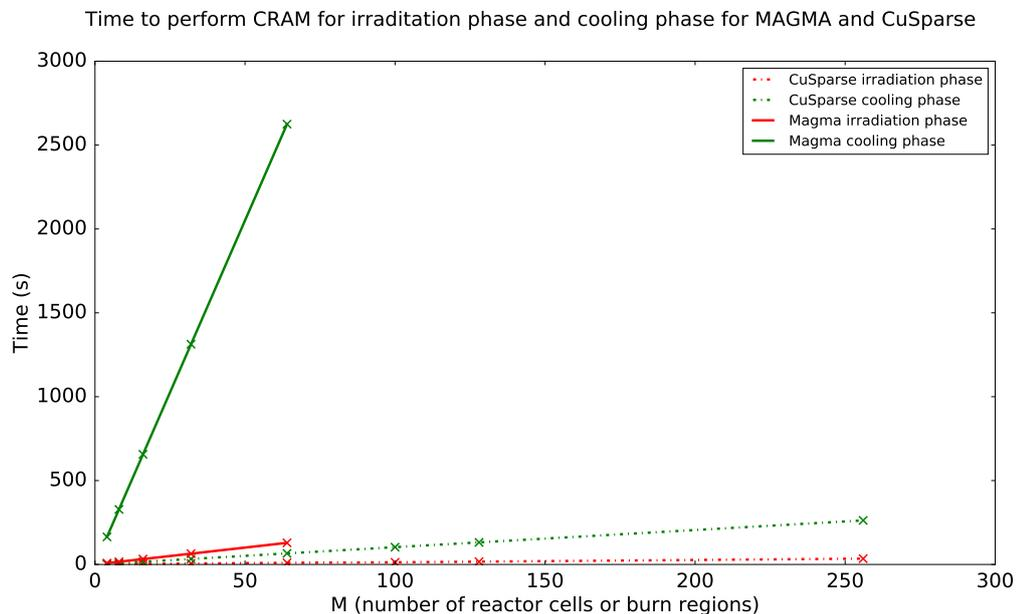
Figure 4.19: The run times for the irradiation and cooling phases of the CRAM solve for both MAGMA and CuSparse methods. The irradiation phase is quicker as this was just one time step in the FNS\_INCONEL simulation, whereas the cooling phase has 21 time steps to calculate.
