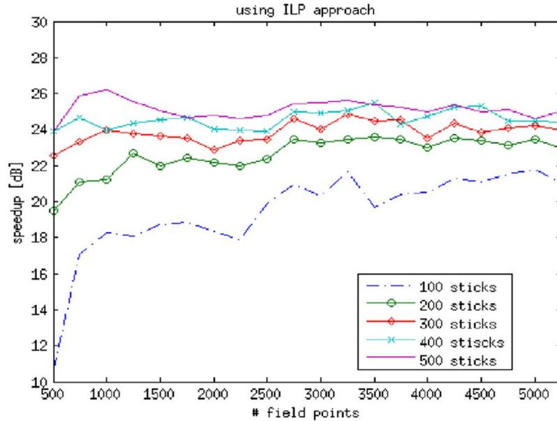
Figure 1.12: Speed-up of MISTIC code on a GPU compared to a CPU where  $\text{Speedup}_{dB} = 20 * \log_{10}(t_{CPU}/t_{GPU})$  [69]. The sticks discretize a conductor in an active coil, e.g. Central Solenoid coil.
