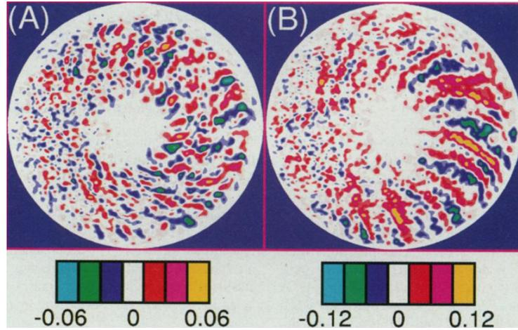
Figure 1.2: GTC poloidal contour plots of fluctuation potential ( $e\phi/T_i$ ) in the steady state of non-linear global simulation with  $E \times B$  flows included (A) and with the flows suppressed (B) [21].
