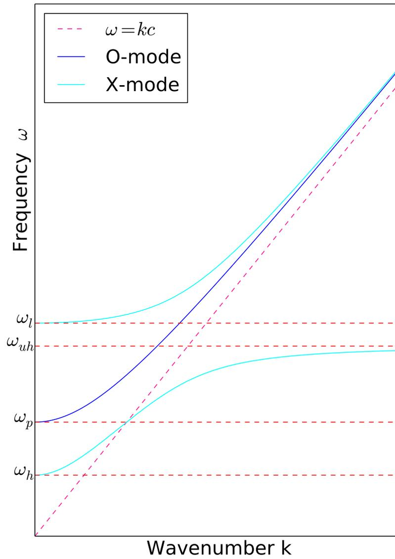
Figure 3.1: Dispersion relations for O and X modes indicating the cut-off frequencies  $\omega_l$ ,  $\omega_p$  and  $\omega_h$ , and the upper hybrid resonance  $\omega_{uh}$ .
