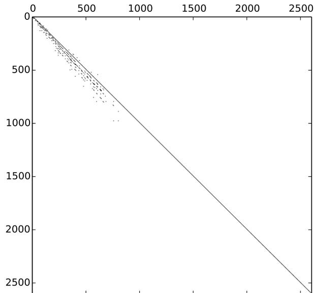
Figure 4.5: Activation matrix of size  $2604 \times 2604$  produced for one burn cell in the FNS\_INCONEL example showing the sparsity structure. There are 23856 non-zero entries in total.
