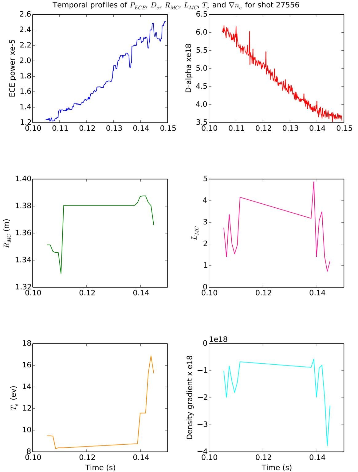
Figure A.2: Temporal profiles of ECE power,  $D_\alpha$  emission, radial location of MC window, density scale length, electron temperature at MC window and density gradient for shot 27556.
