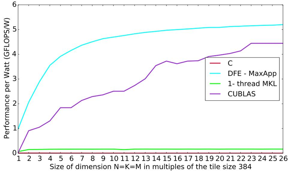
Figure 5.8: The performance per watt (GFLOPS/watt) for the serial C, DFE, CUBLAS and 1-thread MKL implementations for square matrix multiplication ranging from  $N = 384$  to  $N = 9984$ .
