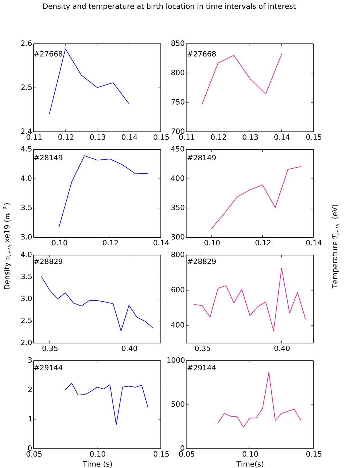
Figure 3.20: Temporal profiles of birth density (left) and birth temperature (right) of microwave emission for shots 27668, 28149, 28829, 29144.
