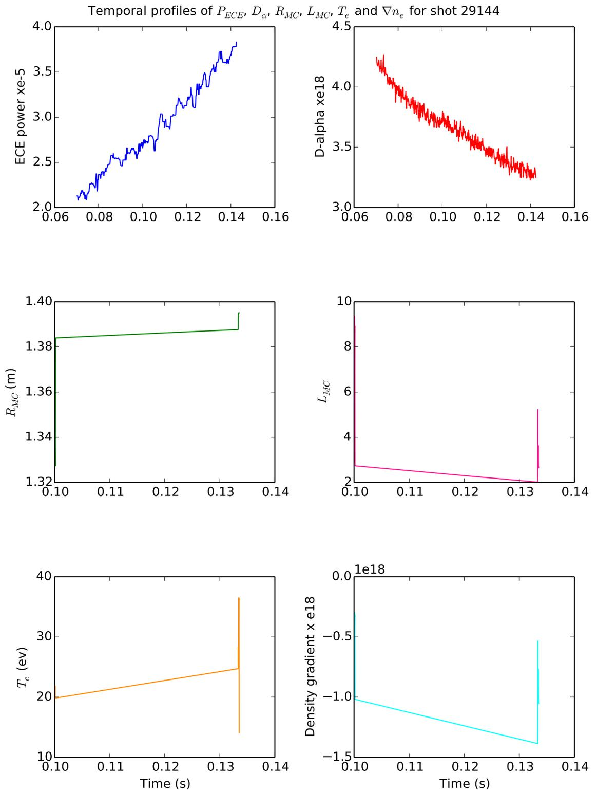
Figure A.6: Temporal profiles for shot 29144. All the previous shots show similar behaviour: the ECE increases, the  $D_\alpha$  decreases and  $T_e$  increases, as the plasma is moving out. Not much information can be obtained from  $L_{MC}$ , which depends on the density gradient.
