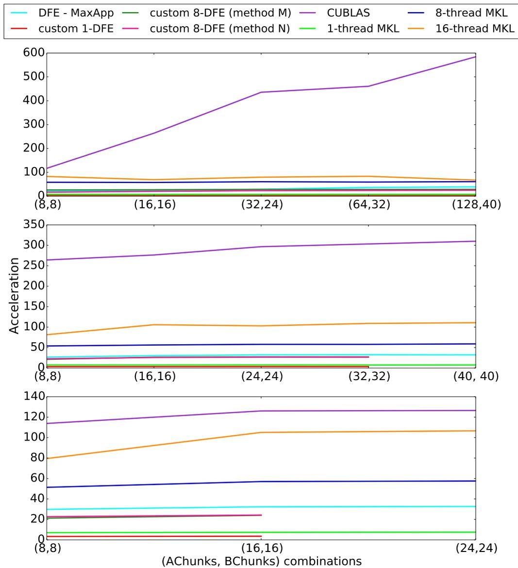
Figure 5.5: The acceleration over a serial C implementation of matrix-matrix multiplication, for increasing matrix sizes. The (AChunks, BChunks) combinations refer to the number of chunks the matrix A and matrix B are split into where the size of a single chunk of A is [40, 9320] (top), [300, 1242] (middle), [1000, 372] (bottom) and the size of a single chunk of B is [9320, 1440] (top), [1242, 1440] (middle) and [372, 1440] (bottom).
