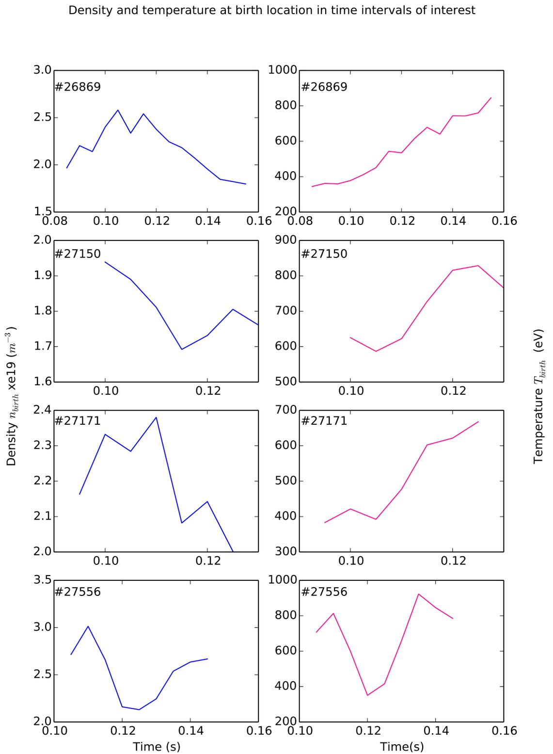
Figure 3.19: Temporal profiles of birth density (left) and birth temperature (right) of microwave emission for shots 26869, 27150, 27171 and 27566.
