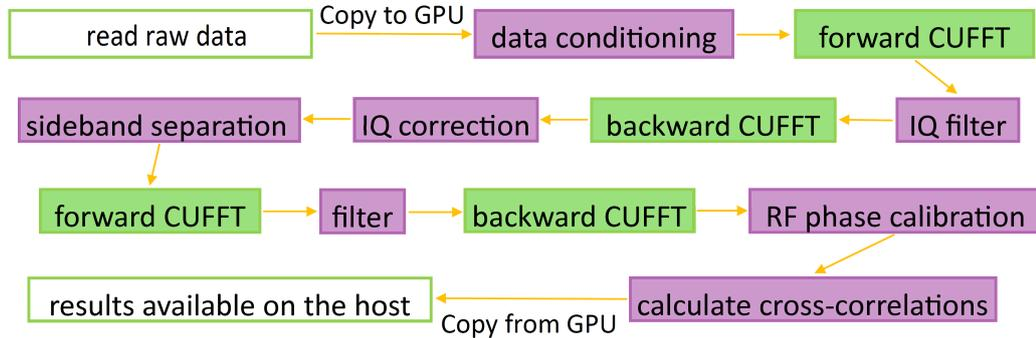
Figure 3.6: A schematic of the SAMI CUDA data processing code showing an initial data copy to the GPU, all data processing performed on the GPU and finally a resulting data copy back to the CPU.
