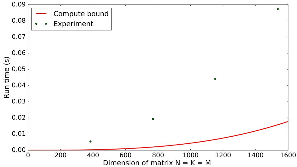
Figure 5.6: The curves for the experimental runtime and compute bound ( $4.34N^3$ ) runtime for square matrices,  $N=K=M$ . Matrix multiplication on the DFE is memory bound as the experimental runtime is slower than the compute time.
