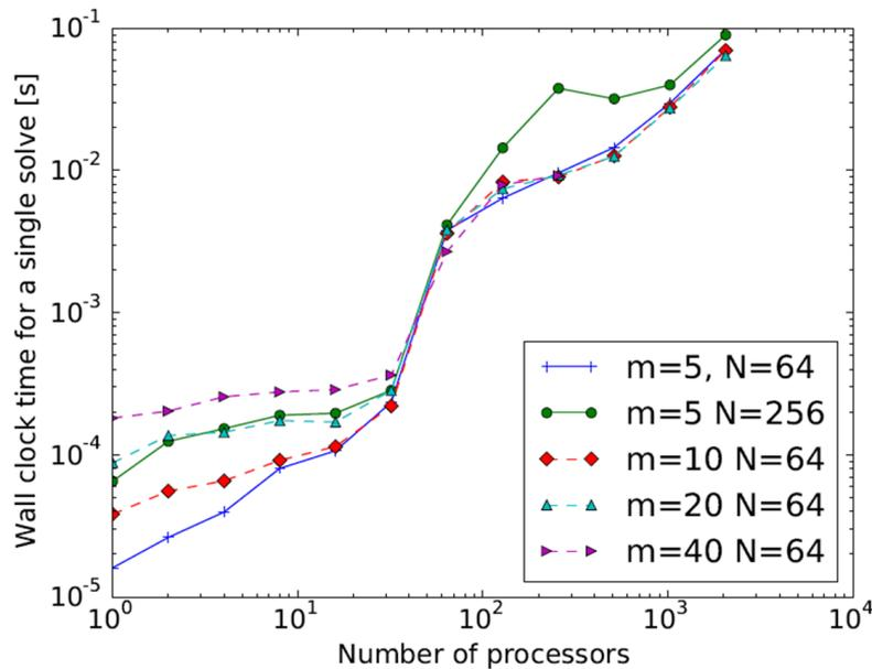
Figure 1.10: BOUT++ simulations on Hector with 32 cores per node and up to a maximum of 2048 cores.  $m$  is the size of each system, and  $N$  is the number of separate systems which are inverted simultaneously [38]. Past 32 cores, the inter-node communication dominates.
