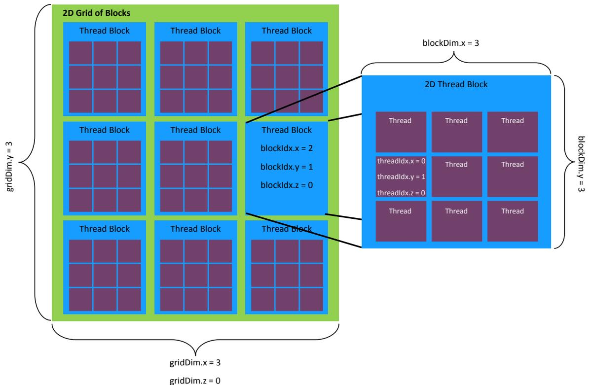
Figure 2.3: A grid used to launch a kernel, adapted from [85]. This is a 2D grid of blocks, where each block is a 2D block of threads. Each thread has a unique identifier labelled by the thread index within a block (specified by `threadIdx`) and the block index within the grid (specified by `blockIdx`).
