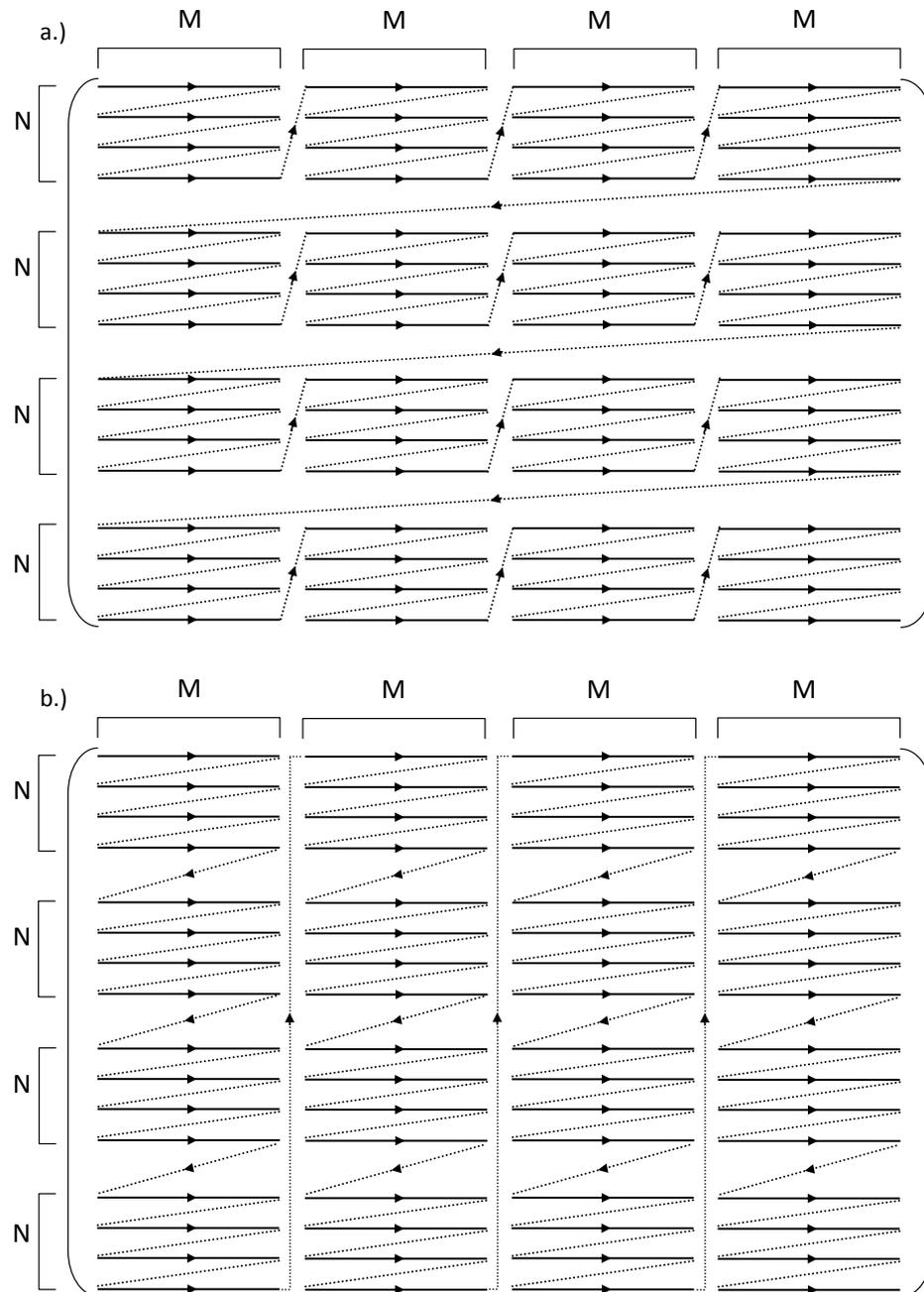
Figure 5.4: A schematic illustrating the order in which the elements of the resulting  $C$  matrix are computed for the two different DFE methods, (a)  $C$  computed row-wise, and (b)  $C$  computed column-wise. Solid lines represent contiguous data elements and dashed lines represent connections to the next contiguous data element.
