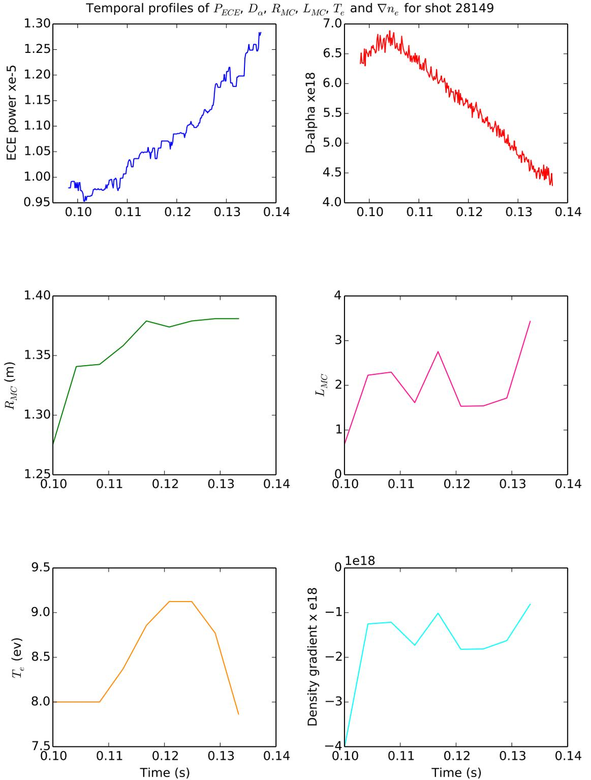
Figure A.4: Temporal profiles of ECE power,  $D_\alpha$  emission, radial location of MC window, density scale length, electron temperature at MC window and density gradient for shot 28149.
