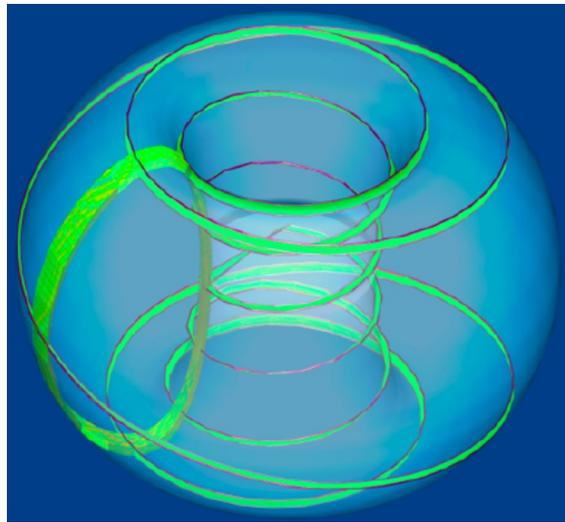
Figure 1.3: The green patches denote the reduced space time domain used in TRINITY, each of which corresponds to a nonlinear gyrokinetic flux tube simulation, and are the grid points in the coarse space-time mesh used to solve the transport equations [28].
