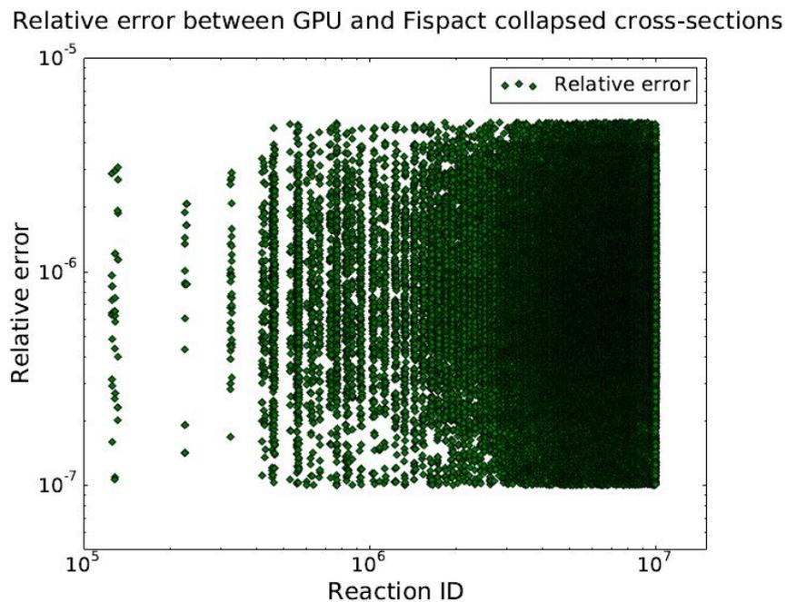
Figure 4.2: Relative error between FISPACT and GPU. Agreement is between  $10e^{-5}$  and  $10e^{-7}$ .
