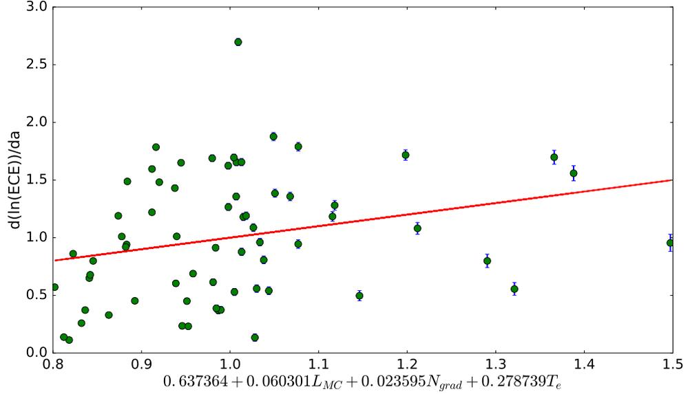
Figure 3.18: Multivariate linear regression for mode conversion parameters  $L_{MC}$ ,  $N_{grad}$  and  $T_e$ . Green points are the observed data, representing each shot. The red line is the model prediction. Error bars are based on the error associated with the Thomson scattering diagnostic.
