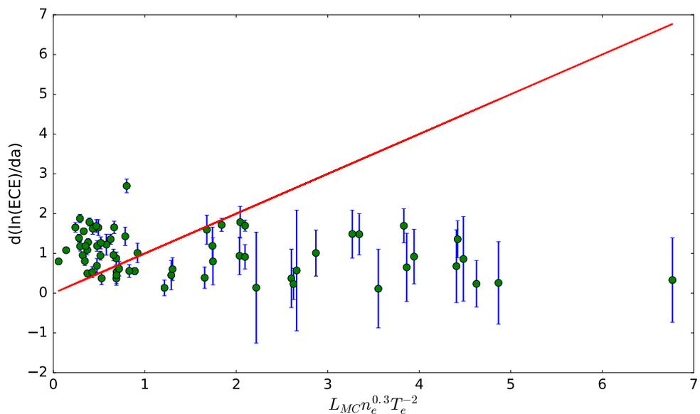
Figure 3.17: Model (iii). Green points are the observed data, representing each shot. The red line is the model prediction. Error bars are based on the error associated with the Thomson scattering diagnostic.
