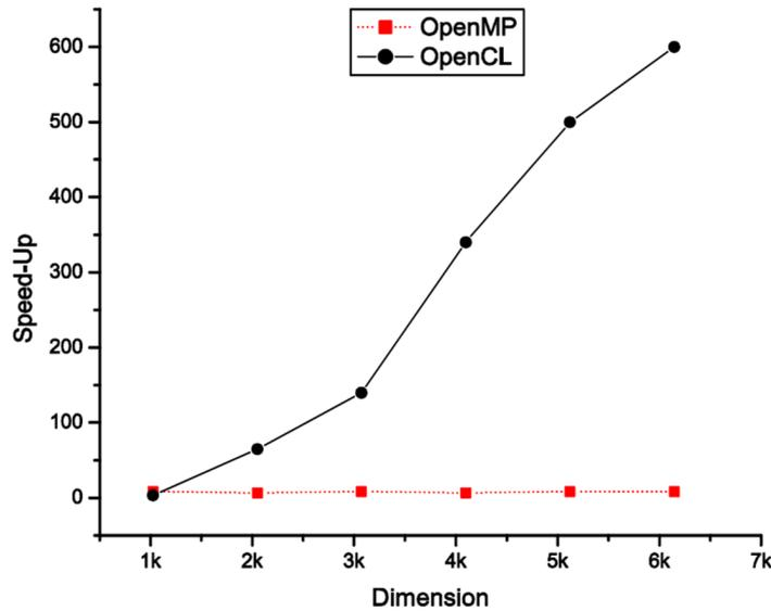
Figure 1.11: Speed-up comparison of dense matrix multiplication for an OpenMP and OpenCL GPU implementation compared to sequential implementation. The OpenCL implementation running on the GPU performs extremely well for large matrix dimension [51].
