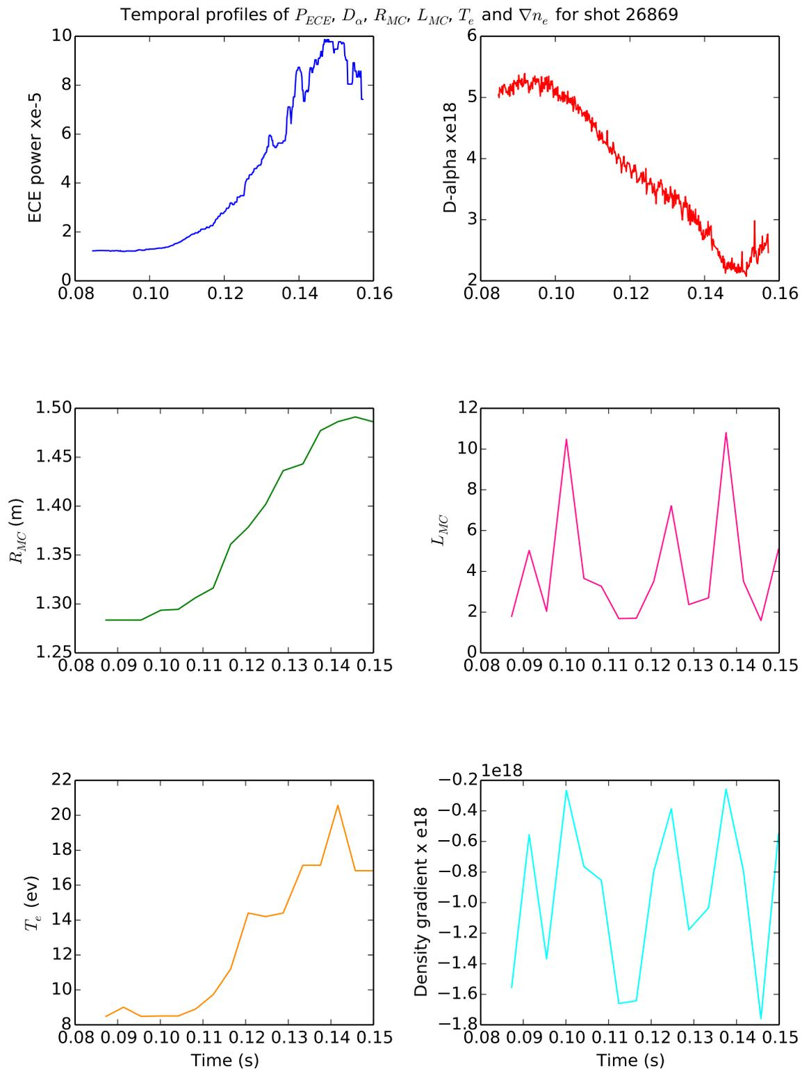
Figure 3.13: Temporal profiles of ECE power (top left),  $D_\alpha$  emission (top right), radial location of MC window (middle left), density scale length (middle right), electron temperature at MC window (bottom left) and density gradient (bottom right) for shot 26869.
