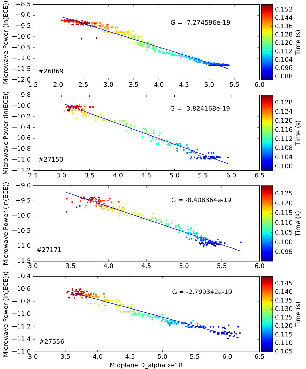
Figure 3.9: Plots of ECE power in antenna 0 vs.  $D_\alpha$  emission for shots 26869, 27150, 27171 and 27566 for frequency channel six (15 GHz). The gradient  $G$  is the exponent defined in equation 3.7.1.
