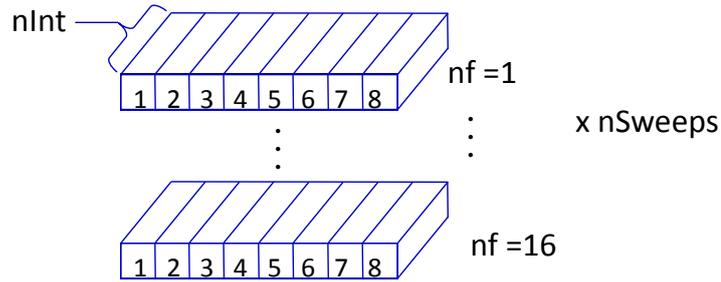
Figure 3.5: A schematic of the SAMI data structure highlighting the SIMD nature. The data is processed as a series of vector operations on vectors of size `nInt` where `nInt` is the number of data points collected before SAMI switches to the next frequency channel.
