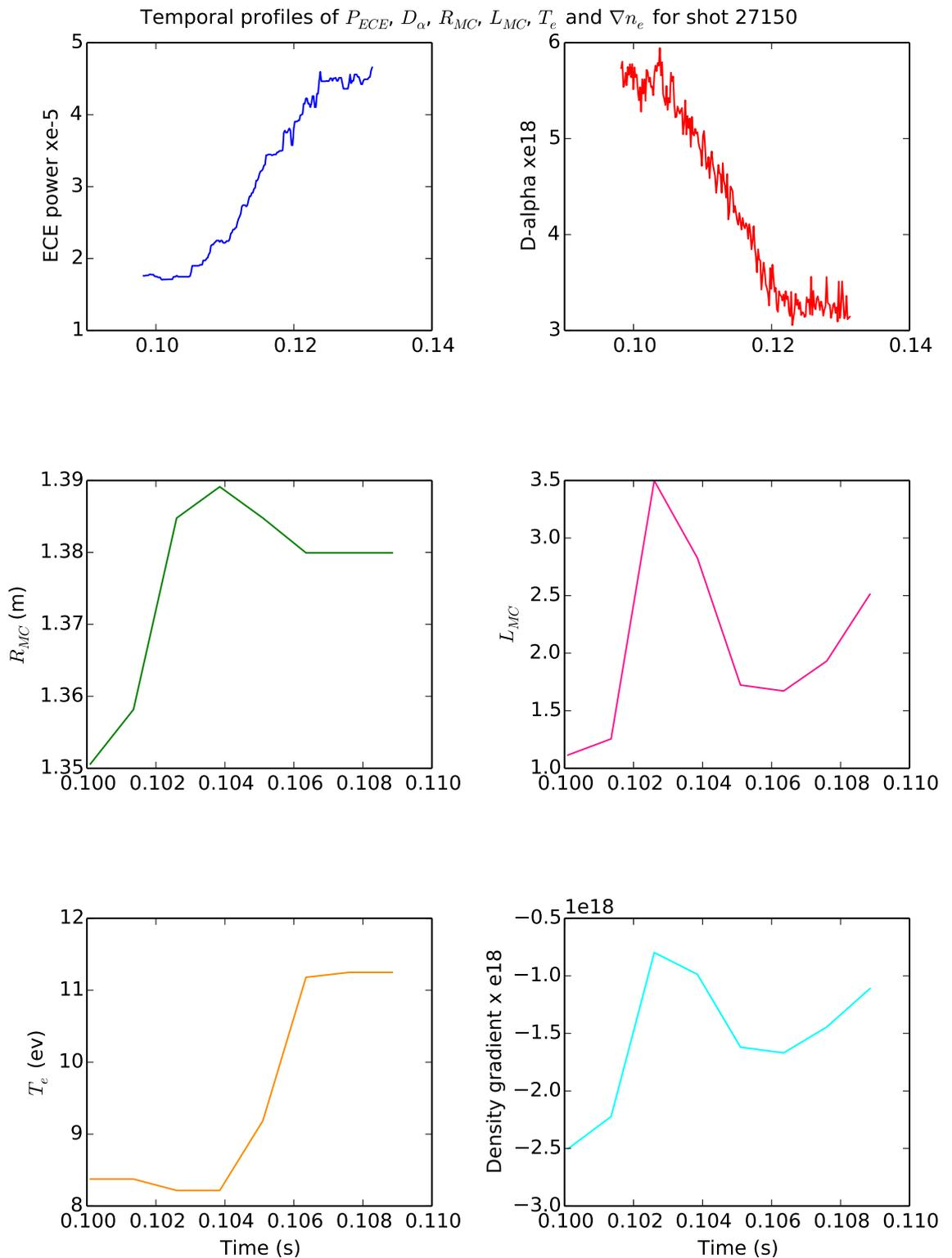
Figure 3.14: Temporal profiles of ECE power,  $D_\alpha$  emission, radial location of MC window, density scale length, electron temperature at MC window and density gradient for shot 27150.
