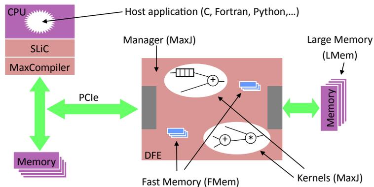
Figure 2.6: A diagram of the DFE system showing detail of the LMem (large off-chip memory), FMem (small on-chip memory), kernel and manager [95]. The DFE is connected to the CPU via PCIe.
