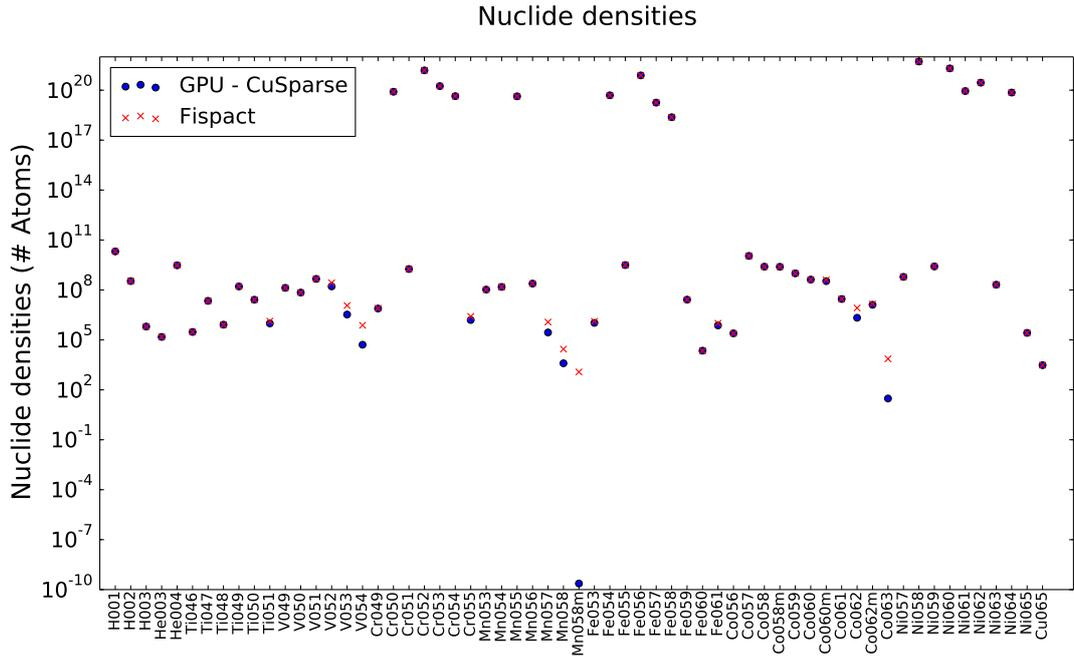
Figure 4.13: FISPACT and GPU inventories using CuSparse to solve the system of linear equations show good agreement for some nuclides but poor agreement for others.
