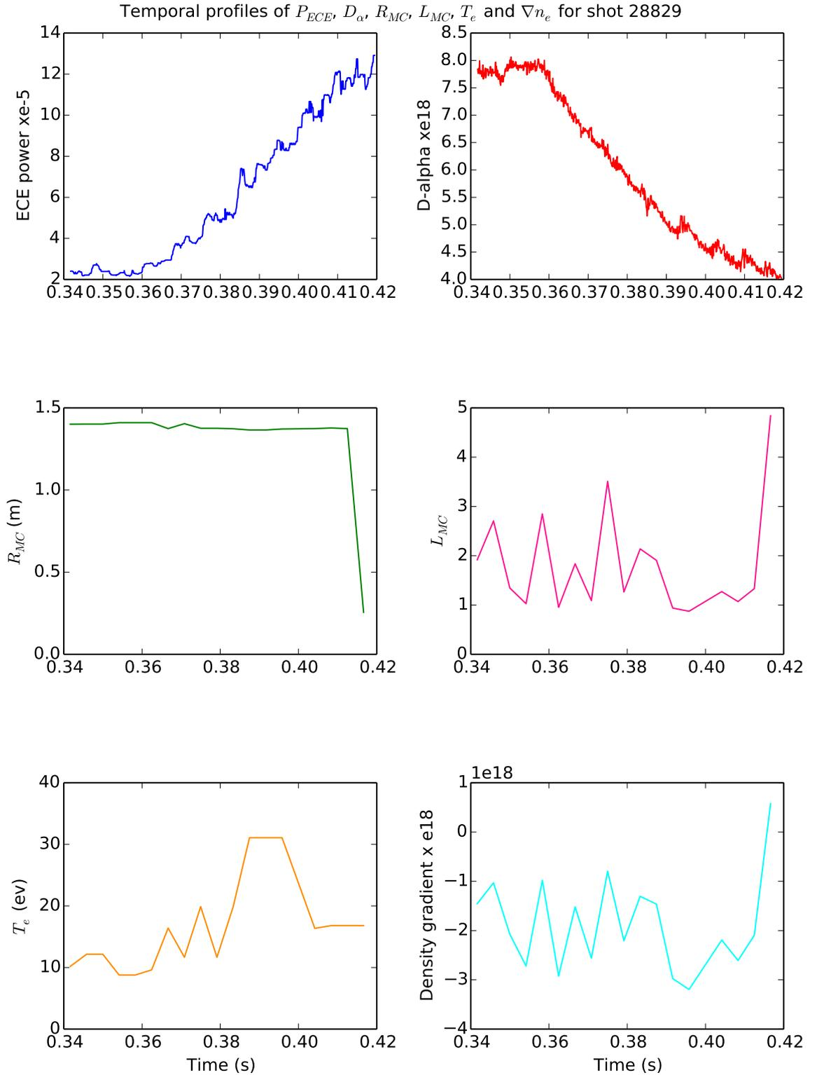
Figure A.5: Temporal profiles of ECE power,  $D_\alpha$  emission, radial location of MC window, density scale length, electron temperature at MC window and density gradient for shot 28829.
