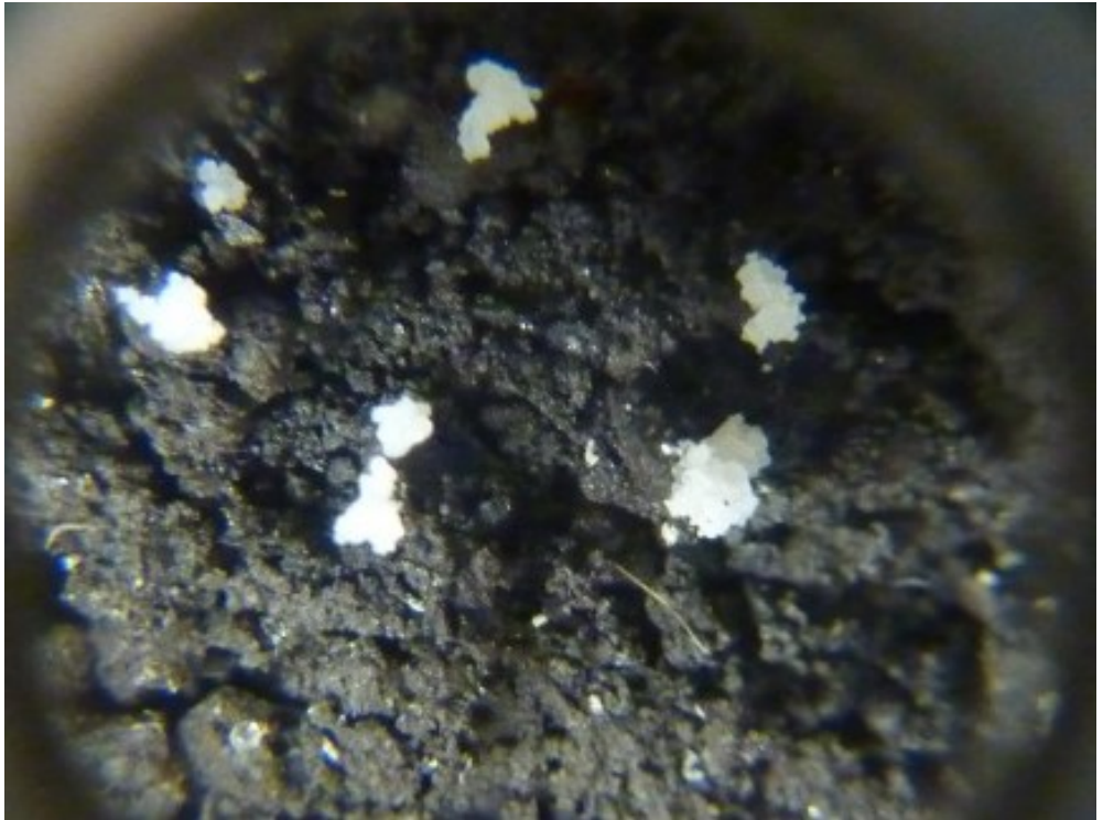
Figure 6.7: Ca-rich crystals precipitated from the CO 2 -Slag-H 2 O fluid at the base of Pipe-2.
