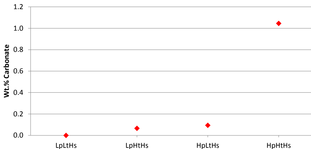
Figure 7.10: Graph showing the carbonation values achieved for 6 mm aggregate slag treated with 1M HCl under the active reaction conditions.
