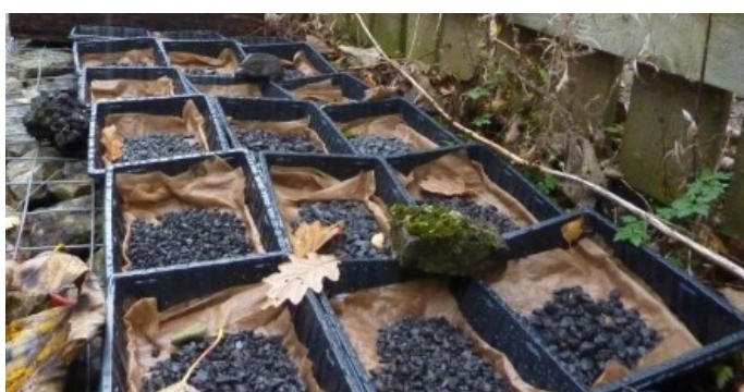
Figure 4.1: Samples weathering in trays under environmental conditions.
