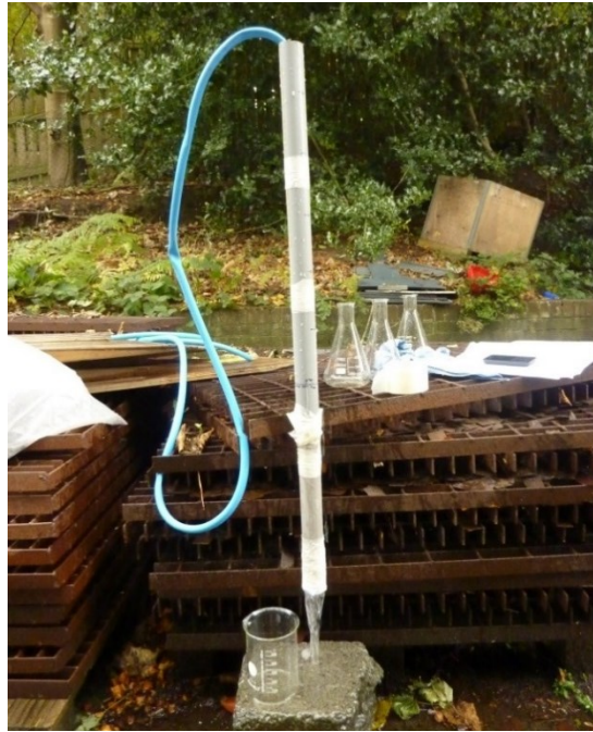
Figure 2.5: Simple apparatus for determining vertical permeability.
