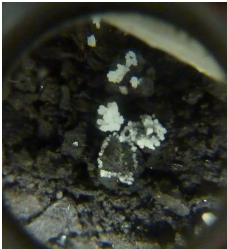
Figure 6.8: Ca-rich crystals precipitated from the CO 2 -Slag-H 2 O fluid at the base of Pipe-2.
