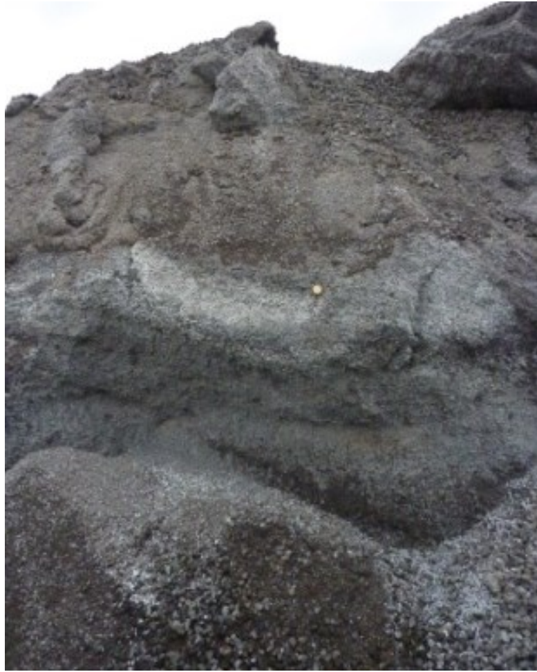
Figure 4.16: Photo of weathering within a sectioned 6 mm aggregate slag heap. Weathered layer is approximately 2.66 % of the heap volume. (Heap height approximately 2 m – gold disk is £1 coin)
