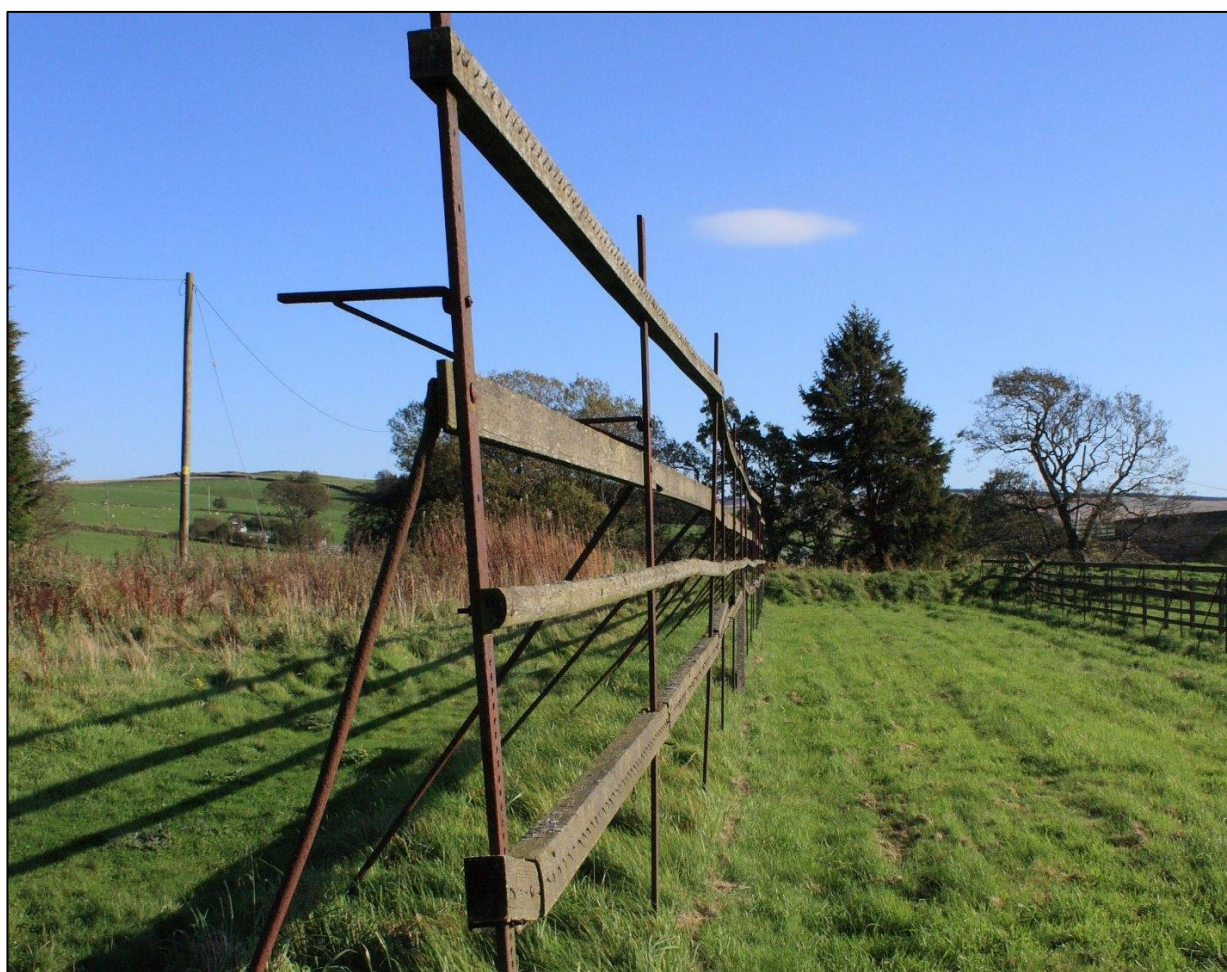
Fig 6.19. Surviving eighteenth-century tenter frames, Otterburn Mill, Northumberland. Image re-produced with kind permission from Janet E. Davis.
