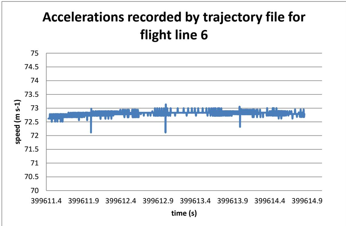
Figure 5-67 graph showing speed over time (acceleration) for flight 6. The spikes in acceleration shown at the whole second are an artefact of the trajectory software rather than true acceleration
