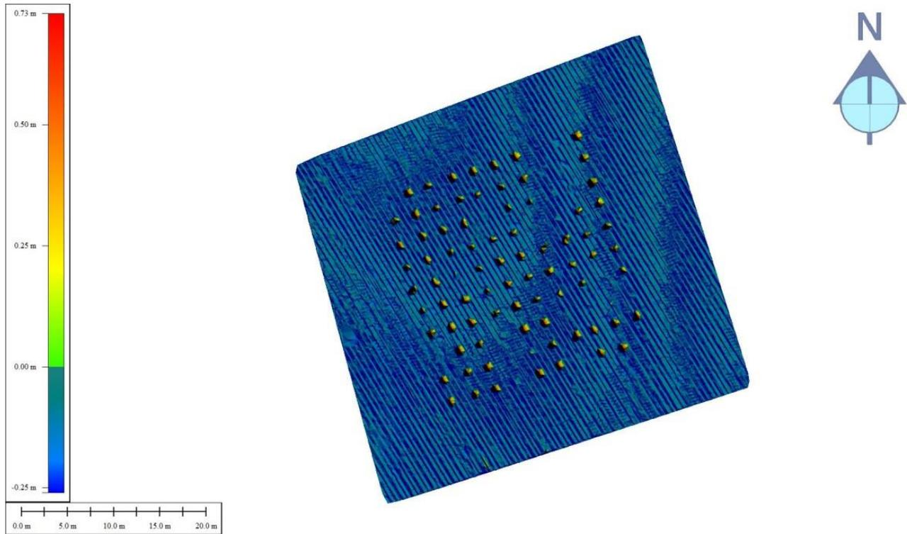
**Figure 5-25 flight 7 normalised DSM. Table separation is 1.5 metres.**
