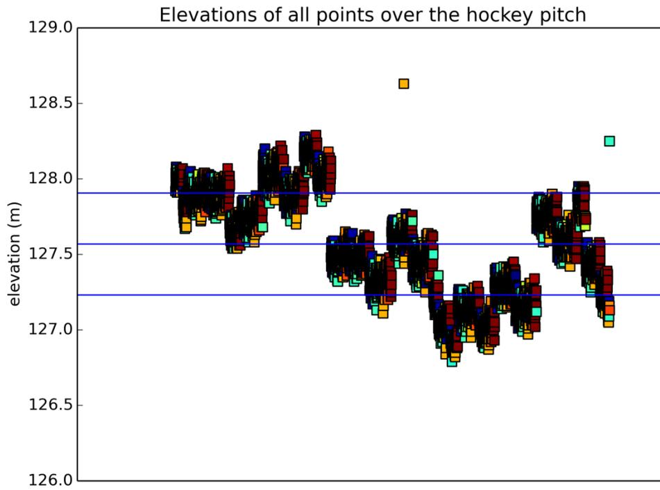
**Figure 5-70 elevation of each point on the hockey pitch. Coloured by flightline. The 3 horizontal bars represent the mean and 1 sigma confidence limits.**
