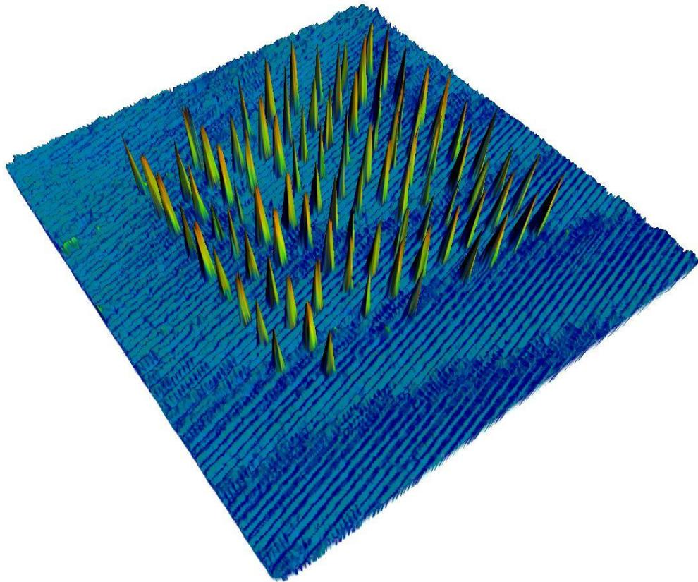
**Figure 5-24 shows a 3 dimensional view of flight line 5's normalised DSM, this highlights the difference between the observations. Table separation is 1.5 metres.**
