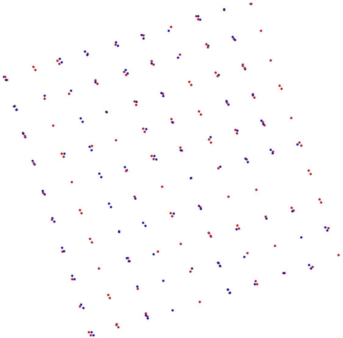
**Figure 5-10 showing the tables detected for the 2.5-metre configuration. No other LiDAR returns are shown in this image. The LiDAR returns are coloured by flight line.**
