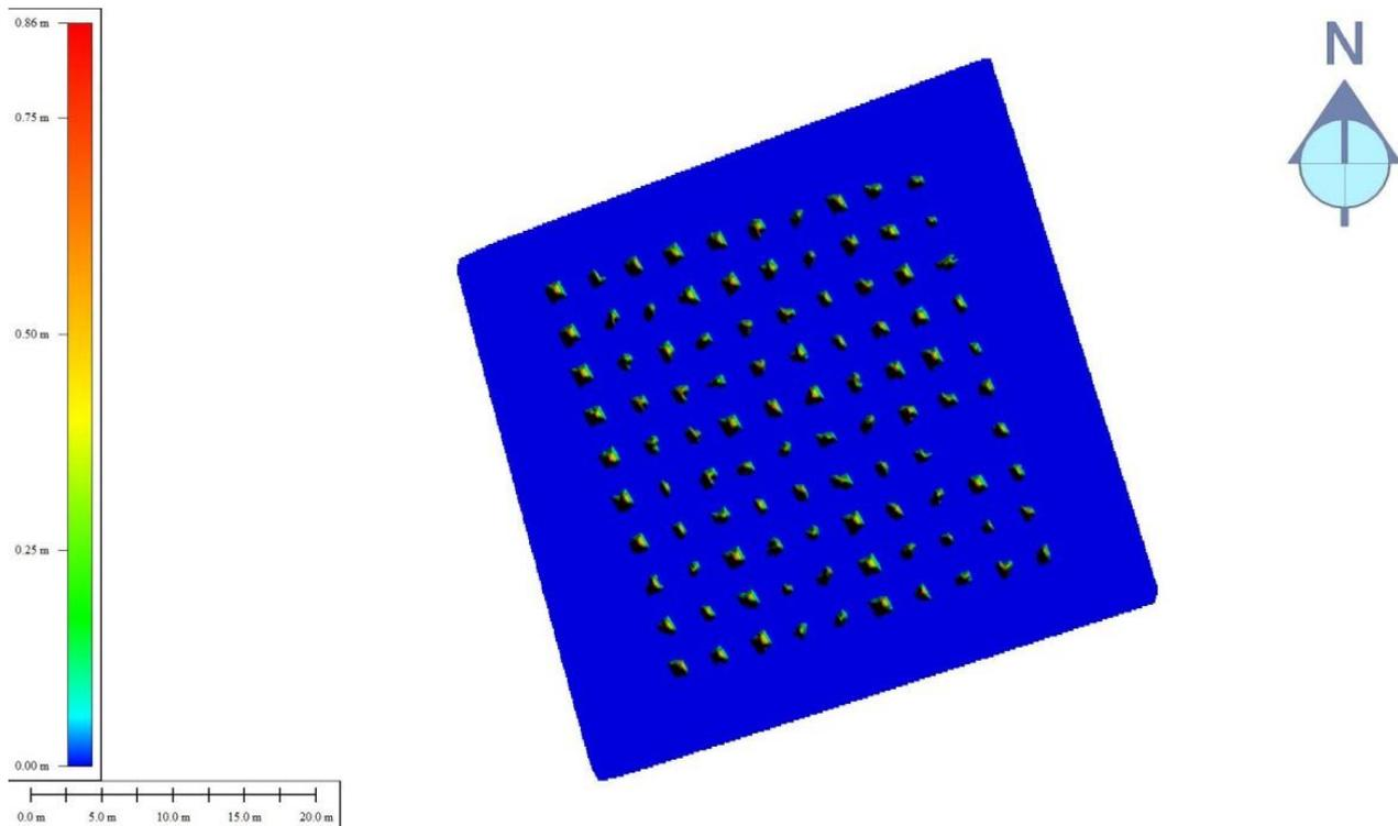
**Figure 5-15 Shaded surface model showing the table surface produced by two over flights of the 2.5 metre configuration, ground level removed to express elevations above local ground height.**
