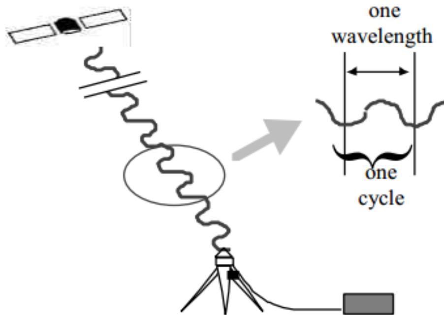
**Figure 3-11 Showing the carrier phase signal to be calculated. source Trimble 2007.**
