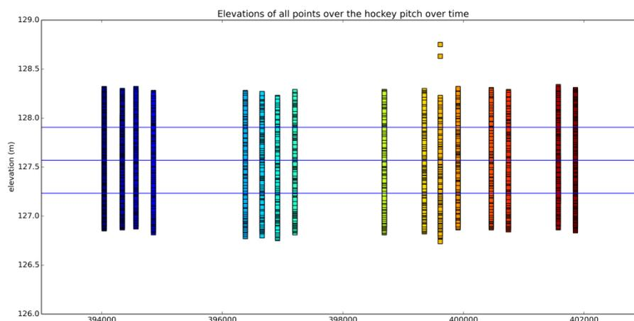
**Figure 5-71 shows a scatter plot of elevation against GPS time. Each vertical cluster is a flight line and the spread of elevations shows the variation.**
