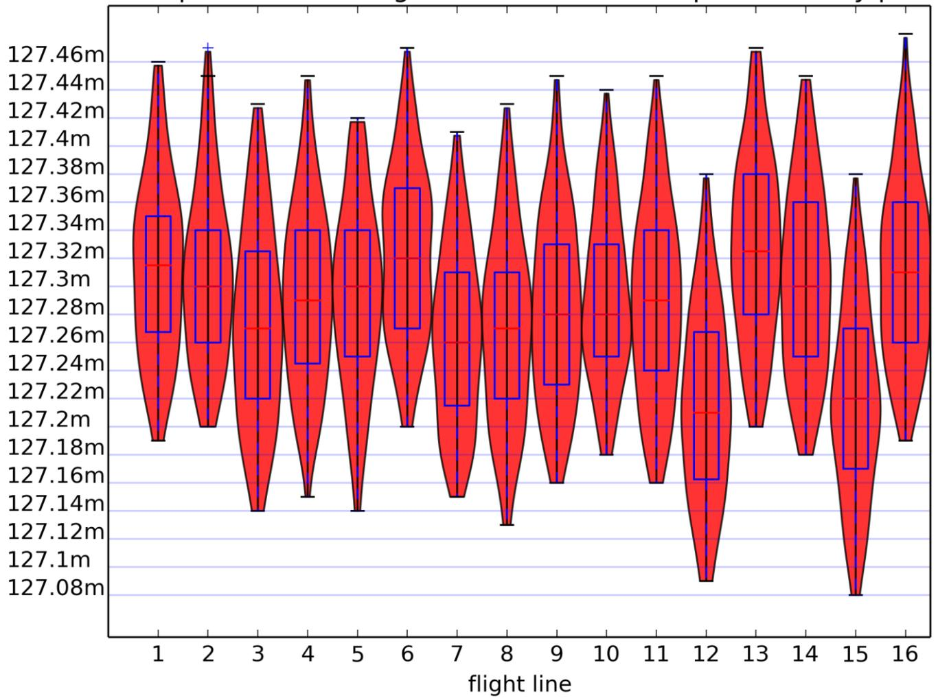
Figure 5-72 Violin plot showing a 5 metre sample of LiDAR data.
