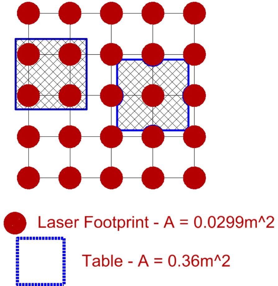
Figure 5-2 showing the different illumination an object can achieve for the same scan pattern
