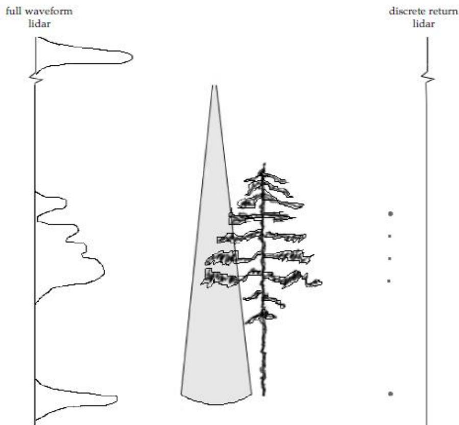
**Figure 3-10** showing the difference in pulse recording between Full waveform (left) and discrete return (right) taken from Lim *et al.*, (2003) page 92
