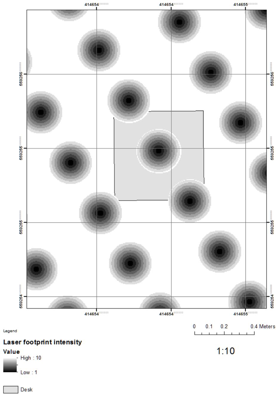
Figure 5-3 Map showing the laser footprints coloured by intensity and a mock up table placed within the survey area
