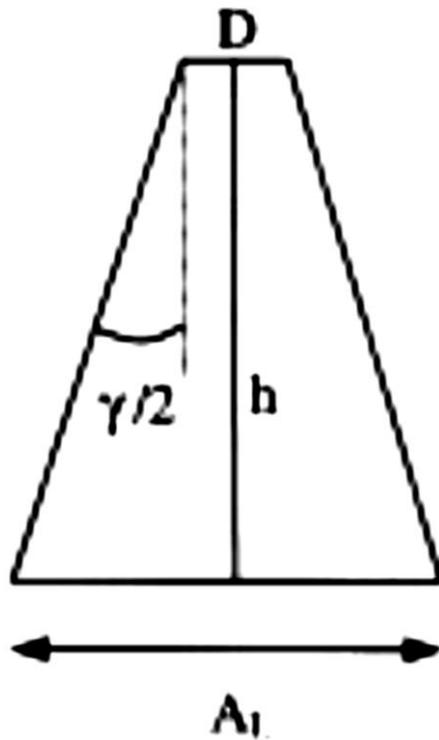
Figure 3-6 Diagram showing the effect of aperture (D), beam divergence (γ) and height (h). When the incident surface is flat. Source Baltasvias, 1999.
