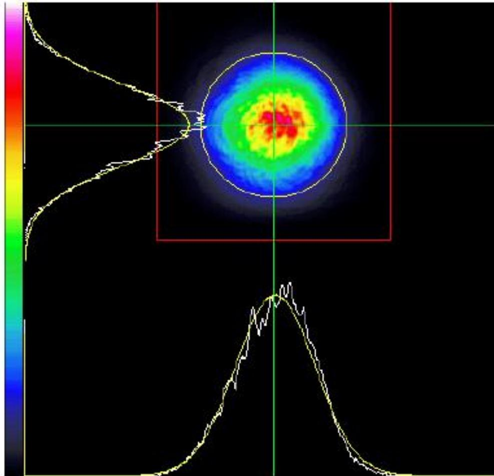
Figure 3-7 showing the Van Mises distribution seen within a laser footprint. Source Ussyshkin (2009)
