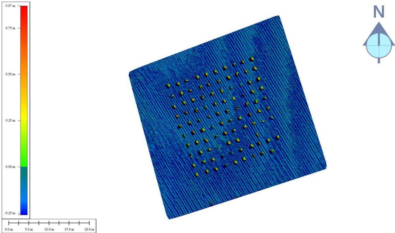
**Figure 5-27** both flights shown as a normalised DSM. Table separation is 1.5 metres.
