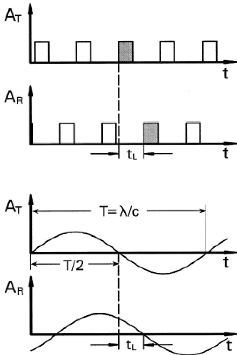
Figure 3-5 Diagram showing the difference between the time of flight method (top) and phase difference method (bottom) of determining an objects distance from the scanner. Source Wehr and Lohr, (1999) page 71
