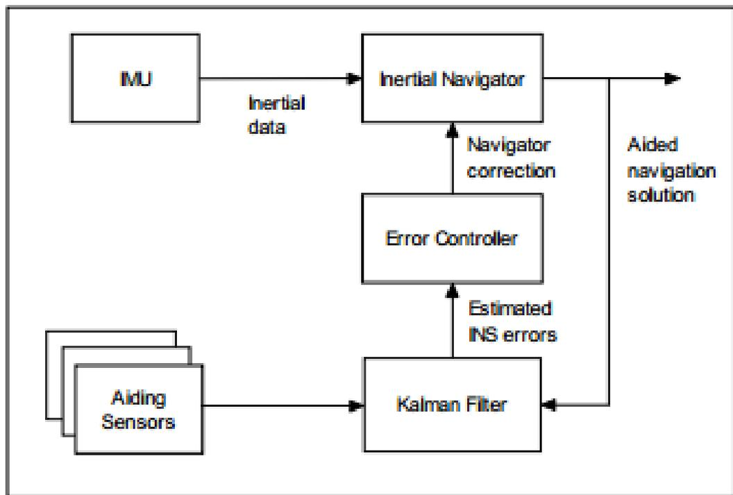
**Figure 3-13 showing the generic architecture of a loosely coupled filter. Source Scherzinger and Hutton 2006**
