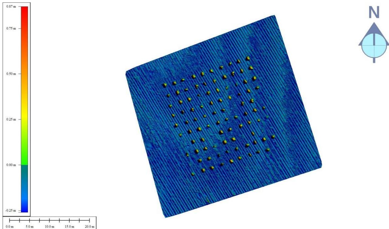
**Figure 5-23 shows the normalised DSM for flight 5. Table separation is 1.5 metres.**
