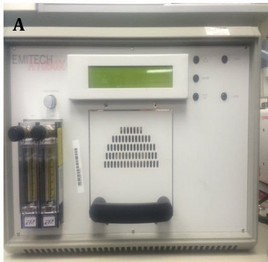
Figure 2.2 A Plasma Asher can be used to pre-treat Alvetex® scaffolds
