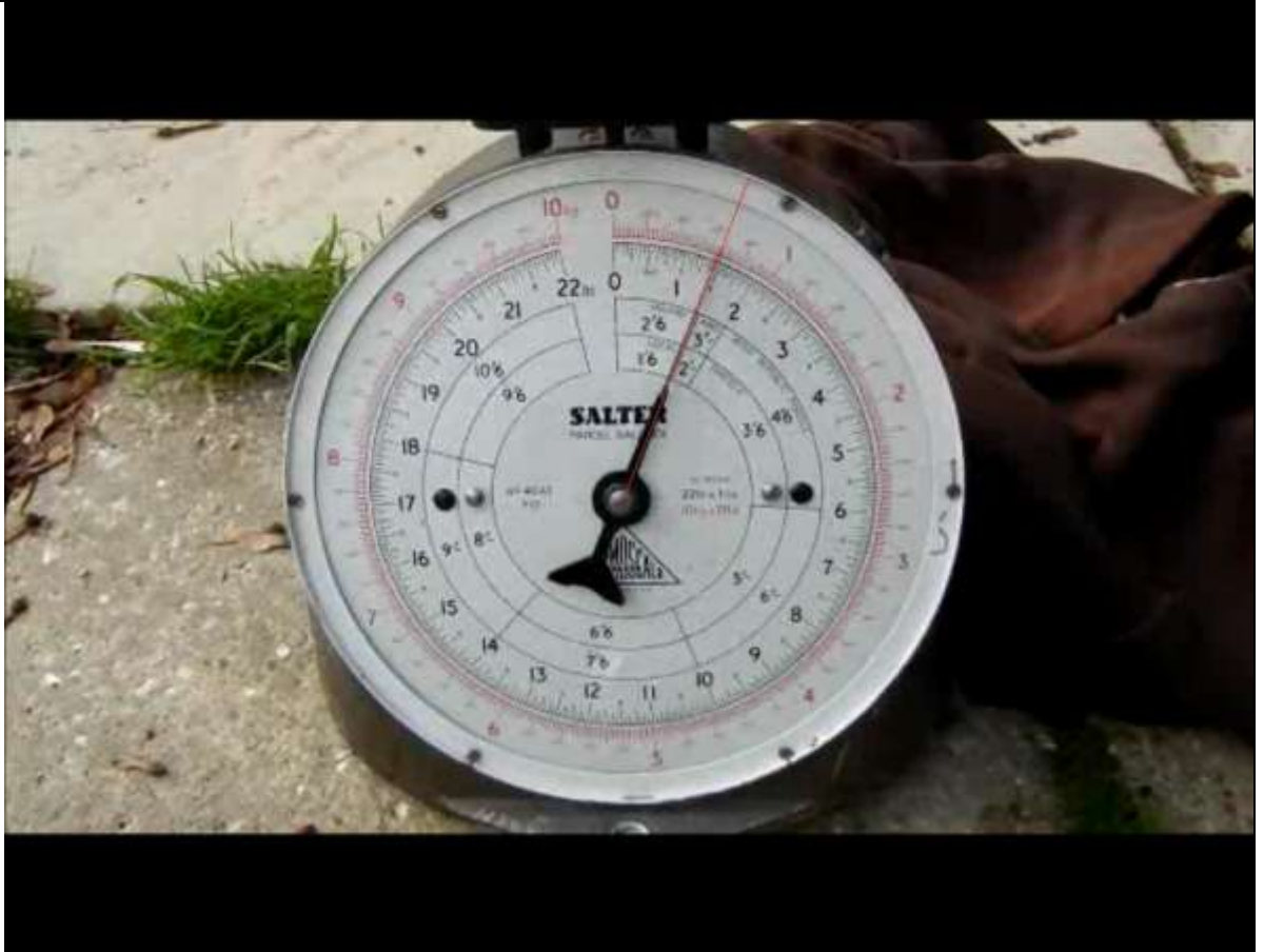
Figure 9.6: Example of an edited screenshot with a red line added to provide a visual aid for taking readings from the dial of the top-loading scale.
