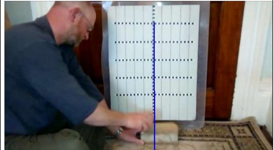
Figure 9.12: Examples of edited screenshots from the footage obtained from Subject 11. The coloured lines were added to provide a visual aid for taking readings from the vertical and horizontal scales during the data extraction stage. The height of the hammerstone blow (i.e., the distance between the two red lines) can be determined from the image showing the maximum height of the hammerstone and the position of the striking platform (left). Note that though the red line at the bottom is not lined up with the scale, the scale can be extended in the editing process to allow readings to take place (see Figure 9.13 below). The degree of lateral movement of the hammerstone blow can be established by comparing the degree of movement from the outside edge of the hammerstone in its starting position (blue line in the image on the left) with the point of its maximum horizontal movement (blue line in the image on the right).
