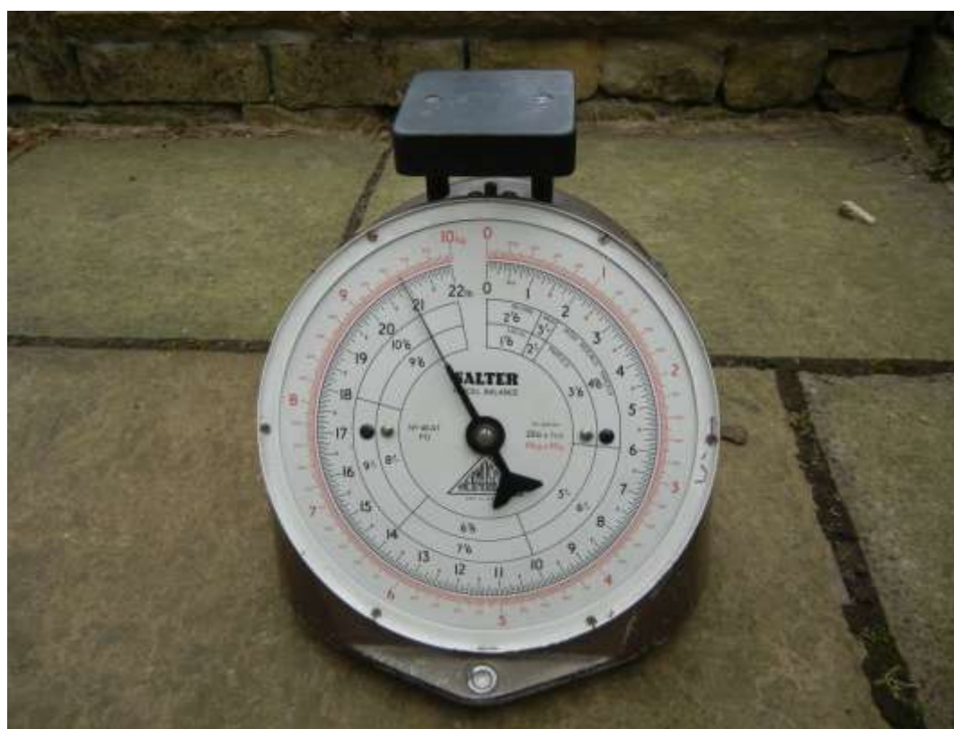
Figure 9.1: The Salter top-loading, dial scale parcel balance used to record blow strengths. Test participants were asked to strike the hard rubber striking platform with the hammerstone in Figure 9.3.
