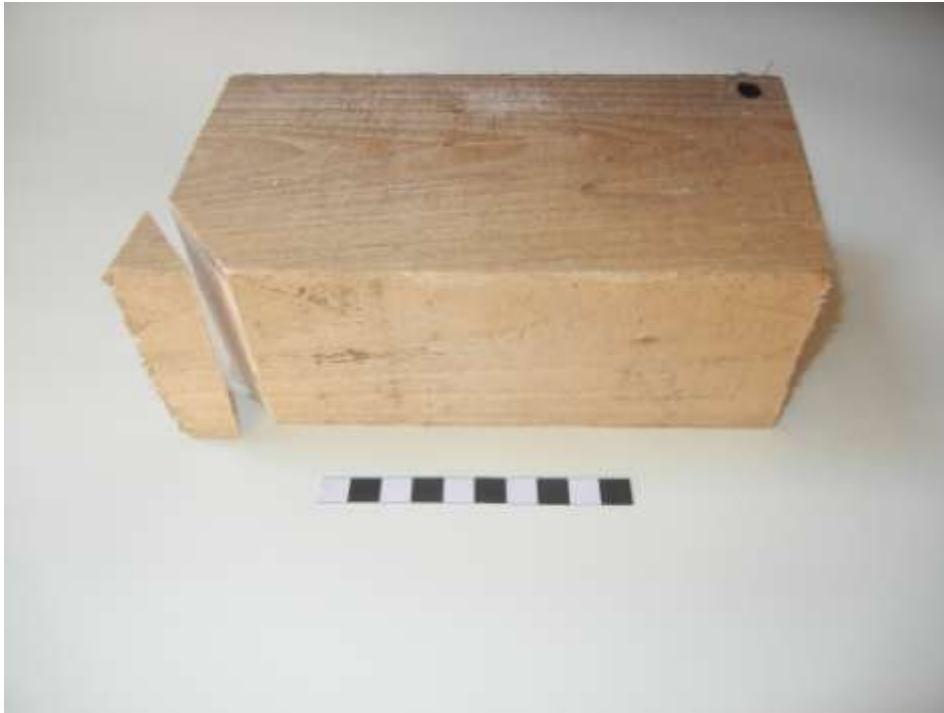
Figure 9.7: The wooden substitute core (19.4cm x 9.8cm x 7.4cm) used by participants in the second phase. An example flake was removed prior to testing (bottom left) and test participants were asked to apply blows to remove a similar flake on the adjacent corner (top right, with a black dot indicating the approximate striking point) (scale in cm).
