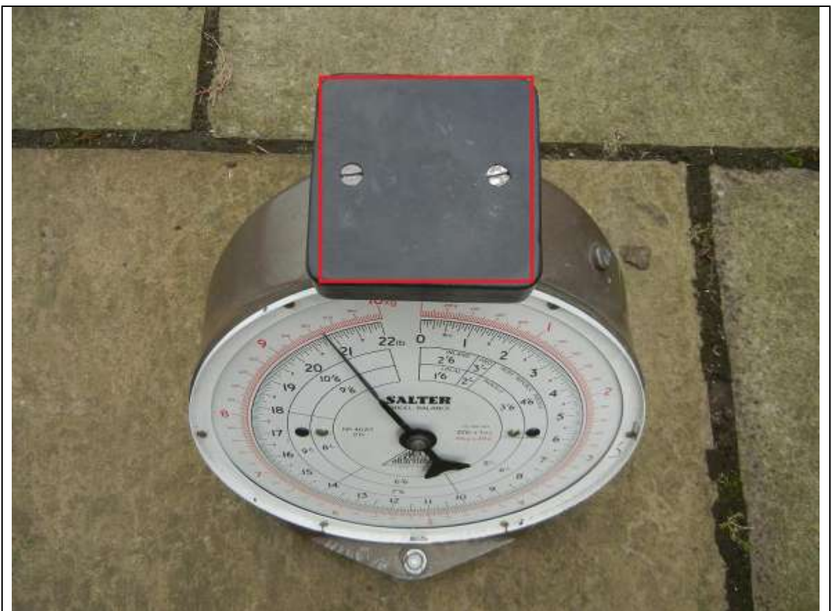
Figure 9.2: Top view of the striking platform. The silversmiths rubber block (highlighted in red) provided a striking platform for test participants (Length 10.0cm, Width 10.0cm, Depth 2.5cm, Weight 365g).
