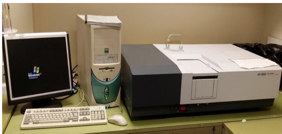
Figure 3.3 Shimadzu UV/VIS/NIR spectrometer in Durham university OEM research laboratory
